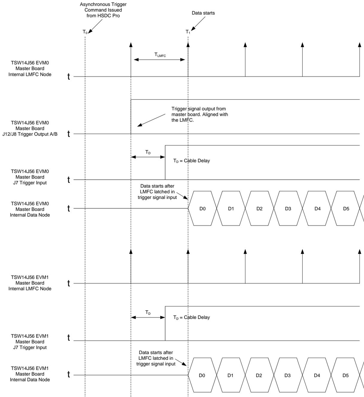
Figure 12. TSW14J56 EVM Sample Alignment in Trigger Mode
