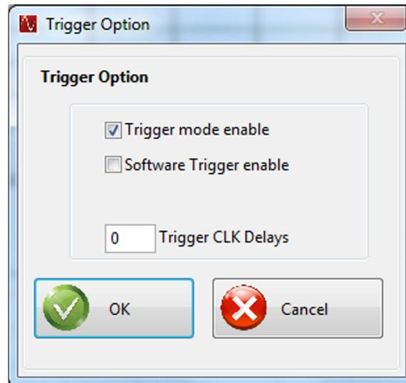
Figure 23. Enabling Slave Mode for TSW14J56 EVM1
