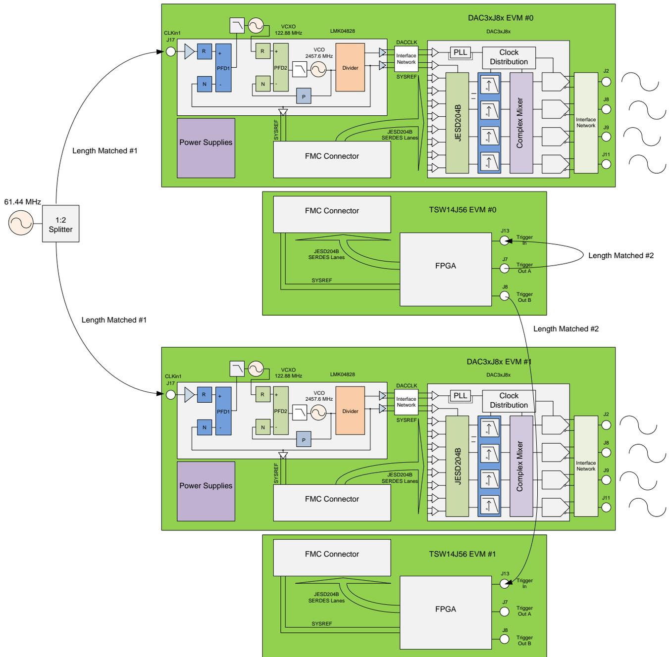
Figure 3. Overall Measurement Setup to Achieve Multiple DAC3xJ8x Device Synchronization
