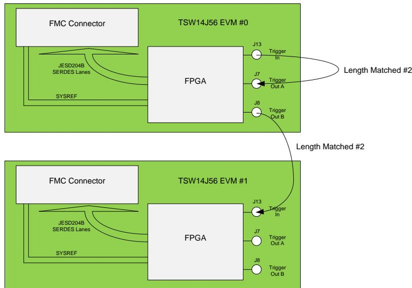
**Figure 11. TSW14J56 EVM Master and Slave Trigger Setup**
