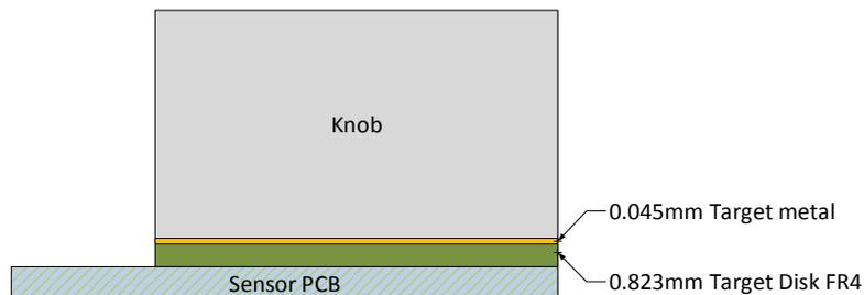
**Figure 24: Target Disk – Sensor spacing using target disk PCB**
