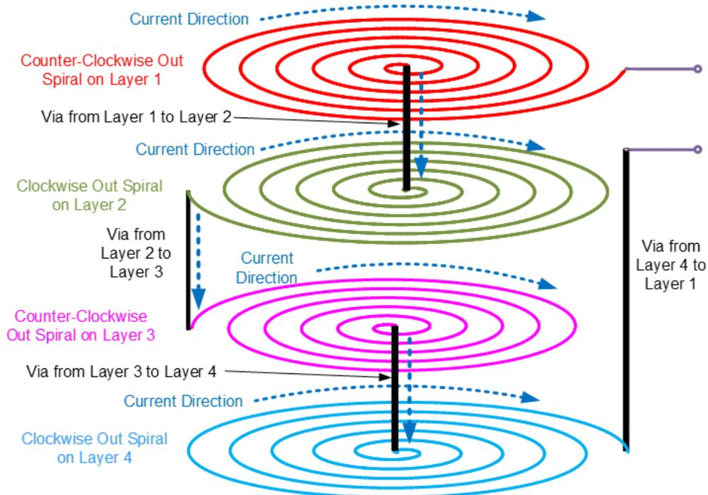
**Figure 22: 4-Layer Inductor/sensor physical construction**
