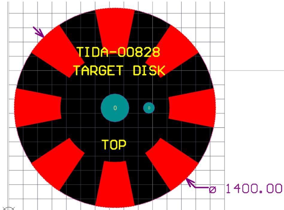
Figure 43: Target Disk PCB Top layer and Top Silkscreen
