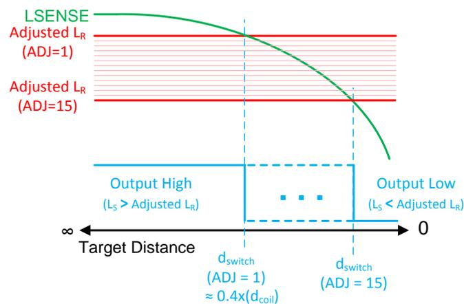
**Figure 12: LDC0851 ADJ pin functionality**
