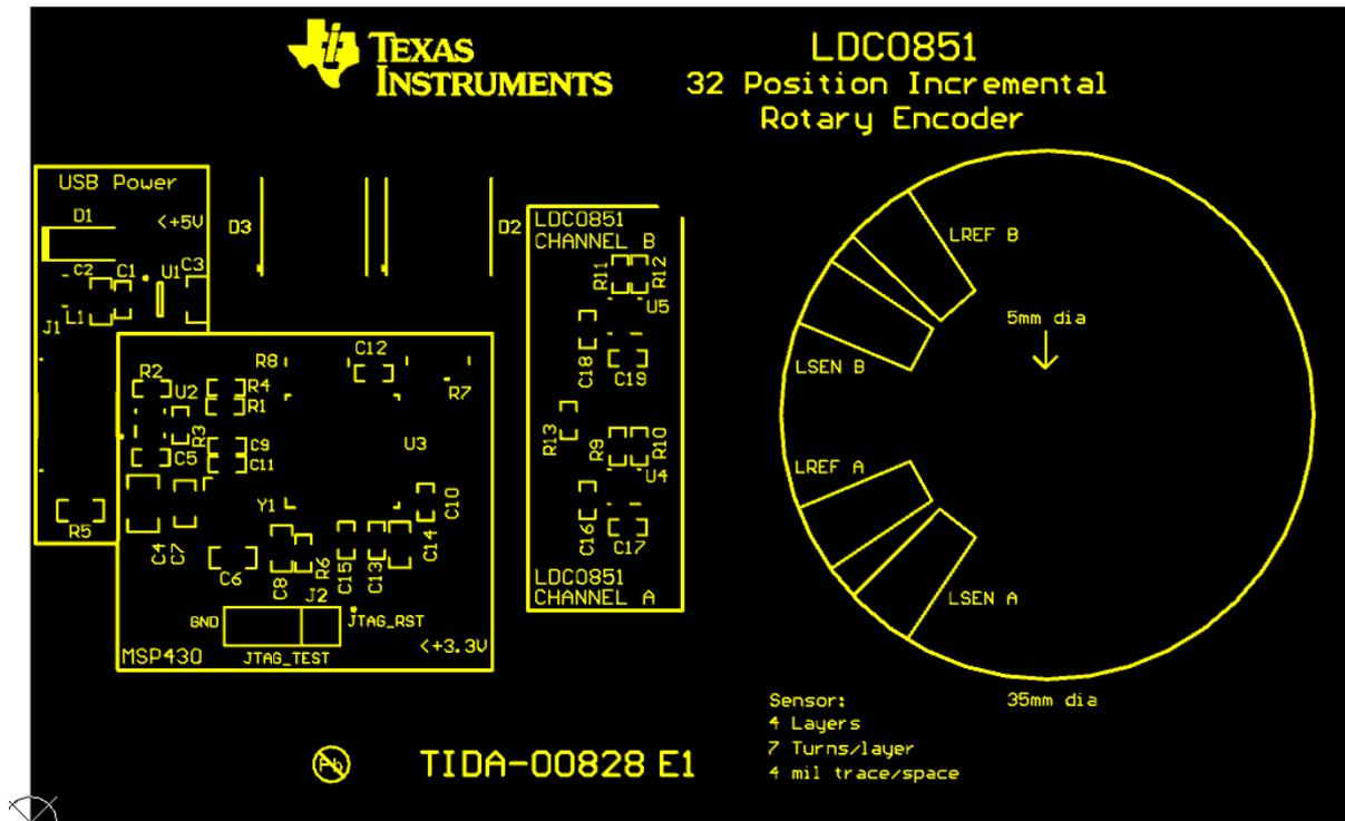
Figure 35: Sensor PCB Top Silkscreen
