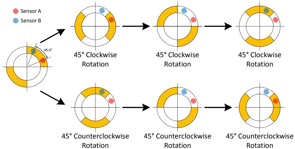
**Figure 15: 8-Position target disk and sensor (SENSE coils) configuration**
