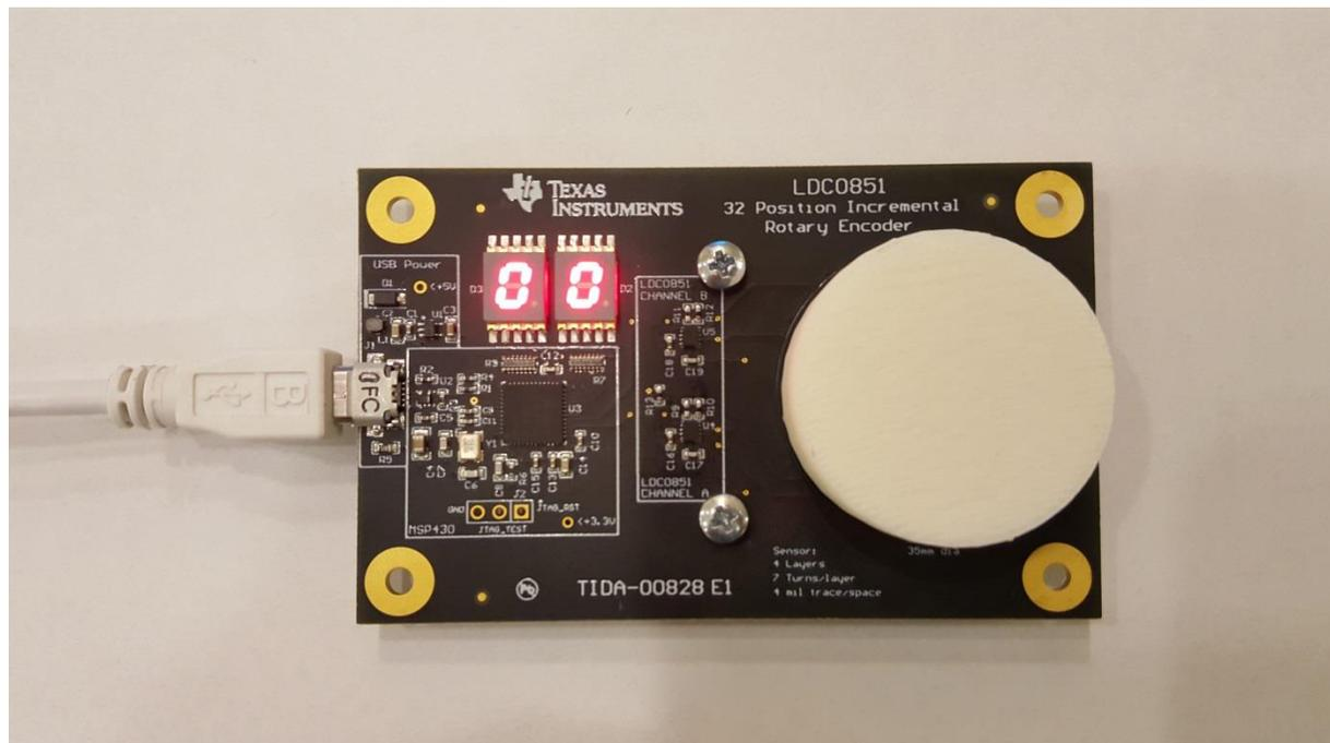
**Figure 3: TIDA-00828 powered up by USB Connection**
