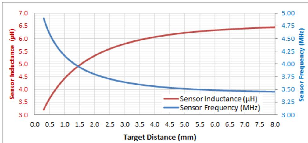
**Figure 7: Example Sensor Response vs. Target Distance**
