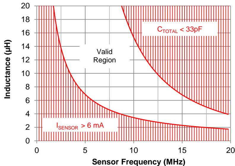
Figure 19: Inductance vs Sensor Frequency Design Space for 3.3V supply
