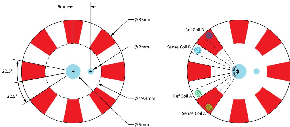
**Figure 18: (Left) 32-Position target disk geometry, (Right) Sensor placement**
