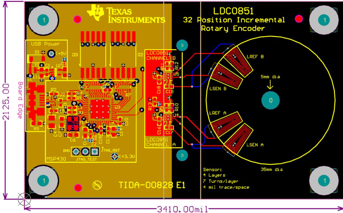
Figure 34: Sensor PCB Multi-layer
