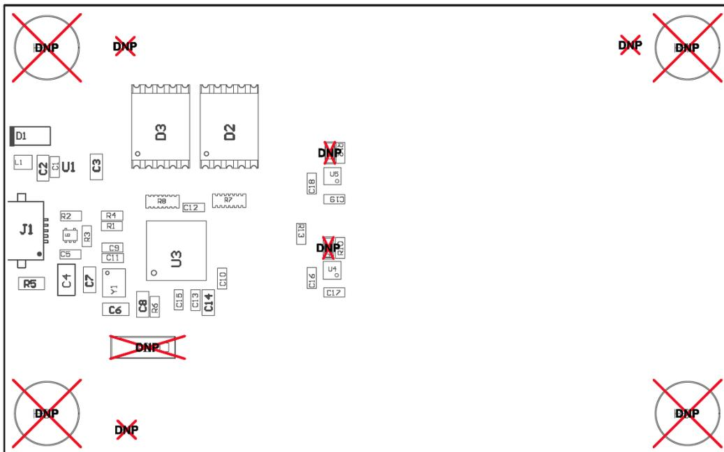
Figure 46: Sensor PCB Assembly Drawing
