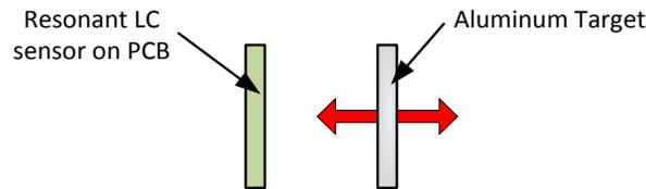
**Figure 6: Aluminum Target moved axially with respect to LC resonant circuit**
