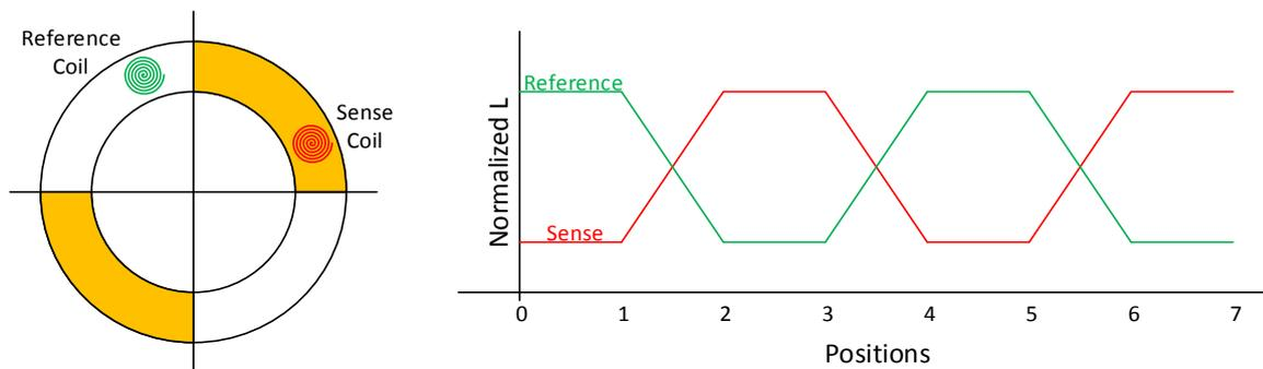
**Figure 17: Reference coil placement and inductance shifts**
