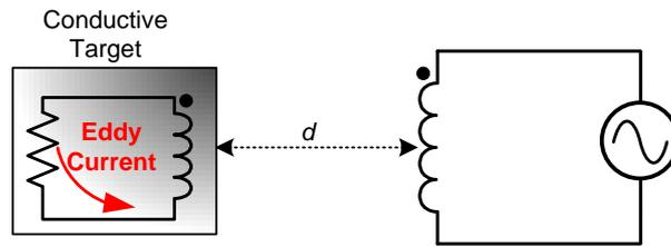
**Figure 4: Conductor in AC Magnetic Field**
