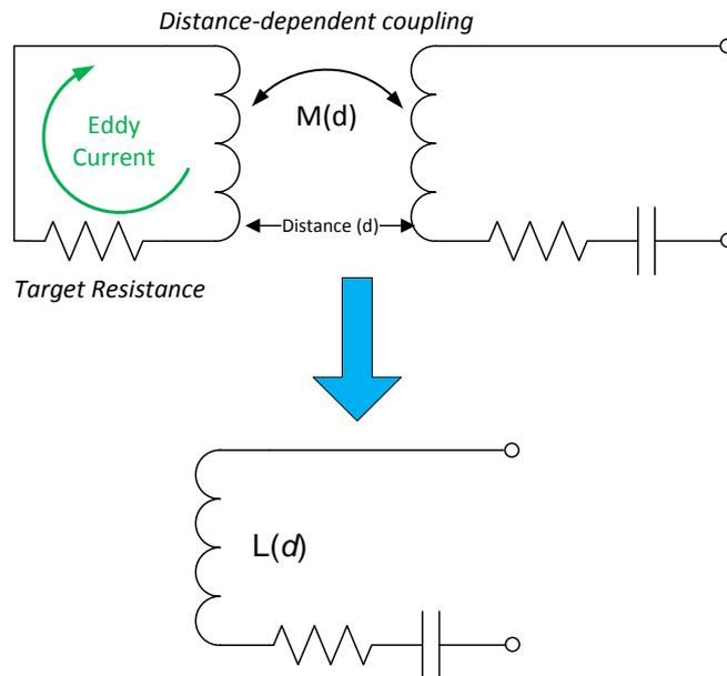
**Figure 5: Electrical Model of Series Inductive Sensor**
