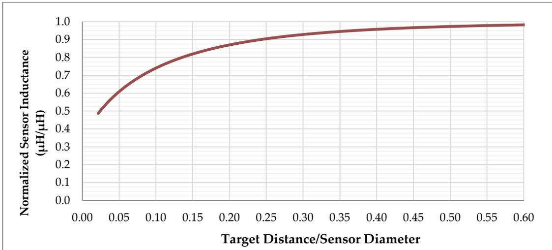
**Figure 8: Normalized Sensor Response**
