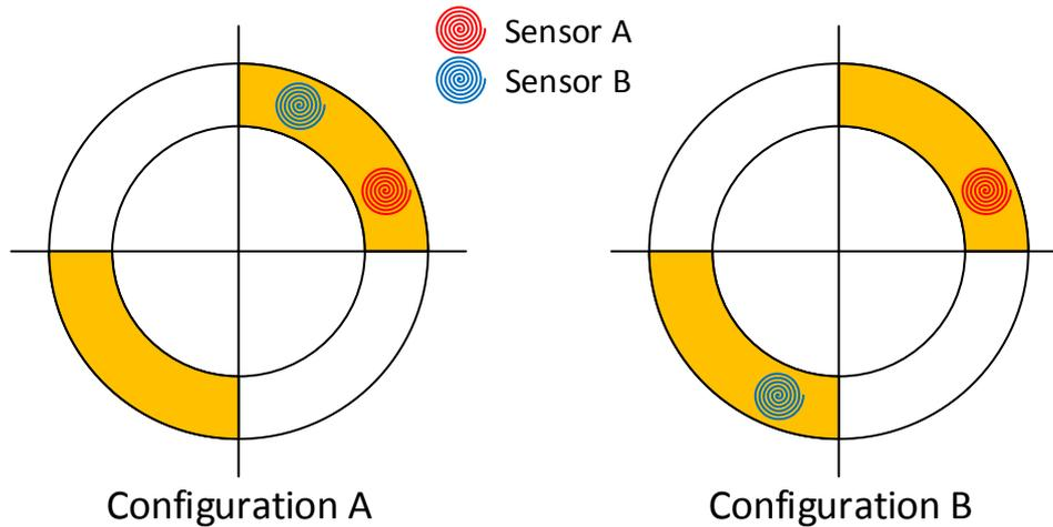
**Figure 16: Equivalent configurations for sense inductors**
