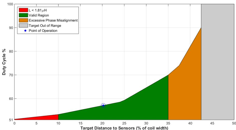
**Figure 28: Target disk distance from sensors vs output duty cycles**
