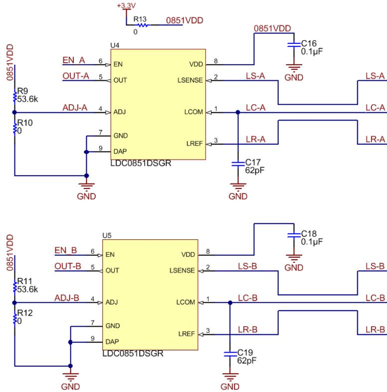
Figure 30: LDC0851 and Sensors. Channels A and B
