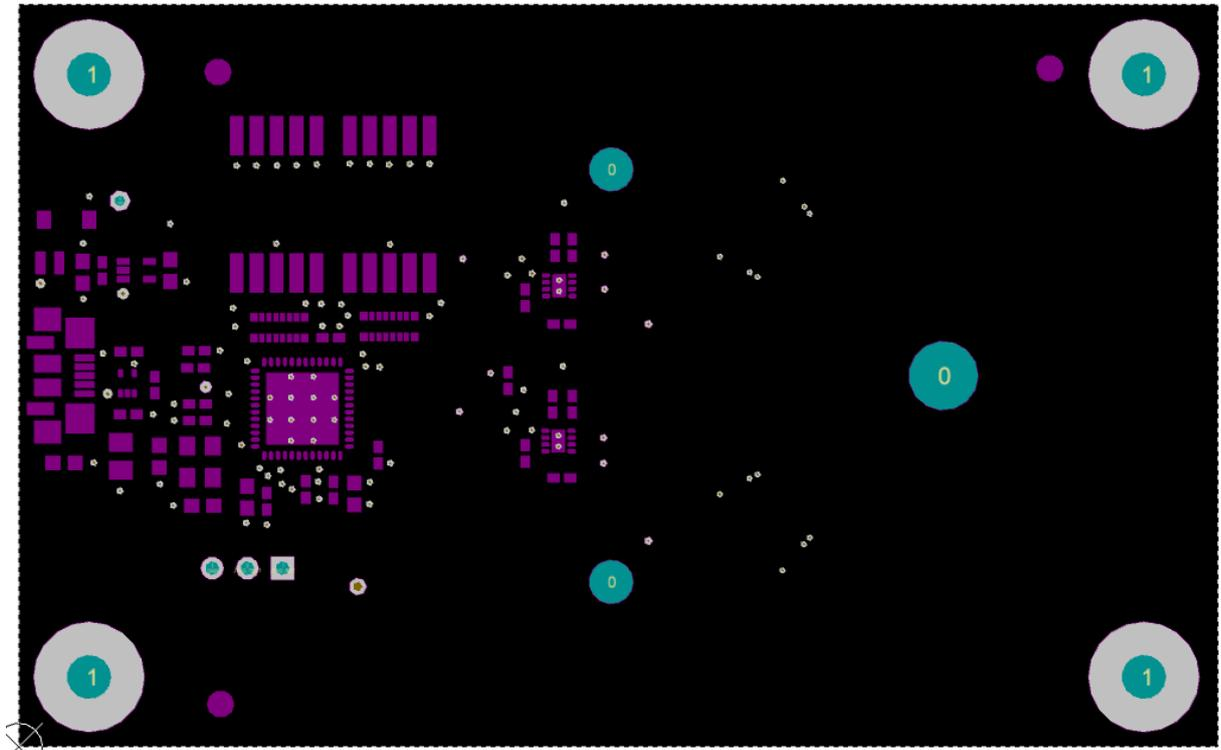
Figure 36: Sensor PCB Top Solder Mask
