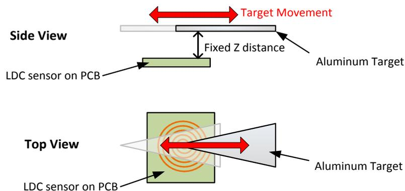
**Figure 9: Lateral Position Sensing with LDC**
