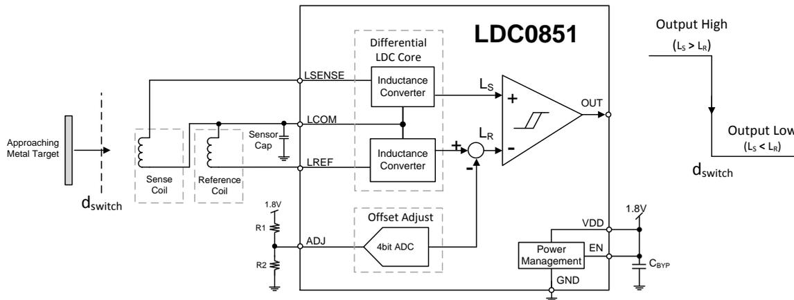
Figure 10: LDC0851 Block Diagram
