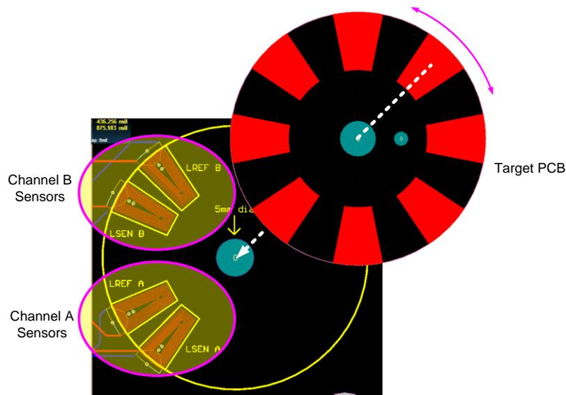
**Figure 13: Sensor and Target configuration**
