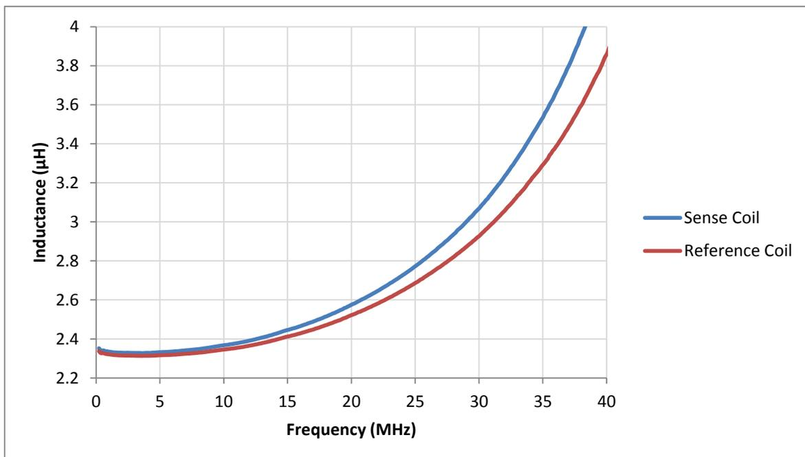
Figure 26: Coil characteristics using impedance analyzer
