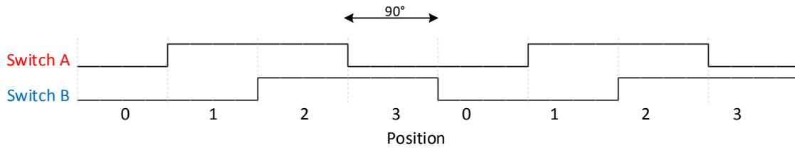
**Figure 14: Quadrature output signals out of phase by 90°**
