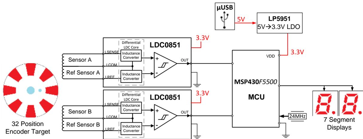
Figure 2: TIDA-00828 System Block Diagram
