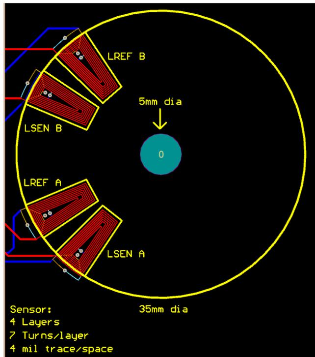
**Figure 21: Trapezoidal sensors placed according to Figure 18 (Right)**
