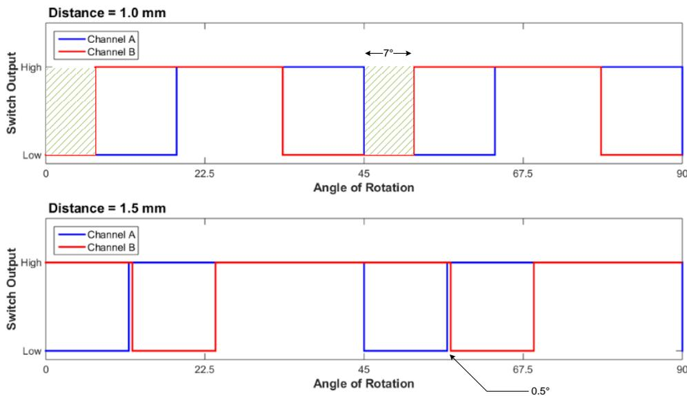
**Figure 29: Channel trough overlaps**
