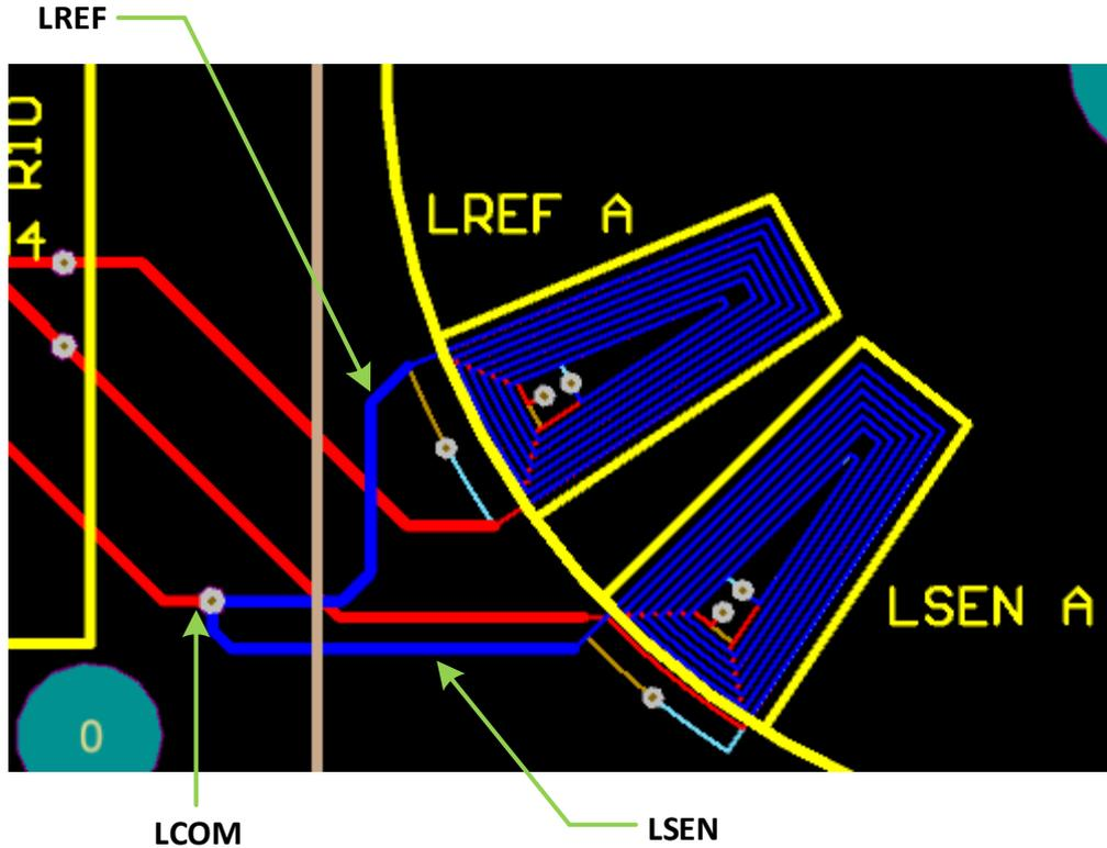
Figure 45: LSENSE, LREF and LCOM traces
