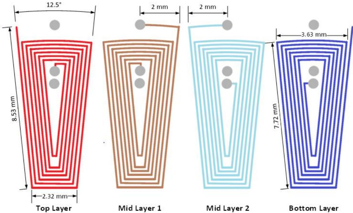
**Figure 20: Trapezoidal Sensor Geometry and Layers**
