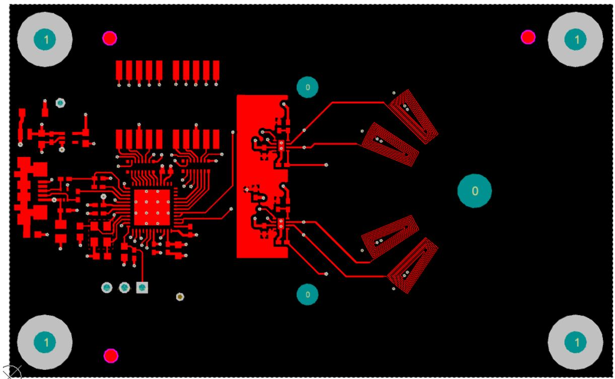
Figure 37: Sensor PCB Top Layer Routing
