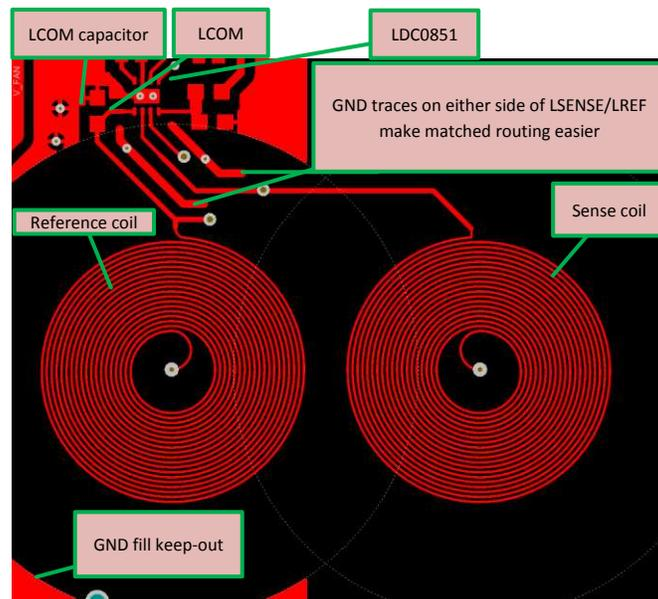
Figure 11. Sensor Configuration
