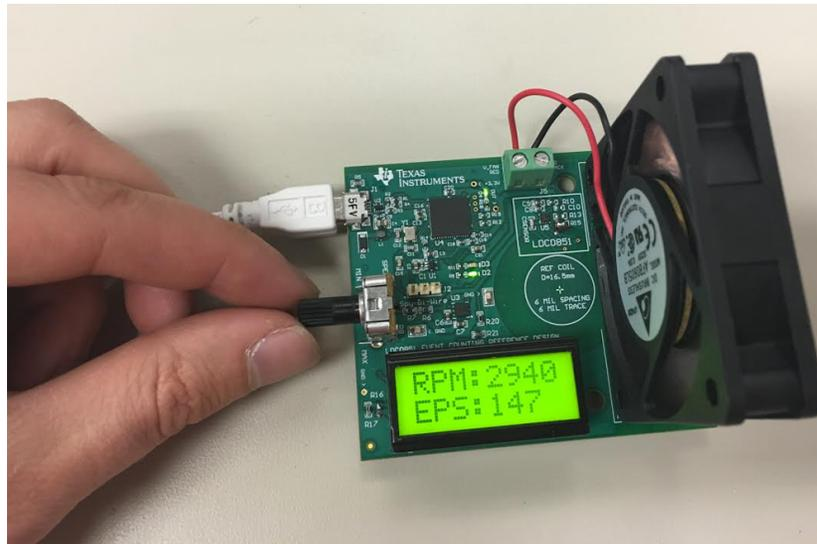
**Figure 3. TIDA-00851-LDC0851 Powered by USB Connection**
