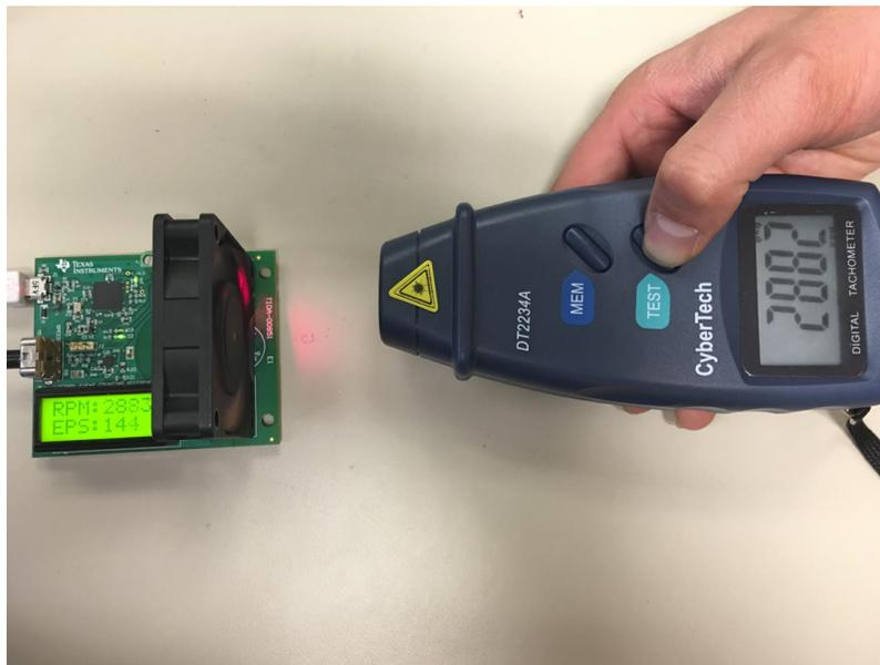
**Figure 17. Verification With Optical Tachometer**
