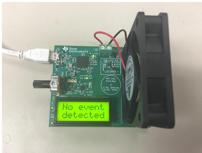
**Figure 5. Detected Speed After Dropping Below One Event per Second**
