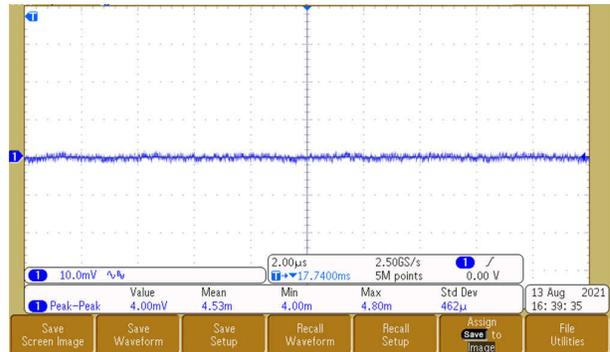
Figure 3-7. Output Voltage Ripple - 3.3 V
