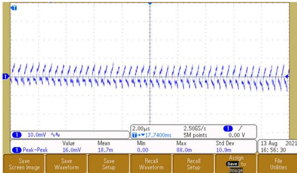
Figure 3-6. Output Voltage Ripple - 3.8 V
