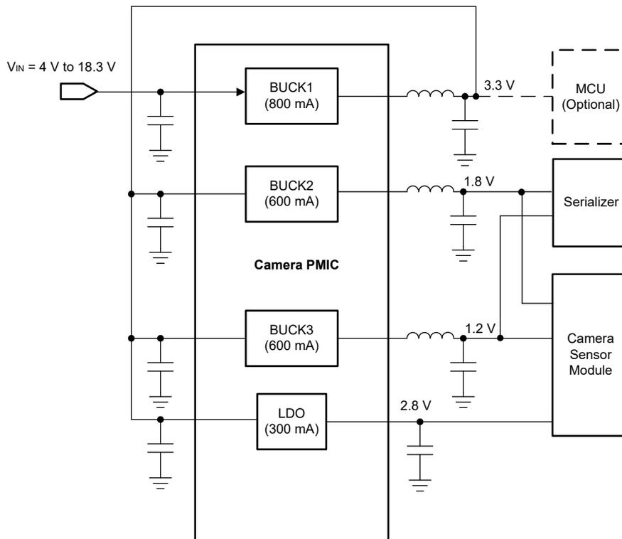
**Figure 2-5. TPS650320-Q1 Typical Application Circuit**
