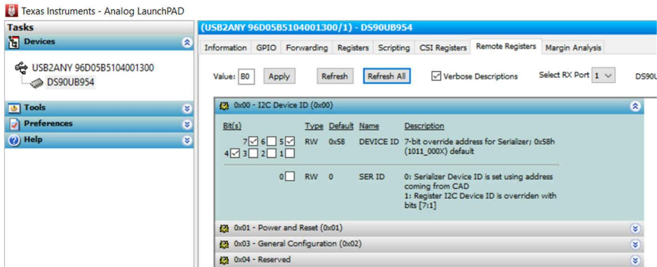
Figure 3-11. Serializer Remote Registers
