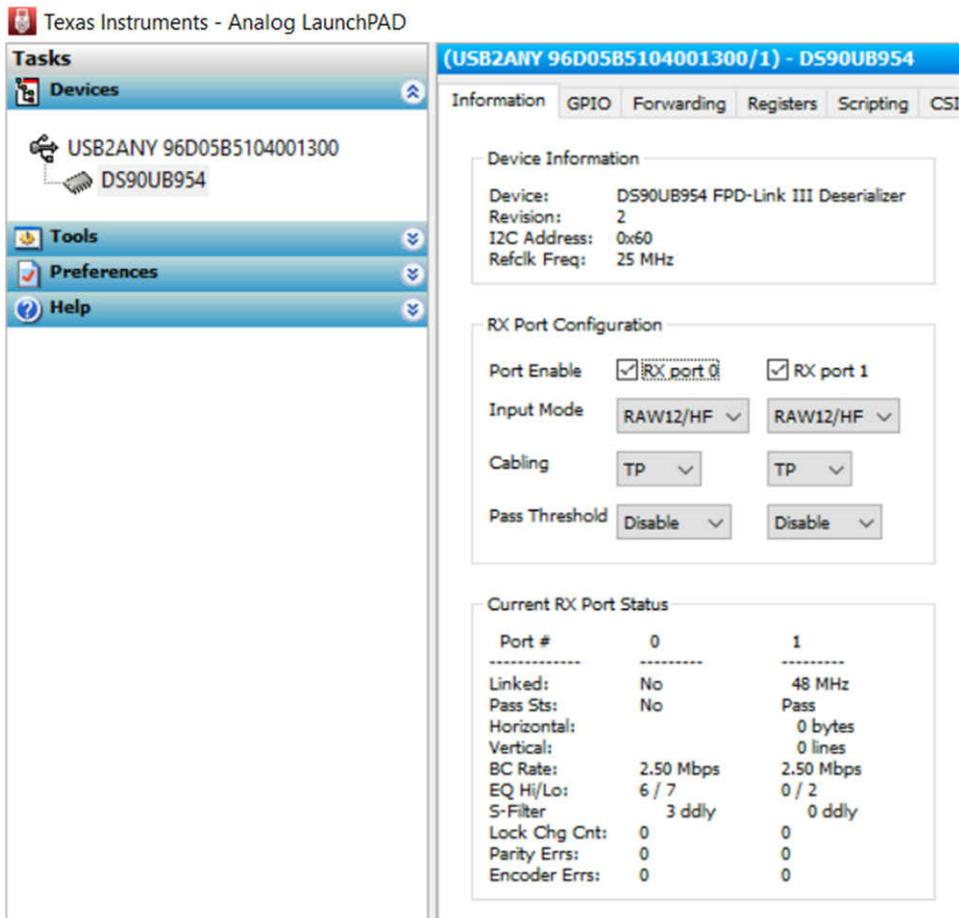
**Figure 3-10. Analog LaunchPad™ Link Confirmation**
