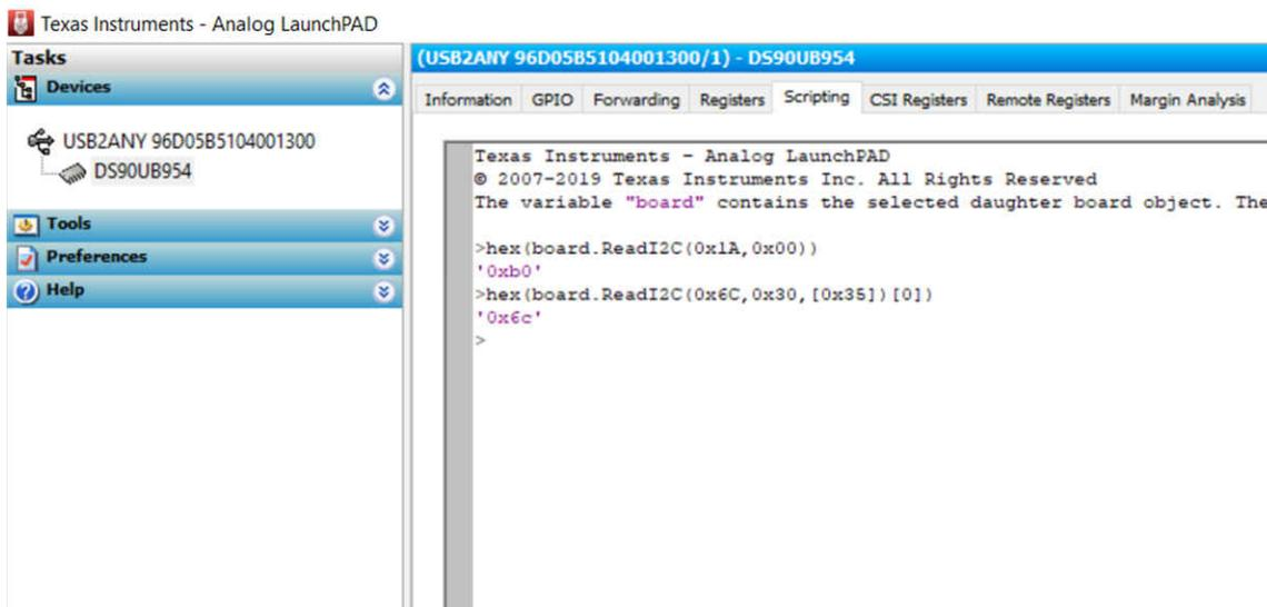
Figure 3-12. Back-Channel I2C Communication
