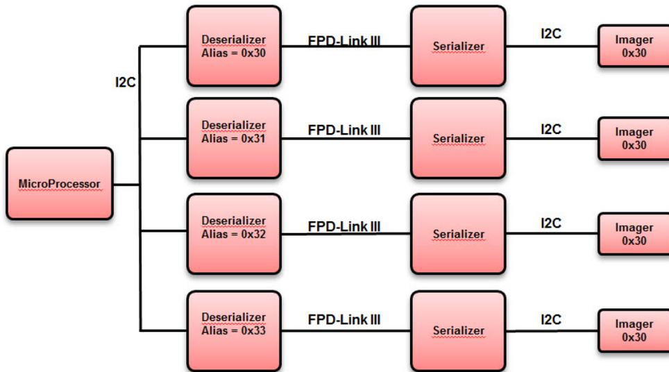
**Figure 6: I2C Address Aliasing**
