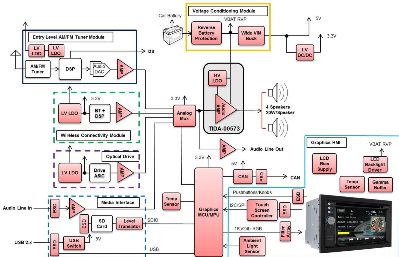
Figure 1. Automotive Head Unit With Integrated Display Example Highlighting TIDA-00573
