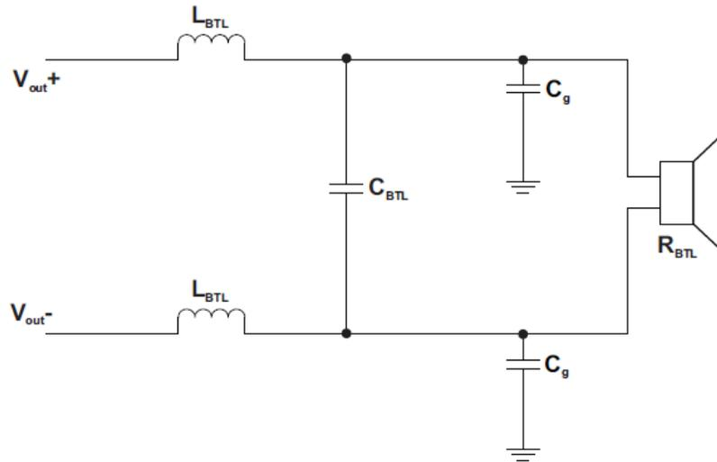
Figure 6. Diagram of Typical Class D Amplifier Output Filter
