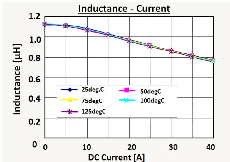
Figure 9. Inductance Versus Current in Metal Alloy Inductor
