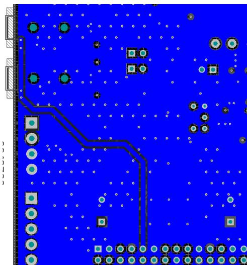
**Figure 20. Ground Trace on Bottom Layer**
