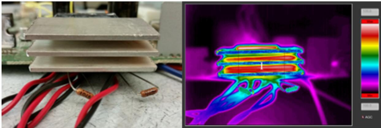
**Figure 28. Thermal Measurement of Class AB Amplifier—Front**
