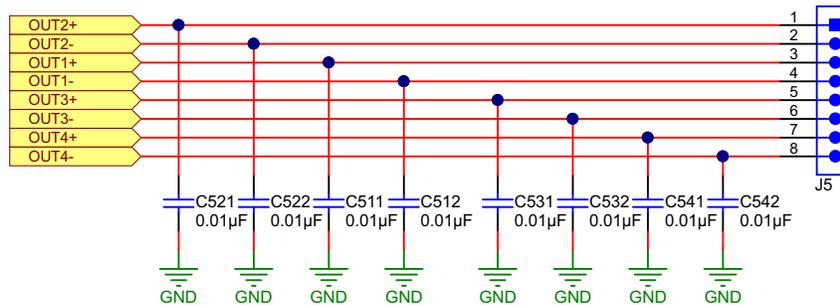
Figure 11. Filter at Connector
