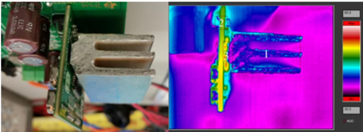
**Figure 27. Thermal Measurement of Class D Amplifier—Side**
