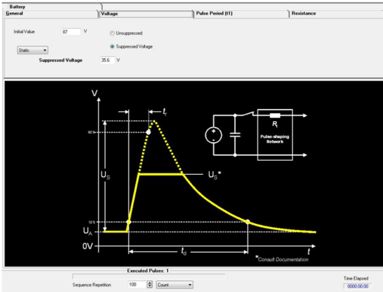
Figure 30. Load Dump Pulse 5b Configuration
