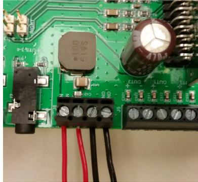
**Figure 12. Step 1— $V_{IN}$  Input Connection**
