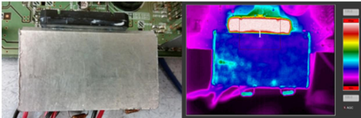
**Figure 29. Thermal Measurement of Class AB Amplifier—Side**
