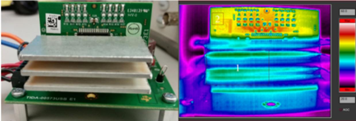
**Figure 26. Thermal Measurement of Class D Amplifier—Front**
