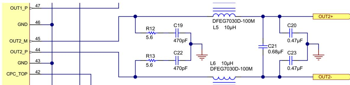
Figure 8. Output Filter in OUT2
