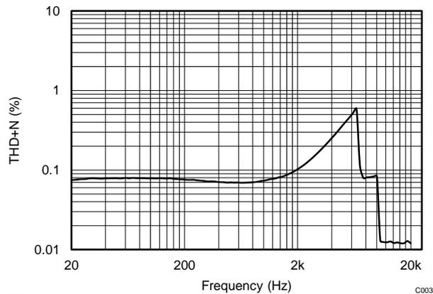
Figure 23. THD Versus Frequency at 1 W into 4 Ω
