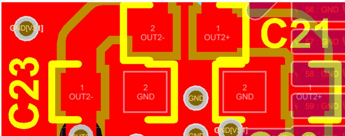
**Figure 18. Common-Mode Capacitors Layout**
