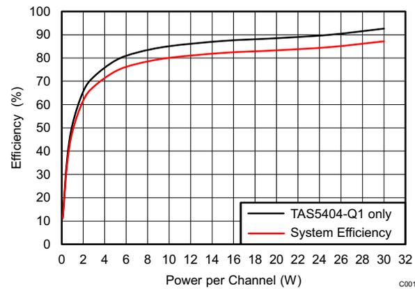
Figure 25. Efficiency of Device and System
