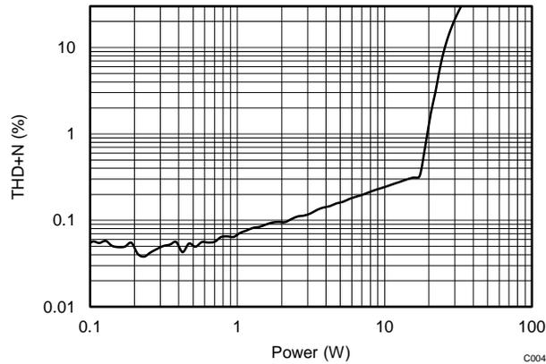
Figure 24. THD+N Versus BTL Output Power at 1 kHz into 4 Ω
