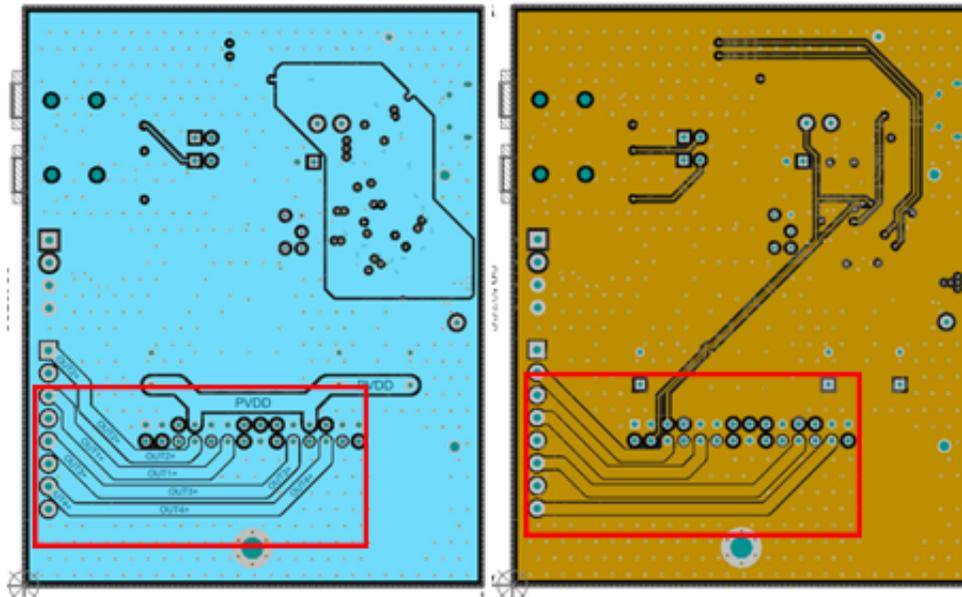
**Figure 21. Output Signal Traces Overlap for Current Cancellation in Layer 2 and Layer 3**
