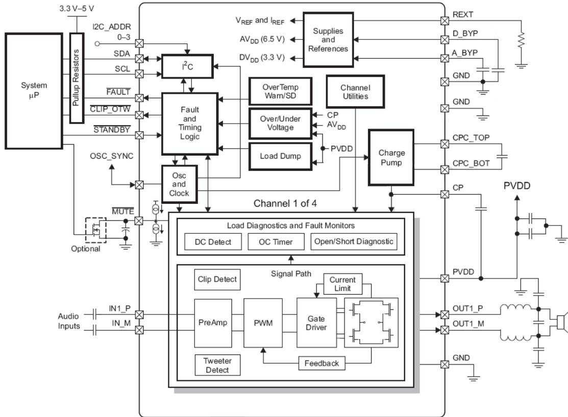
Figure 3. 25-W, Analog, Single-Ended Input, 4-Ch, Class D Amp With Load Dump Protection and I²C Diagnostics
