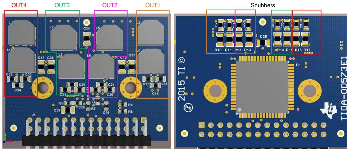
**Figure 19. Placement of Components—Daughterboard**
