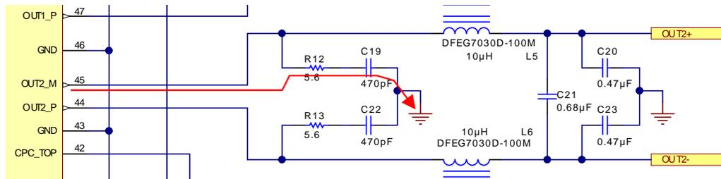
**Figure 17. AC Current Path in Snubber Circuits**
