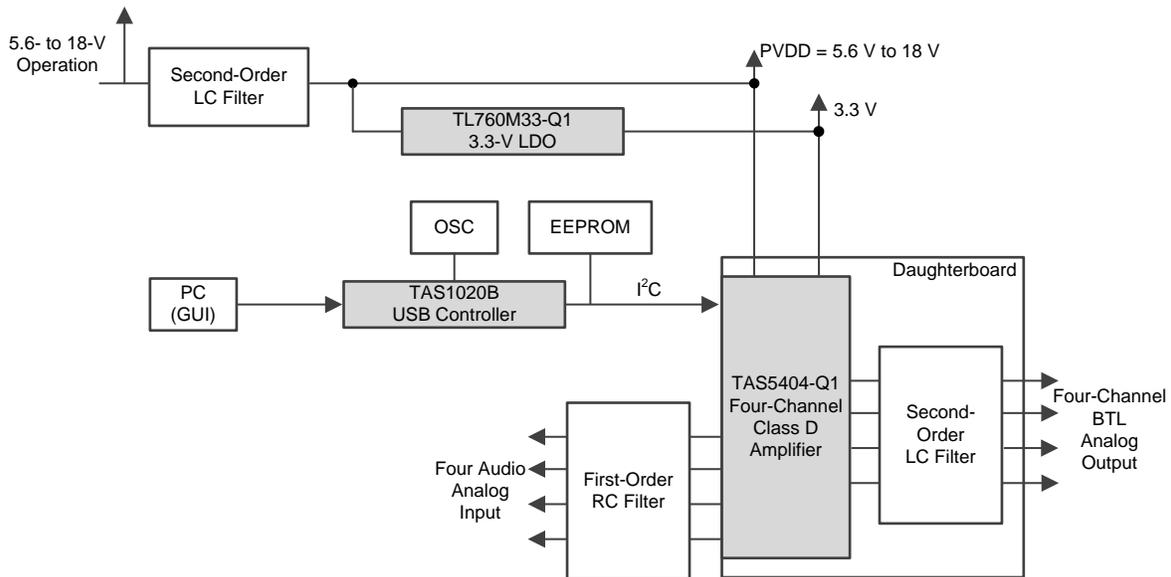
**Figure 2. Automotive, Four-Channel, Class D Amplifier for Head Unit**
