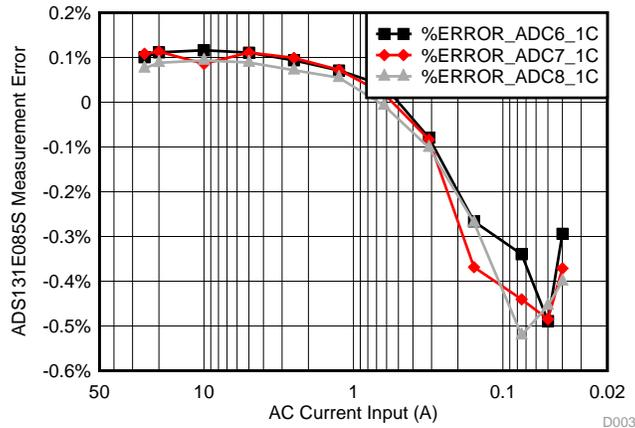
Figure 29. Input Current Vs ADC Measurement Error
