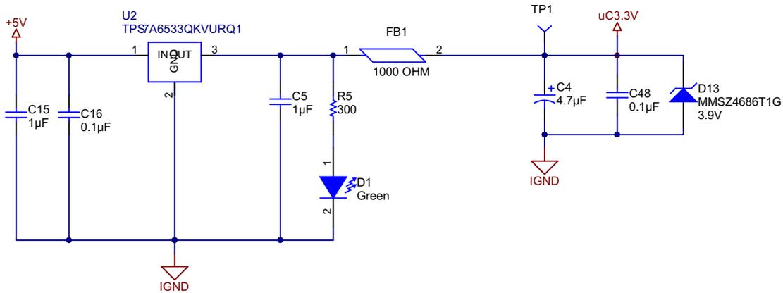
Figure 10. 3.3-V LDO for ADC and MCU Board
