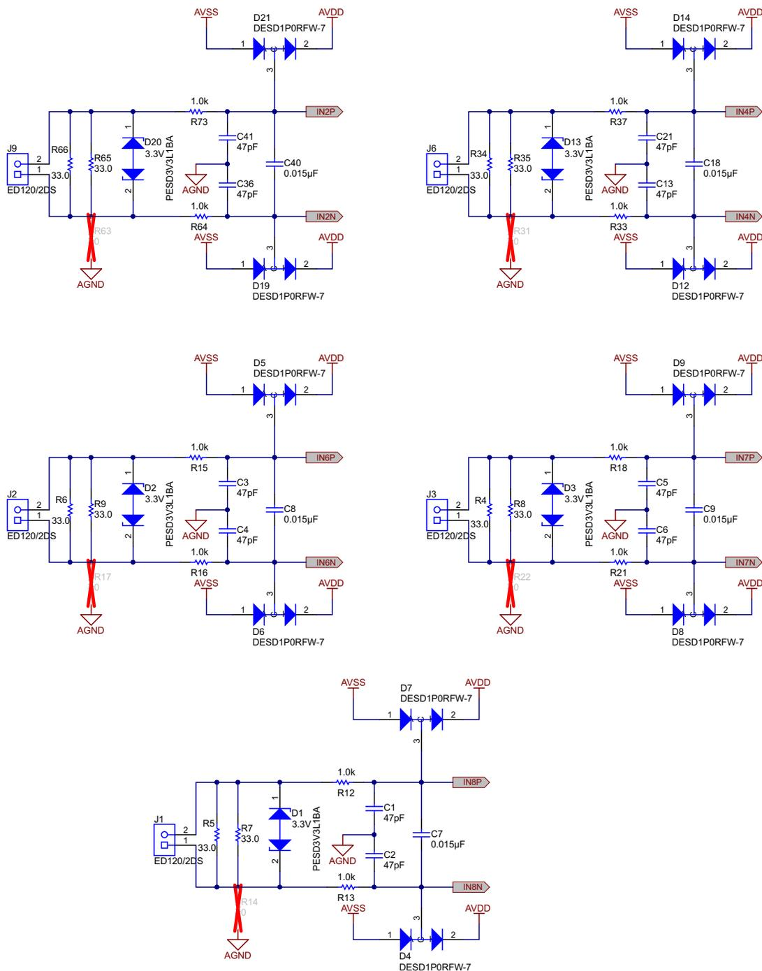
Figure 4. Current Input Connectors
