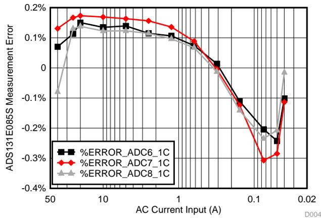
**Figure 30. Input Current Vs ADC Measurement Error (4-V Reference)**
