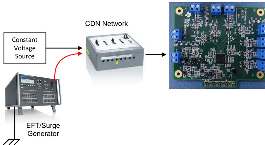
**Figure 34. Surge Setup for ADC Board**
