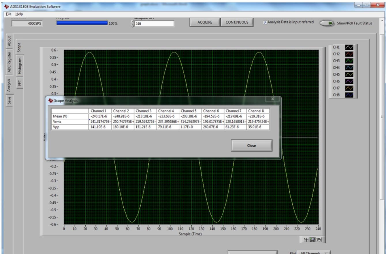
**Figure 26. RMS Readings for Captured Signal**
