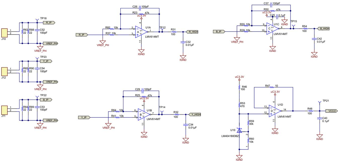
Figure 12. Earth Fault Current Signal Conditioning
