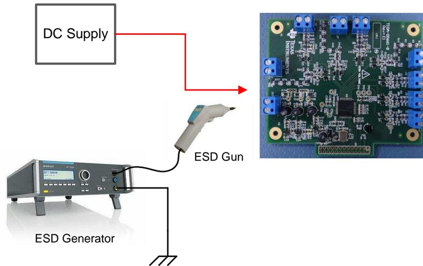
**Figure 35. ESD Setup for ADC Board**
