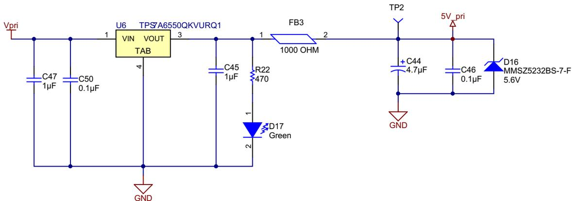
Figure 11. Primary-Side DC Output Regulator
