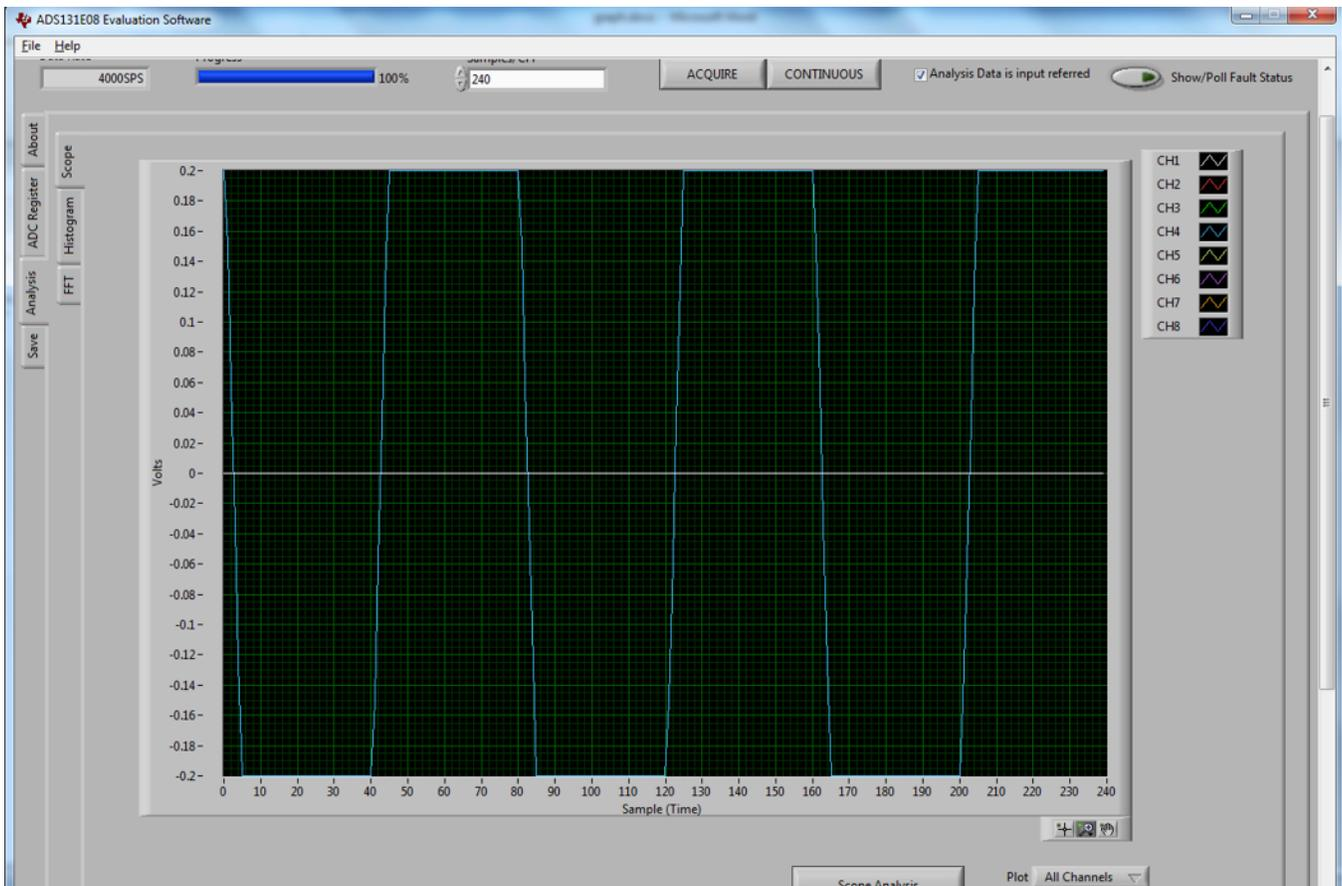
Figure 25. Waveform With Saturated Input
