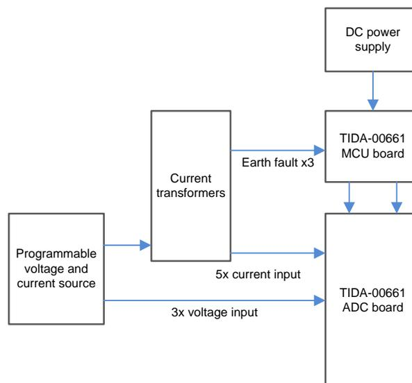
**Figure 20. ADC Board Interfaced to MSP430 MCU-Based Interface Board**
