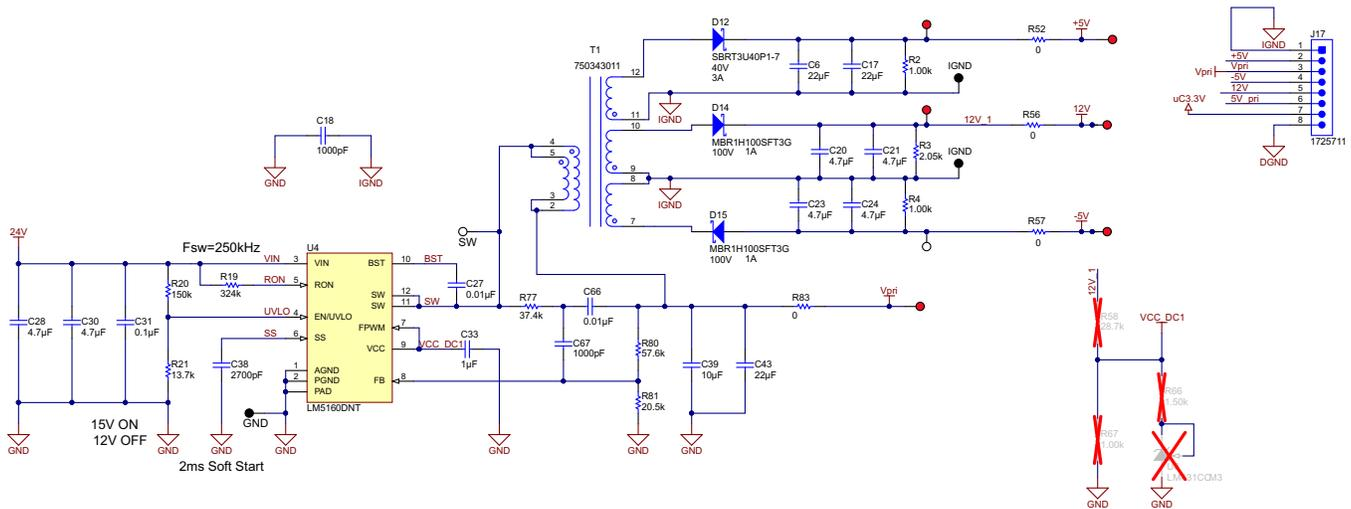
Figure 8. LM5160 Configured for Fly-Buck Operation
