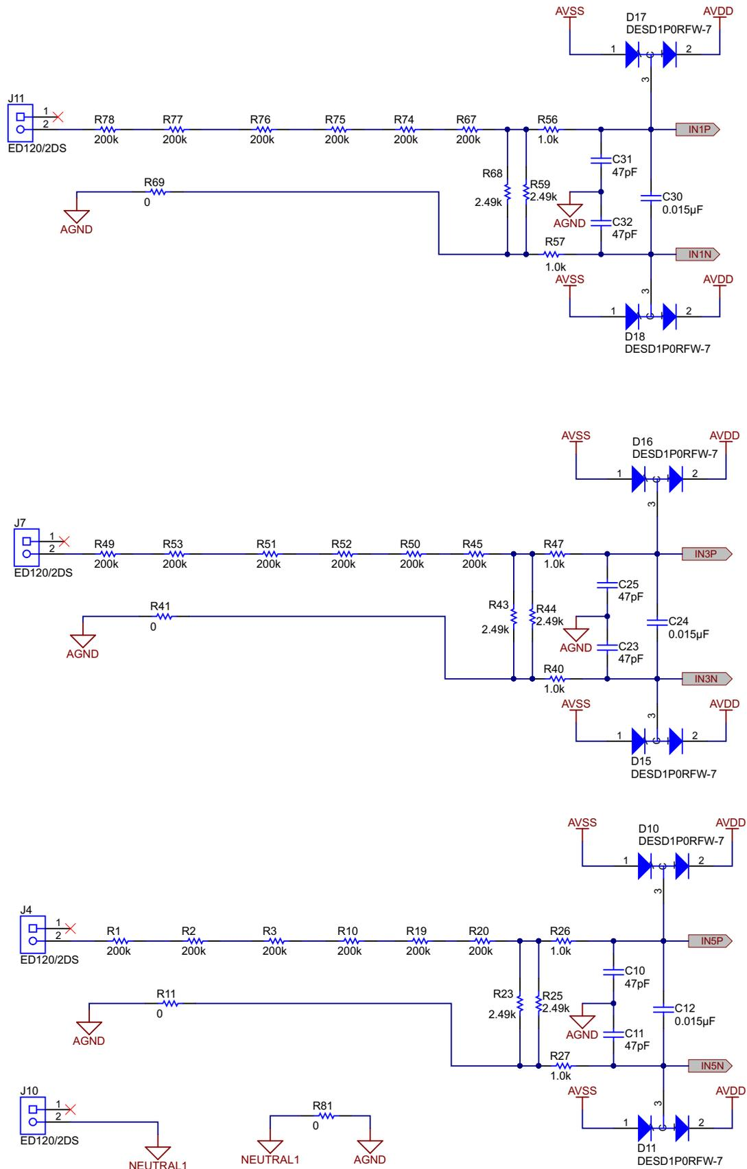
Figure 3. Voltage Input—Connector and Potential Divider for Three Phases
