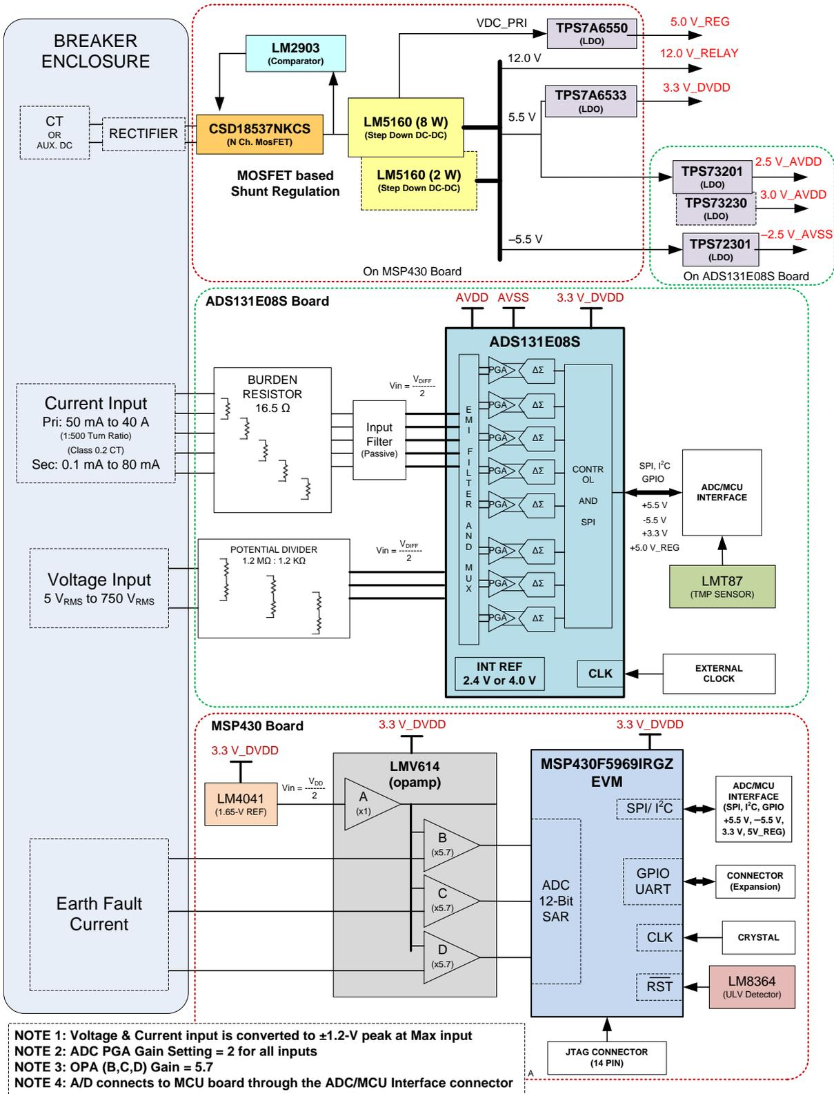
Figure 1. TIDA-00661 Block Diagram
