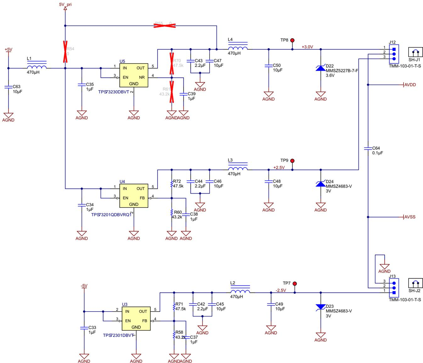
**Figure 9. LDO for ADC Analog Supply**
