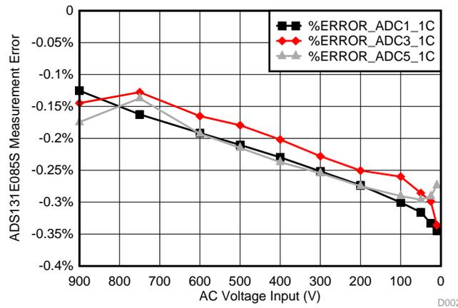
**Figure 28. Input Voltage Vs ADC Measurement Error (4-V Reference)**
