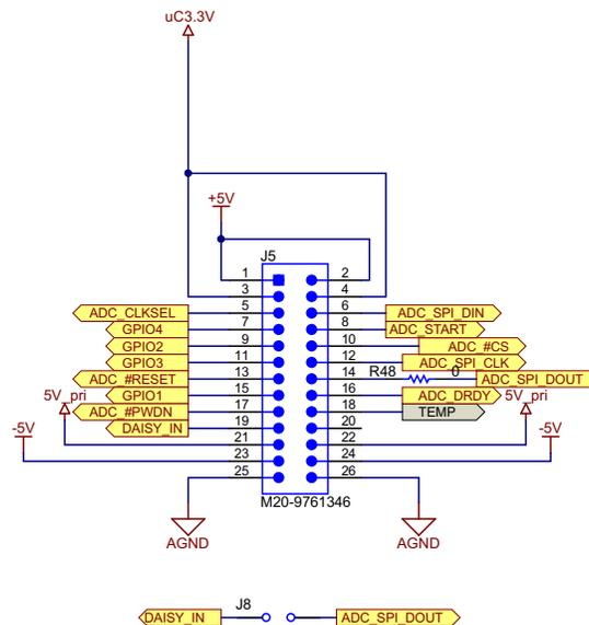
Figure 14. Interface Connector—From ADC Board to MCU Board
