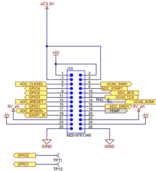
Figure 13. Interface Connector—From MCU Board to ADC Board
