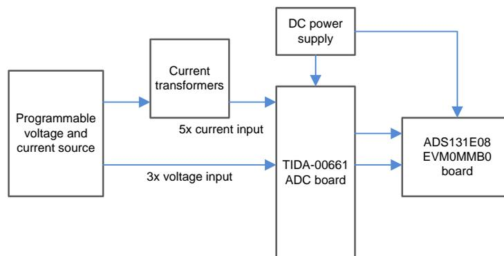
**Figure 19. ADC Board Interfaced to MMB0 Board**
