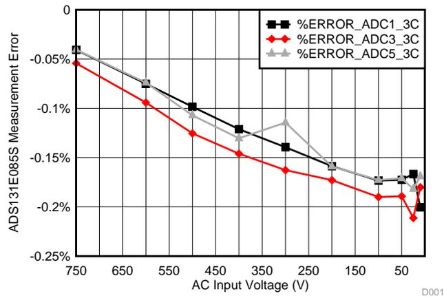
Figure 27. Input Voltage Vs ADC Measurement Error (2.4-V Reference)
