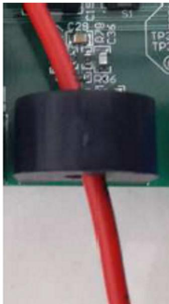
**Figure 30. Current Input Wire Through CT**
