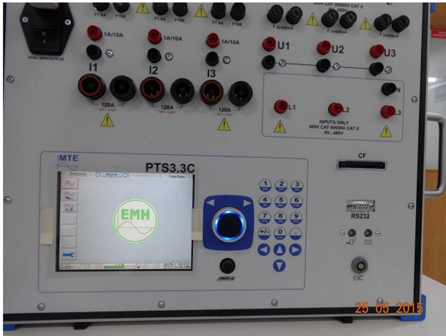
Figure 33. Three-Phase Test System with Programmable Power Source
