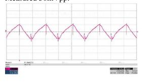
5V Ripple (C13) 20mV/div, 2usec/div Measured 70mVpp:
