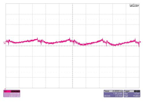
The output ripple voltage is shown in the figure below. The image was taken with the 12V output loaded to 4.2A and the input voltage set to 36V. (10mV/DIV, 1uS/DIV)
