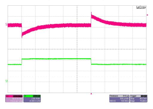
The photo below shows the 12V output voltage (ac coupled) when the load current is stepped between 2.2A and 4.2A. Vin = 24V. (100mV/DIV, 2A/DIV, 500uS/DIV)
