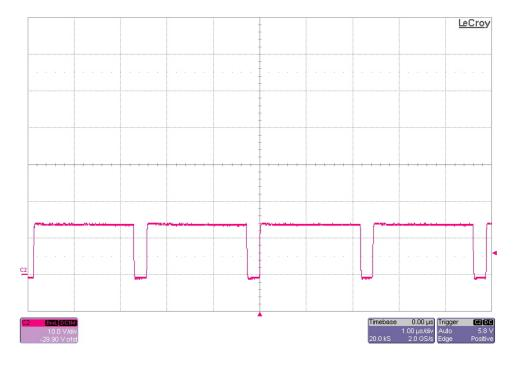
The photo below shows the switch node voltage. The input voltage is 36V and the 12V output is loaded to 4.2A. (10V/DIV, 1uS/DIV)
