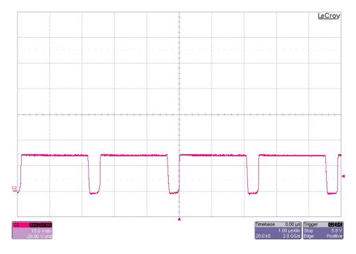
The photo below shows the switch node voltage. The input voltage is 36V and the 12V output is loaded to 0.55A. The converter has entered Discontinuous Conduction Mode. (10V/DIV, 1uS/DIV)
