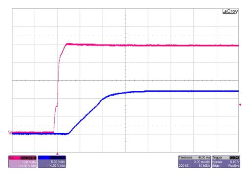
The photo below shows the output voltage startup waveform after the application of 24V in with the 12V output loaded to 4.2A. (5V/DIV, 2mS/DIV)
