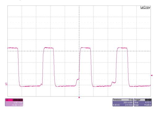
The photo below shows the FET switching voltage (TP3) for an input voltage of 6.4V and a 0.05A load. The converter has just transitioned to DCM at this load. (5V/DIV, 200nS/DIV)
