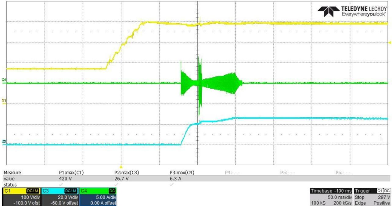
**4.6 120VAC/60Hz – Full Load (PSON high & S2 On=>25V/13.5A and 12V/1A at outputs)**
