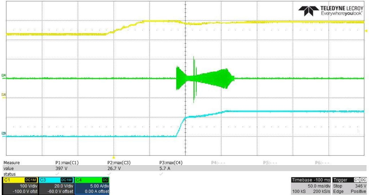
**4.8 230VAC/50Hz – Full Load (PSON high & S2 On=>25V/13.5A and 12V/1A at outputs)**
