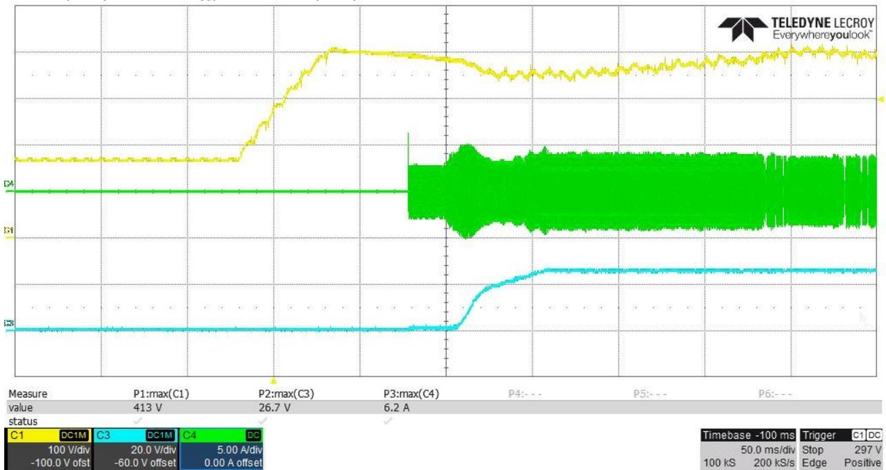
**4.7 230VAC/50Hz – No Load (PSON high & S2 On=>25V/0A and 12V/0A at outputs)**
