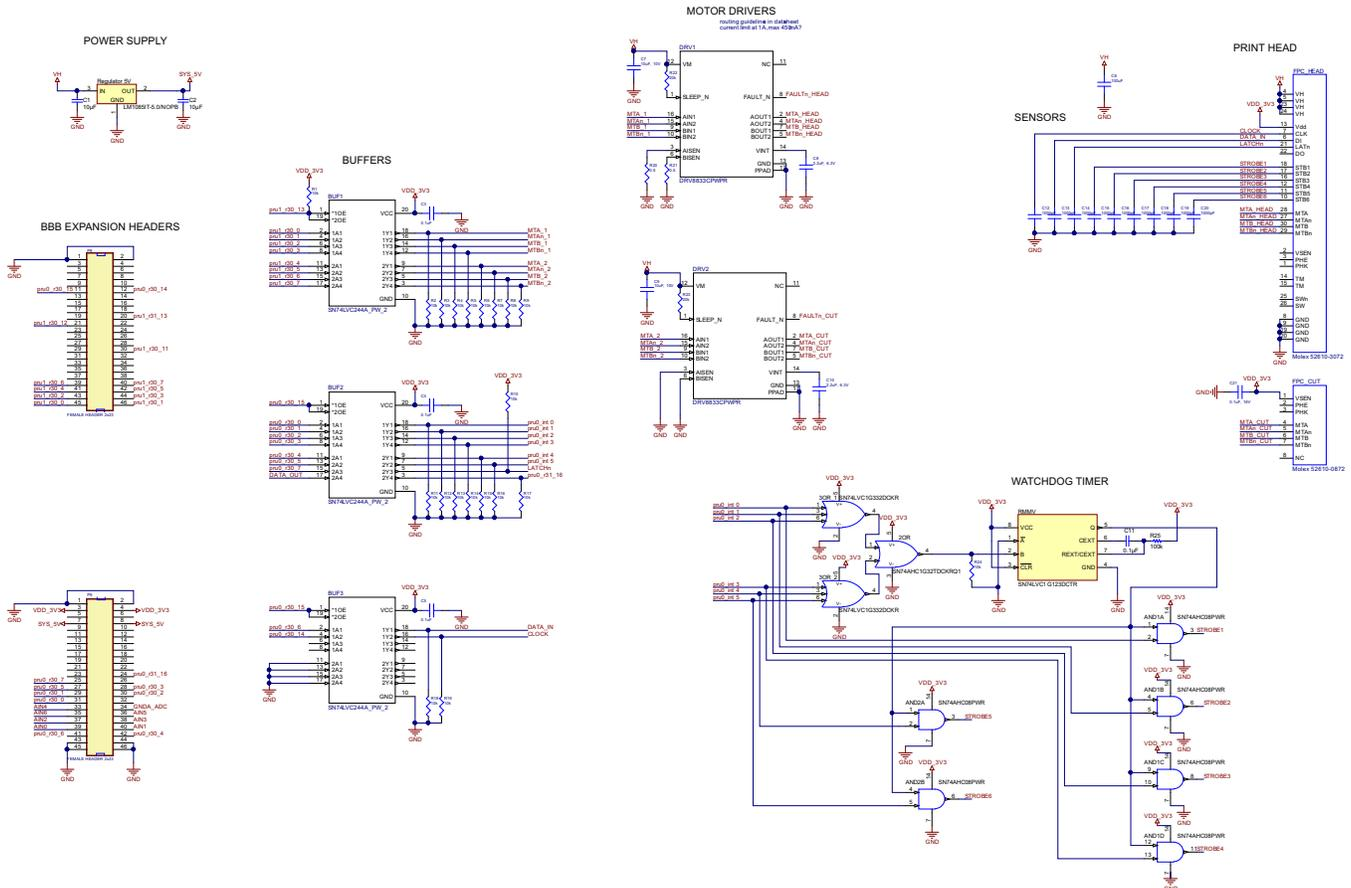
Figure 10. PRU Thermal Printer Schematic
