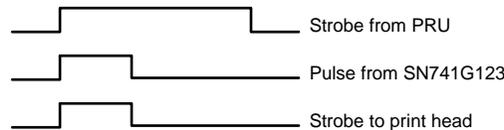
**Figure 4. Watchdog Circuit De-asserts Strobe if Asserted for Extended Period of Time**
