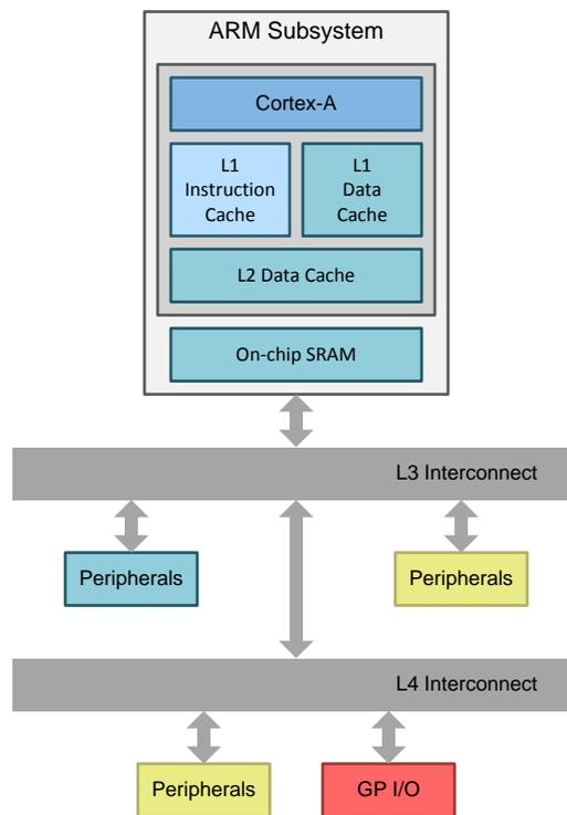
Figure 1. ARM Processor and Interconnects
