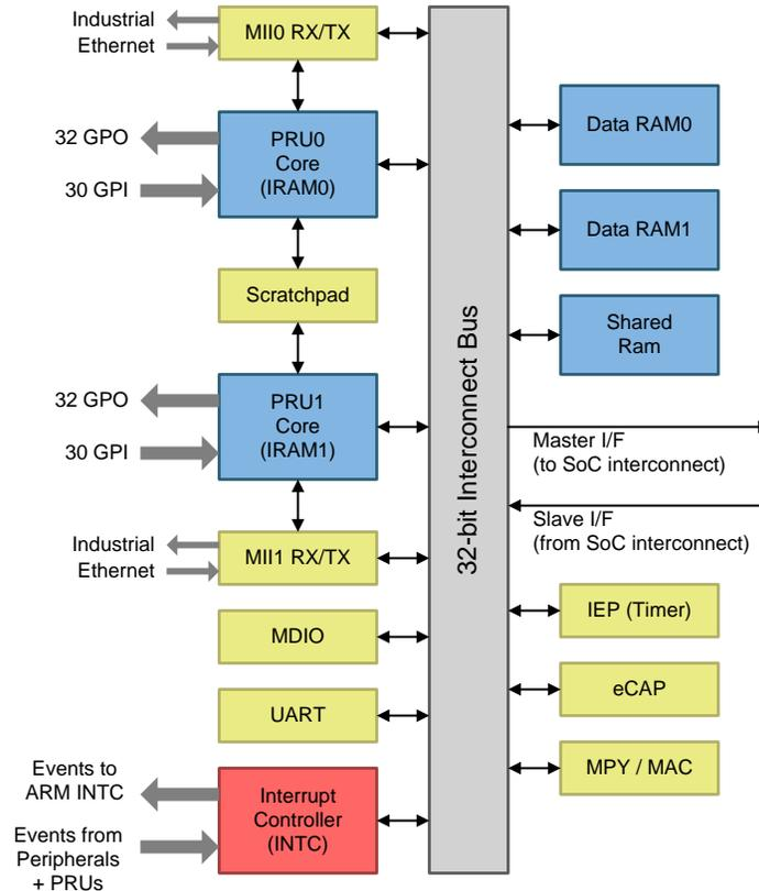
Figure 2. PRU Subsystem Block Diagram
