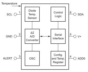
Figure 3. TMP102 Block Diagram
