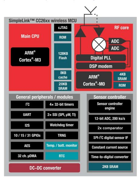
Figure 2. CC2650 Block Diagram
