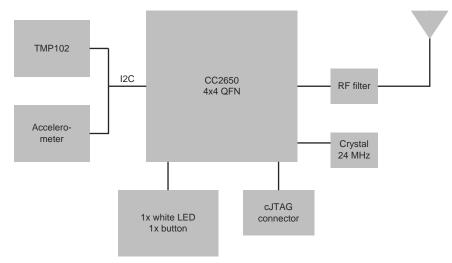
Figure 1. C2650 µTag Block Diagram
