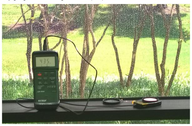
Figure 18. Light Meter Measuring Light Level in a Sunny Window
