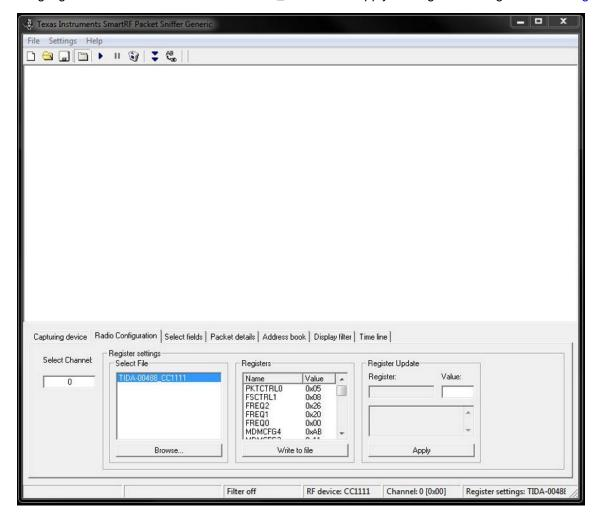
Figure 15. Radio Configuration and Monitor Screen
