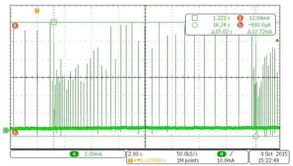
Figure 29. System Current Showing One Complete Transmit Cycle
