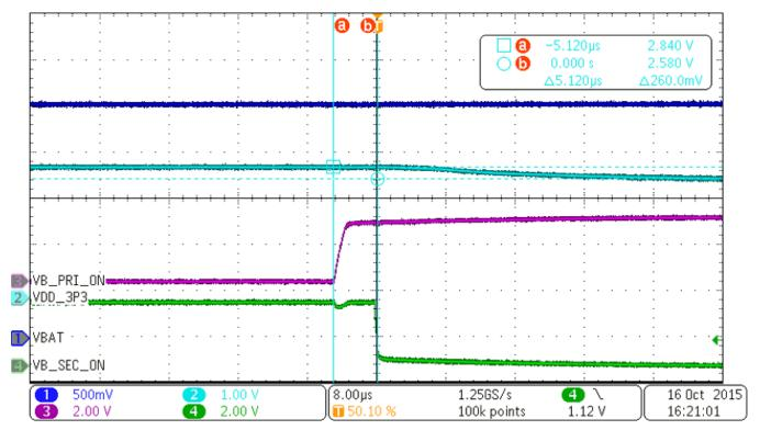
Figure 19. Power Transition From Primary Cell to the Capacitor Reservoir Charged by the Solar Cells
