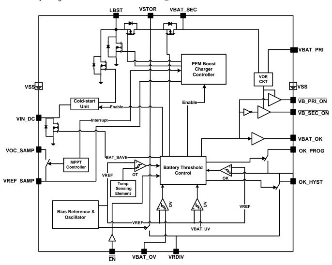
Figure 3. bq25505 Functional Block Diagram
