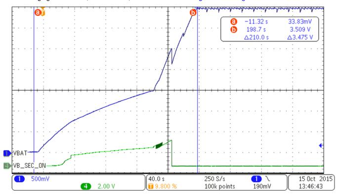
Figure 23. Capacitor Reservoir Charging Profile With 2,000 Lux Light Level
