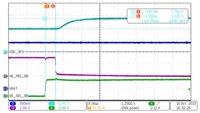
Figure 20. Power Transition From Primary Cell to the Capacitor Reservoir Charged by the Solar Cells
