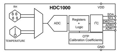
Figure 7. HDC1000 Functional Block Diagram
