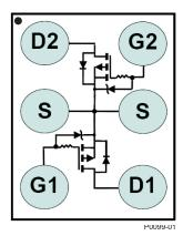
Figure 8. CSD75208W1015 Device Configuration
