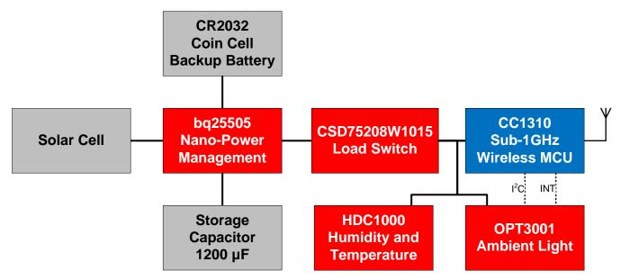
Figure 2. Energy Harvesting Ambient Light and Environment Sensor Node for Sub-1GHz Networks
