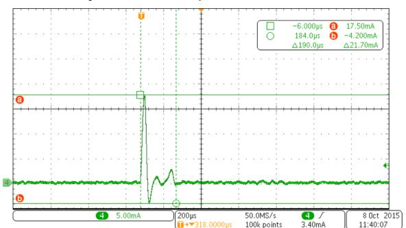
Figure 30. Current Transient During CC1310 Shutdown
