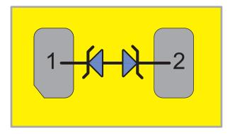
Figure 9. TPD1E10B06 Functional Block Diagram
