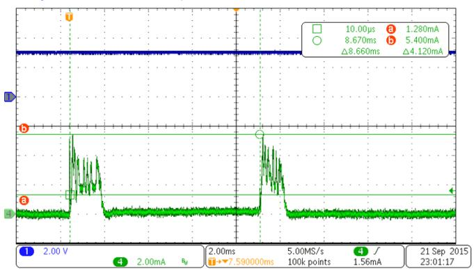
Figure 26. Current Profile During Conversion Trigger and Temperature-Humidity Sensor Read
