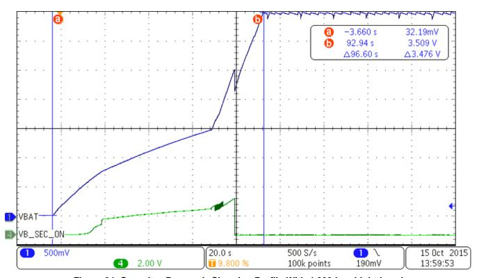
Figure 24. Capacitor Reservoir Charging Profile With 4,000 Lux Light Level
