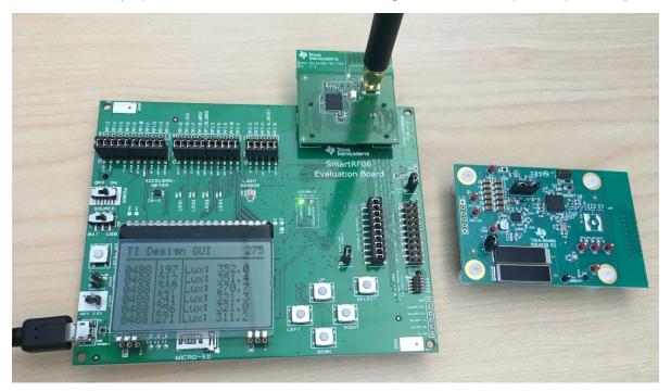
Figure 13. Sniffer Application Running on the SmartRF06 EVM With the CC13xxEM Radio
