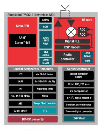
Figure 4. CC1310 Functional Block Diagram
