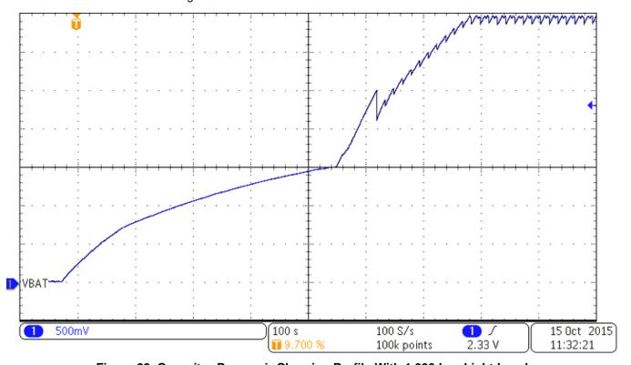
Figure 22. Capacitor Reservoir Charging Profile With 1,000 Lux Light Level
