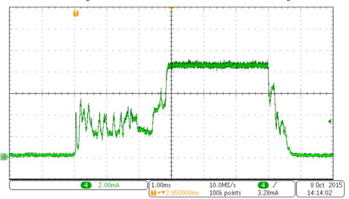
Figure 28. Light Sensor Data Read and RF Transmission
