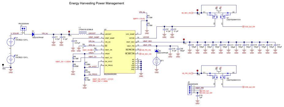
Figure 32. Energy Harvesting Schematic
