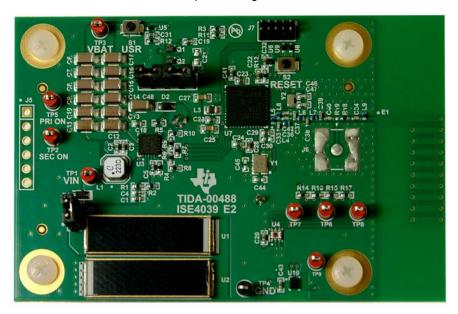
Figure 11. Energy Harvesting Ambient Light and Environment Sensor Node for Sub-1GHz Networks
