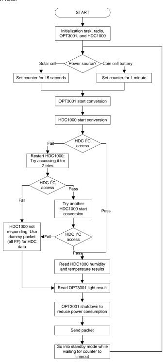
Figure 10. Firmware Flowchart
