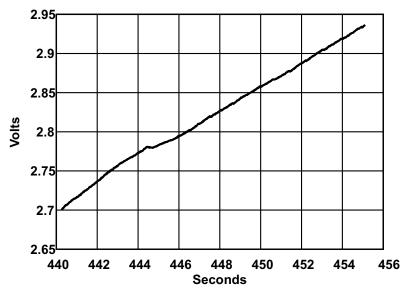
Figure 31. Voltage Rise Between Transmissions During Capacitor Reservoir Charging With 1000 Lux
