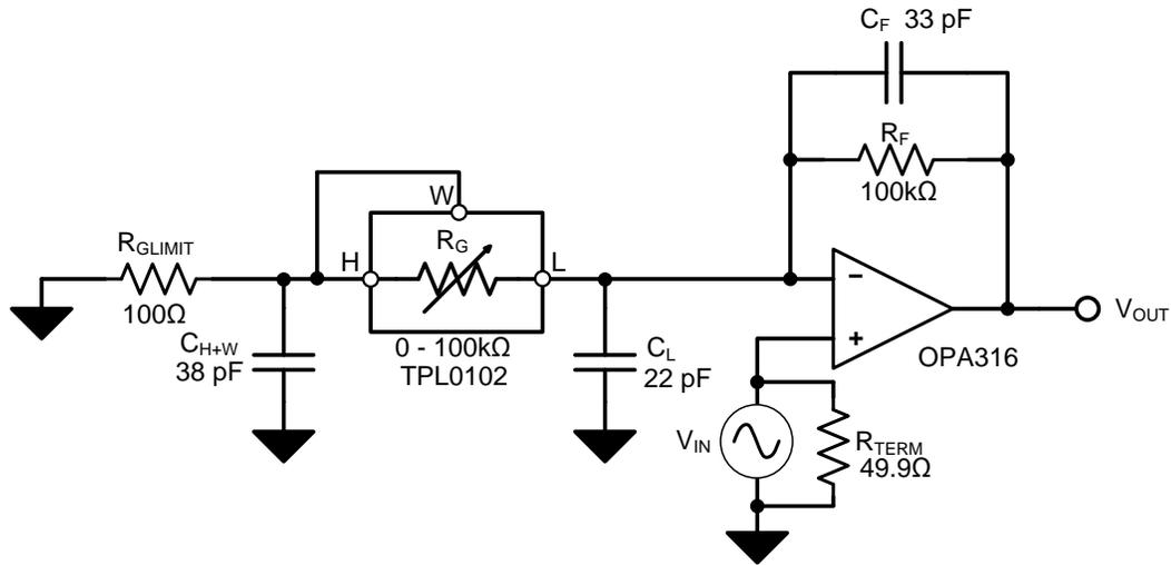
**Figure 4: Detailed Programmable Gain Amplifier Circuit Schematic**
