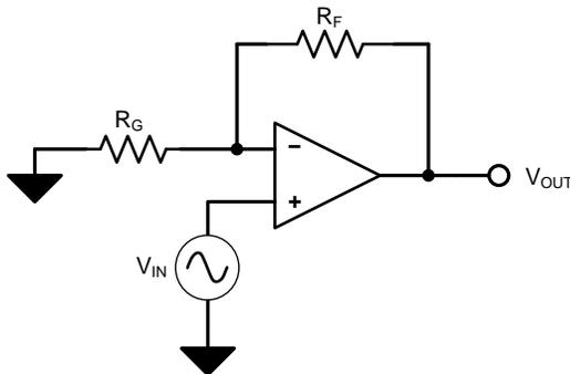
**Figure 2: Non-Inverting Amplifier Circuit**
