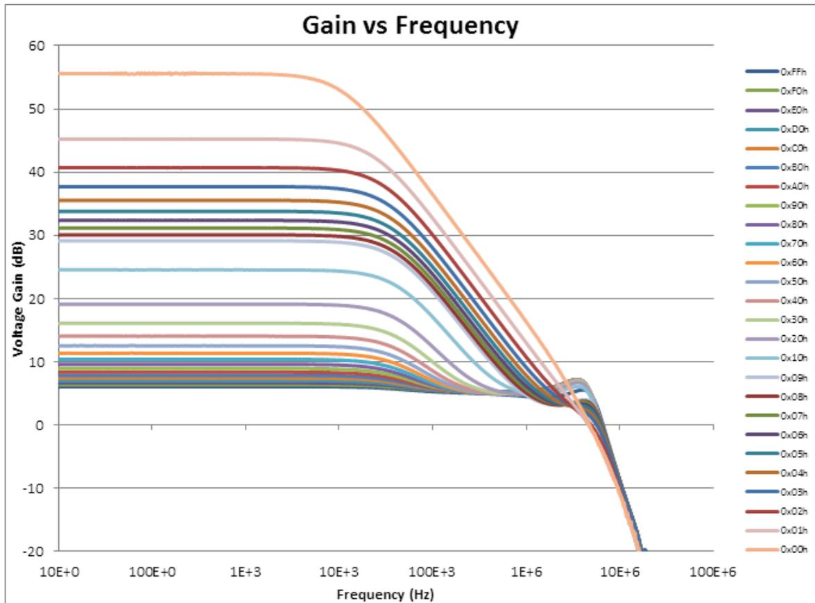
**Figure 1: Measured Transfer Function over the Full Range of Input Codes**
