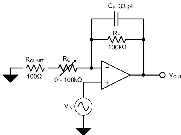
**Figure 3: Non-Inverting Programmable Amplifier Circuit Topology**
