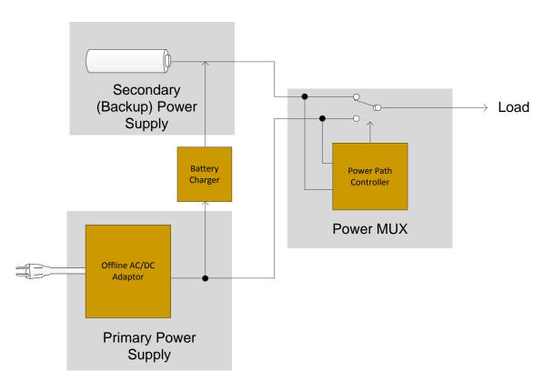
Figure 1: Battery Backup Block Diagram
