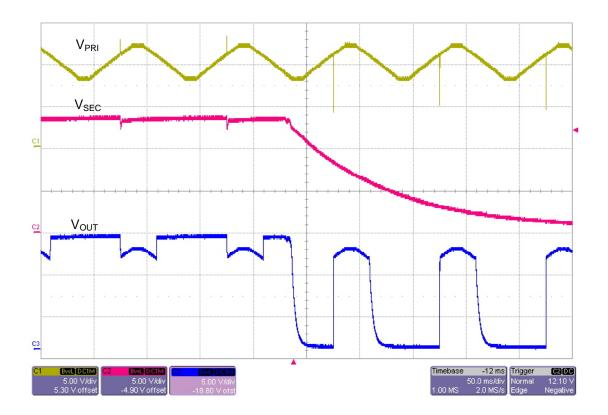
FIGURE 11: V<sub>PRI</sub> Ramp. V<sub>SEC</sub> = 13.5 to 0 V, Load = 65  $\Omega$
