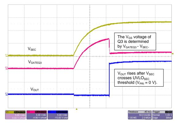
FIGURE 5: V<sub>SEC</sub> Startup. V<sub>PRI</sub> = 0 V, Load = 65  $\Omega$
