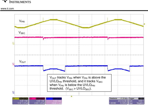
FIGURE 9: V<sub>PRI</sub> Ramp. V<sub>SEC</sub> = 13.5 V, Load = 65  $\Omega$
