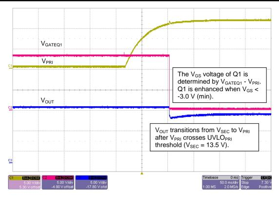
FIGURE 7: V<sub>PRI</sub> Startup. V<sub>SEC</sub> = 13.5 V, Load = 65  $\Omega$
