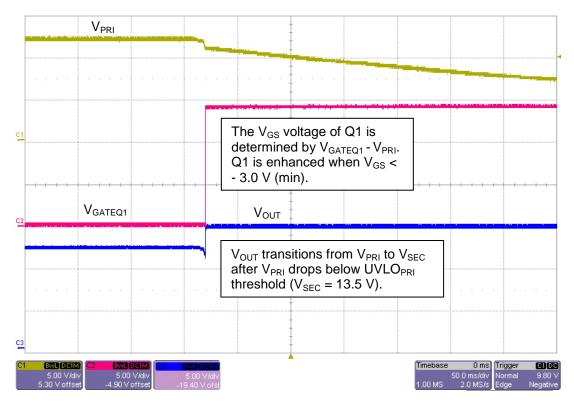
FIGURE 8: V<sub>PRI</sub> Falling. V<sub>SEC</sub> = 13.5 V, Load = 65  $\Omega$
