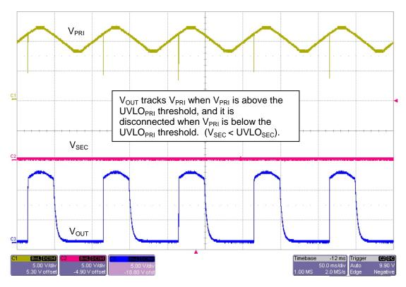
FIGURE 10: V<sub>PRI</sub> Ramp. V<sub>SEC</sub> = 0 V, Load = 65  $\Omega$
