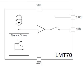
Figure 4: LMT70 Block Diagram
