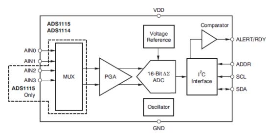
Figure 5: ADC1115 Block Diagram
