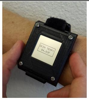
Figure 21: Holding the Button for Two Seconds Changes Temperature to Fahrenheit
