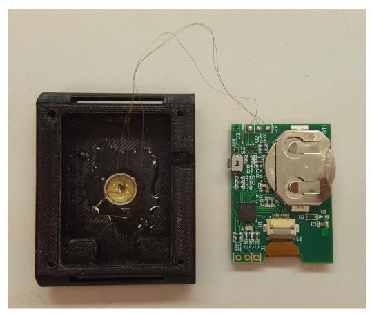
Figure 13: Wearable Design of Main PCB and Remote PCB Epoxied into Metal Cap
