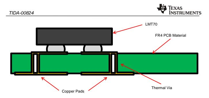
Figure 7: Remote PCB Side Cutout View
