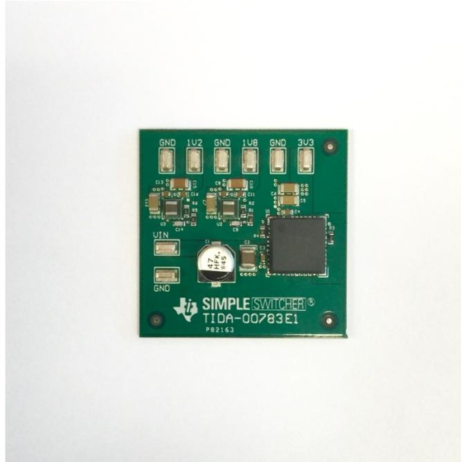
Figure 1 Reference board top view
