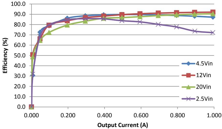
Figure 3 Power efficiency
