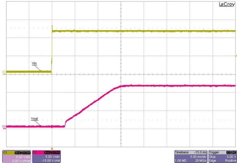
**Figure 7 Power up into no load at 12V input**
