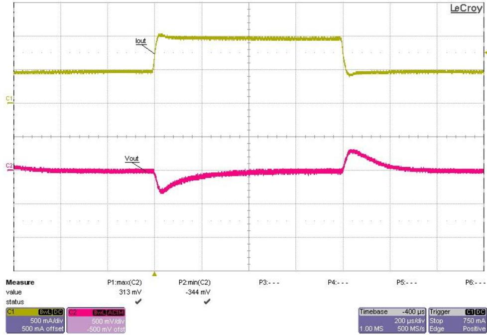
Figure 14 Output load transient response at 20V input
