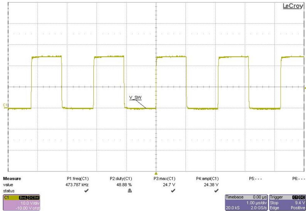
Figure 10 Switch node voltage at full load, 12V input
