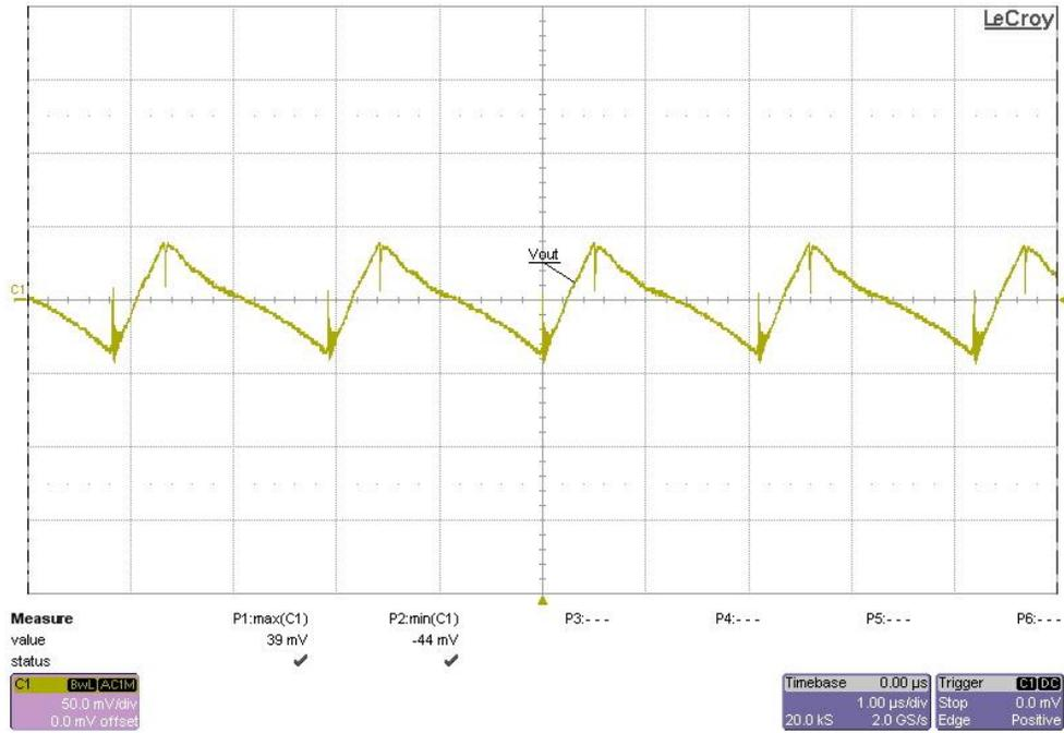
Figure 15 Output ripple at full load, 4.5Vin
