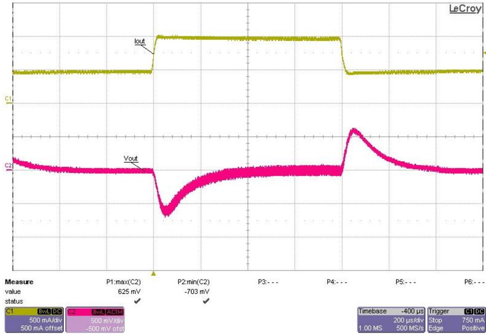
Figure 12 Output load transient response at 4.5V input
