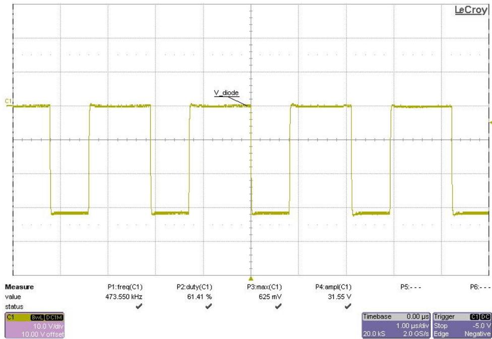
**Figure 11 Output diode anode (+) to cathode (-) voltage at full load, 20V input**
