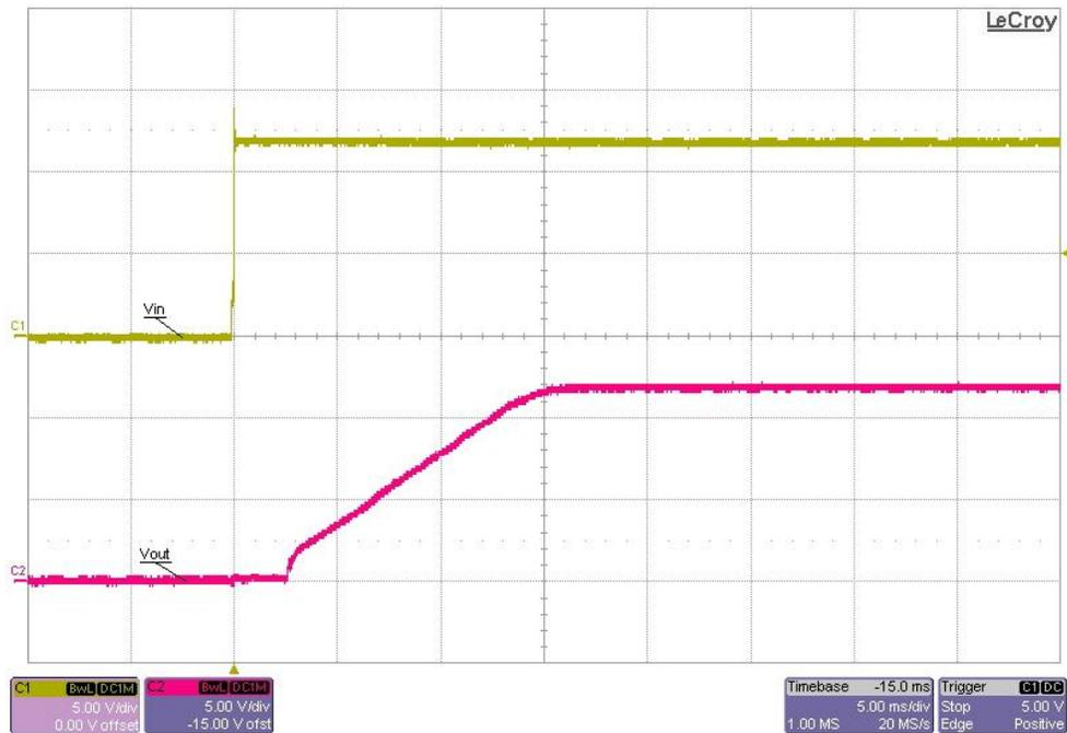
**Figure 8 Power up into full load at 12V input**
