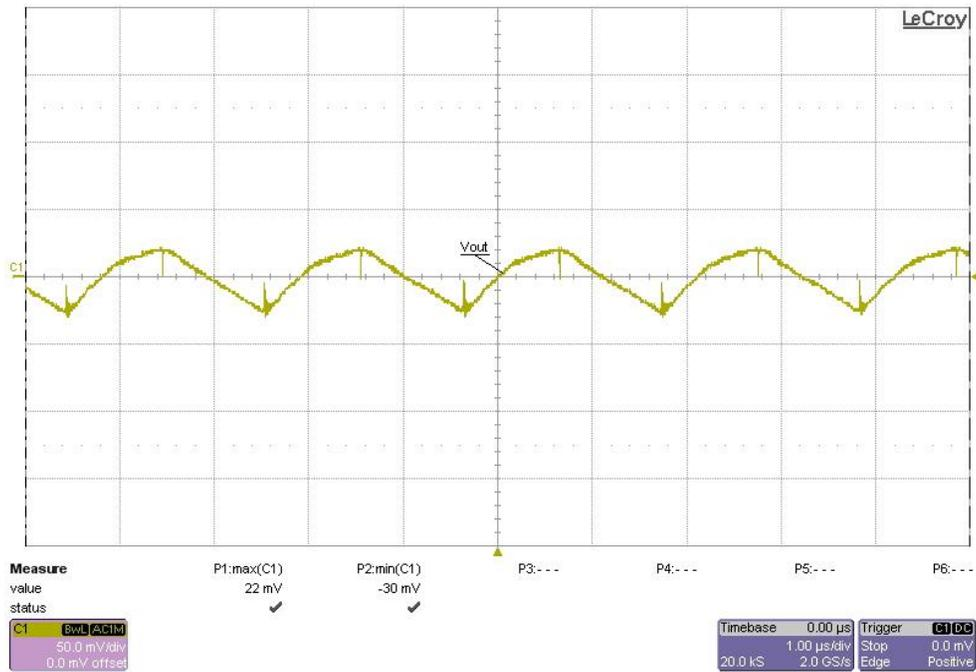
Figure 16 Output ripple at full load, 12Vin
