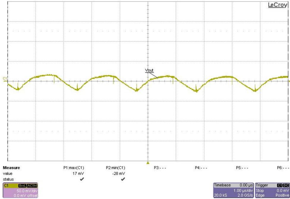
Figure 17 Output ripple at full load, 20Vin
