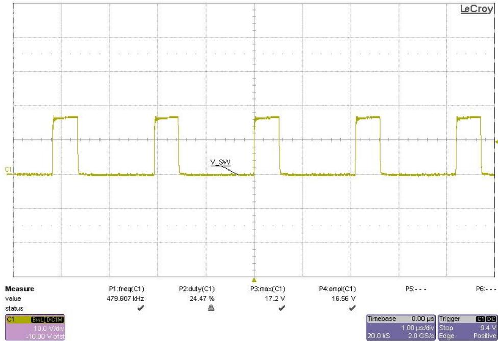
Figure 9 Switch node voltage at full load, 4.5V input
