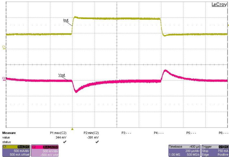
Figure 13 Output load transient response at 12V input
