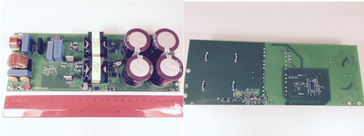
Load: 2 LED strings in parallel. Max. LED current each string: 0.35A
