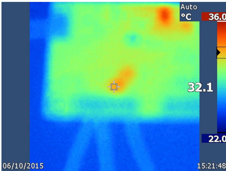
Figure 60. TPS54116-Q1 Inductor, Full Load, Steady State
