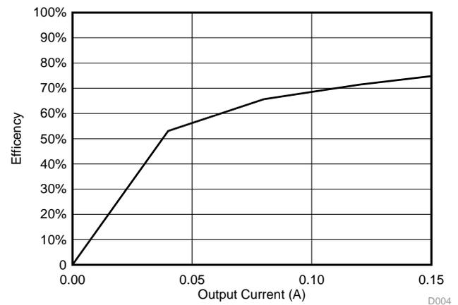
Figure 30. VCAN Efficiency ( $V_{IN} = 3.3\text{ V}$ )
