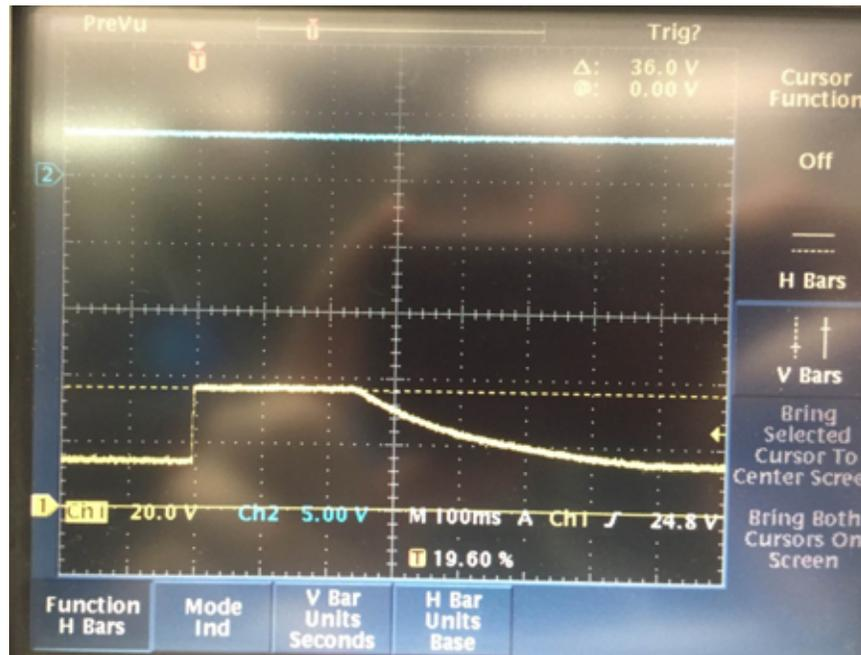
**Figure 71. Wide  $V_{IN}$  Output Undisturbed During Load Dump Pulse**
