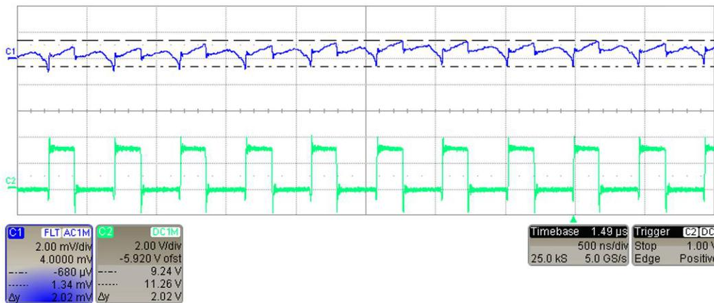
Figure 43. V\_CORE, VOUT = 1.06V, IOUT = 1.2A
