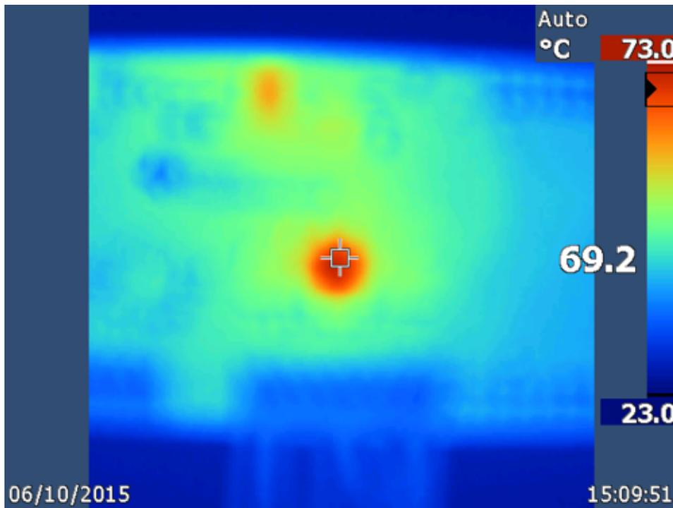
Figure 57. LP8731 IC, All Four Rails Full Load, Steady State
