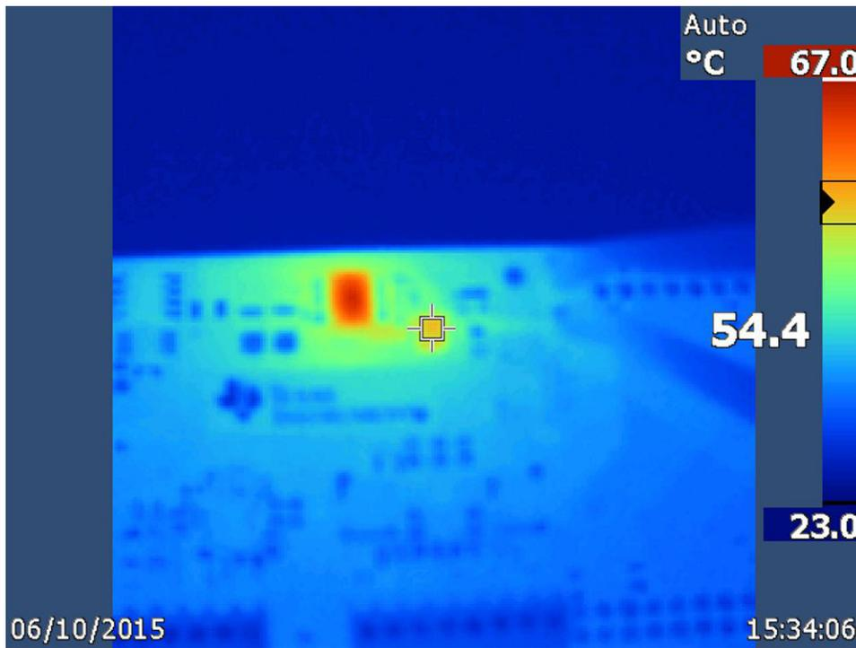
Figure 55. LM53603 (Wide-VIN Buck) Inductor, Full Load, Steady State
