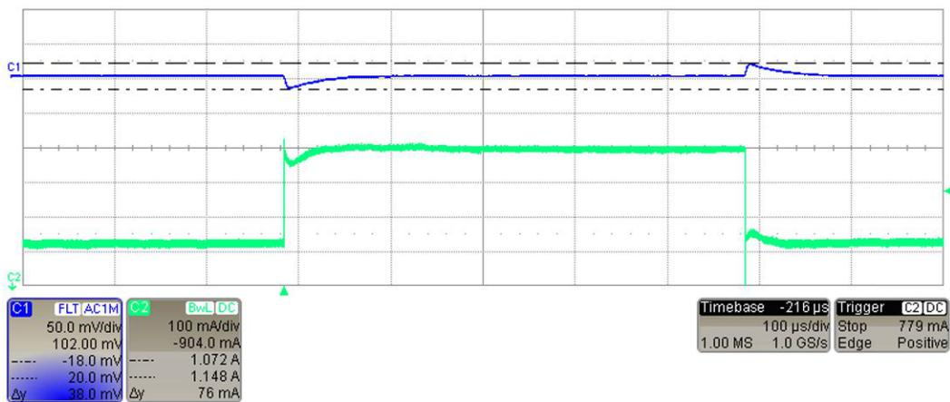
Figure 49. VDDQ, VOUT = 1.5 V, IOU\_STEP = 250 mA
