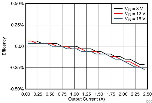
Figure 32. V3PV Load Regulation 0 to 2.5 A, 8 to 16 V<sub>IN</sub>
