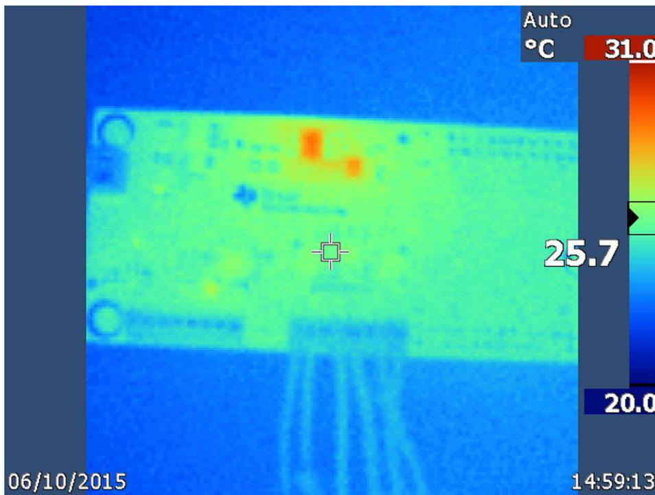
Figure 56. LP8731 IC, No Load, Steady State
