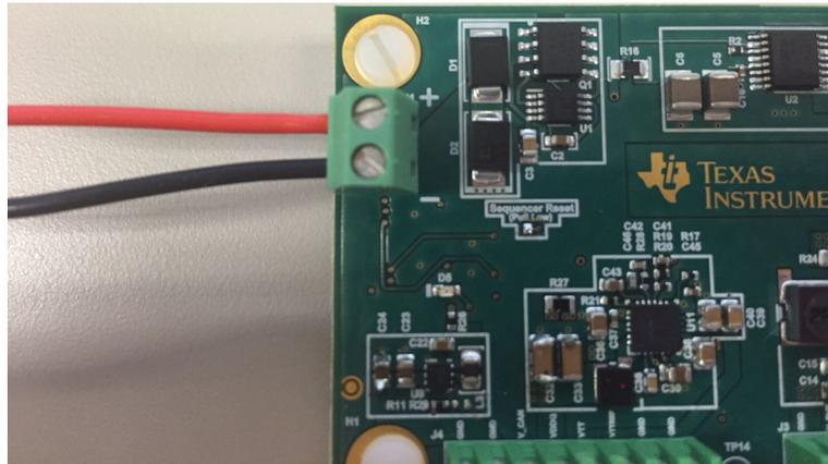
**Figure 13. Board Input Terminal**
