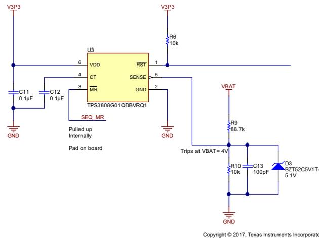
**Figure 9. TPS3808-Q1 Voltage Supervisor**
