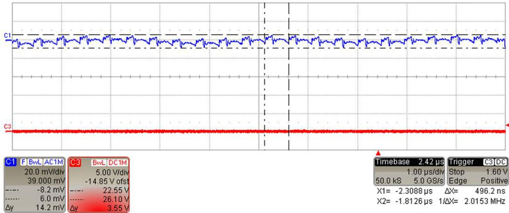
Figure 41. V3P3, VOUT = 3.3V, IOUT = 2.5A
