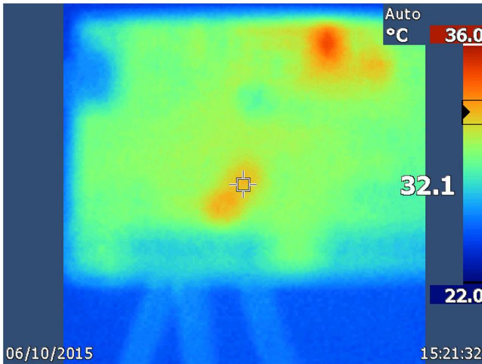
Figure 59. TPS54116-Q1 IC, Full Load, Steady State
