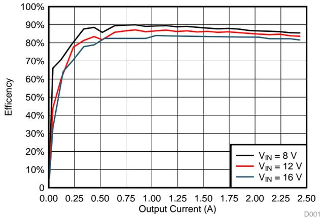
Figure 27. V3P3 Efficiency
