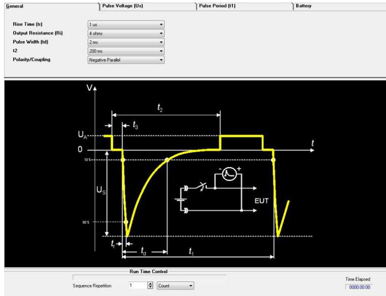
Figure 26. AutoStar Setup for Pulse 1
