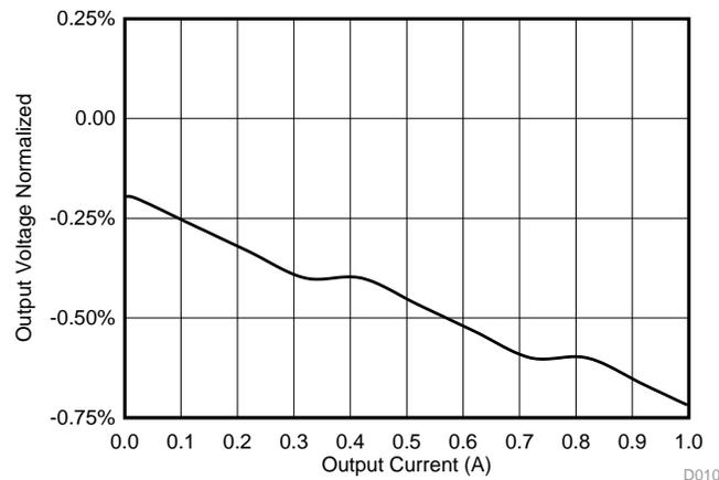
Figure 36. VDDQ Load Regulation 0 to 1 A (V<sub>IN</sub> = 3.3 V)
