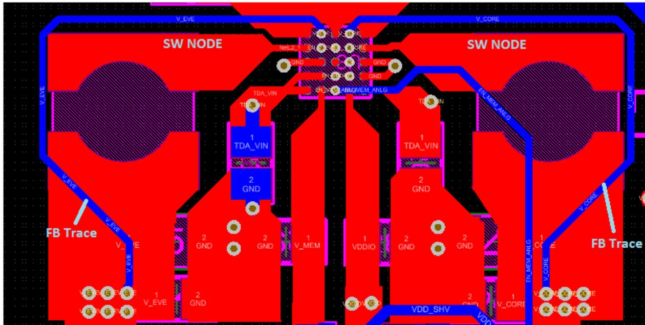
Figure 72. Routing Feedback Traces Around Switch Nodes
