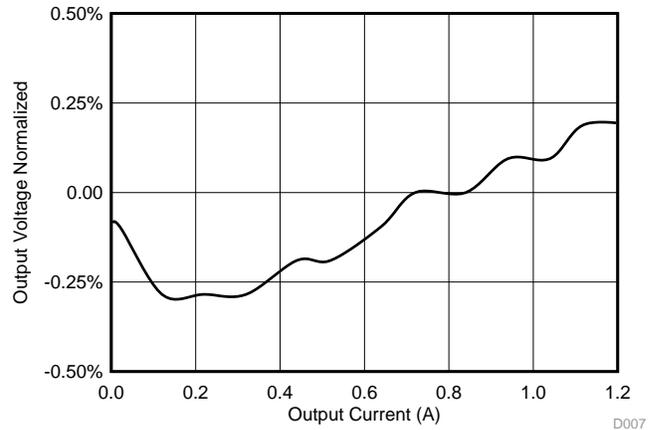
Figure 33. VEVE Load Regulation 0 to 1.2 A (V<sub>IN</sub> = 3.3 V)
