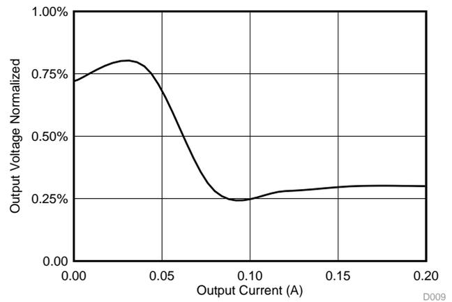
Figure 35. VCAN Load Regulation 0 to 0.2 A (V<sub>IN</sub> = 3.3 V)
