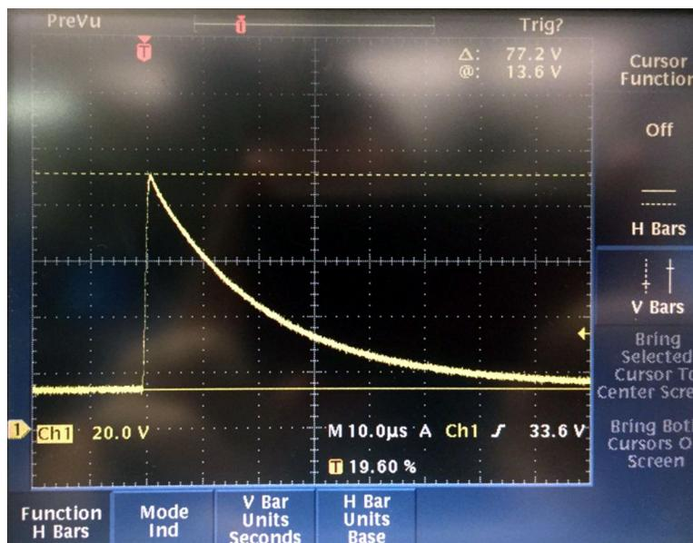
Figure 67. Pulse 2a Test Pulse
