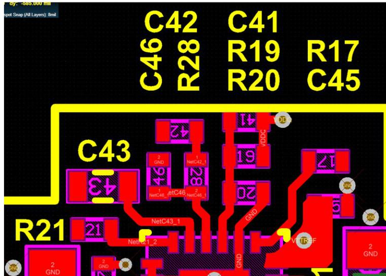
Figure 73. Compensation and Feedback Components Placed Close to IC
