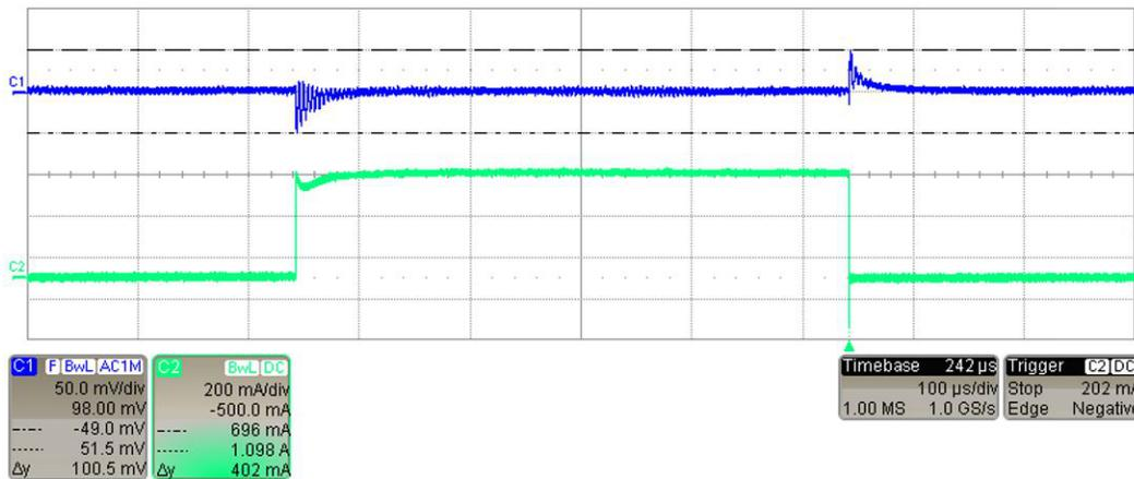
Figure 46. V3P3, VOUT = 3.3 V, IOUT\_STEP = 500 mA
