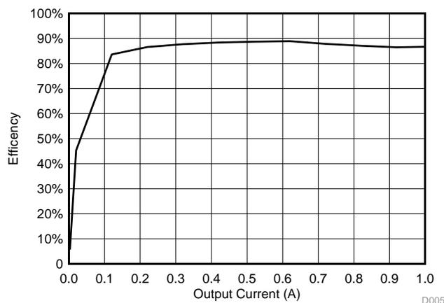
Figure 31. VDDQ Efficiency ( $V_{IN} = 3.3\text{ V}$ )
