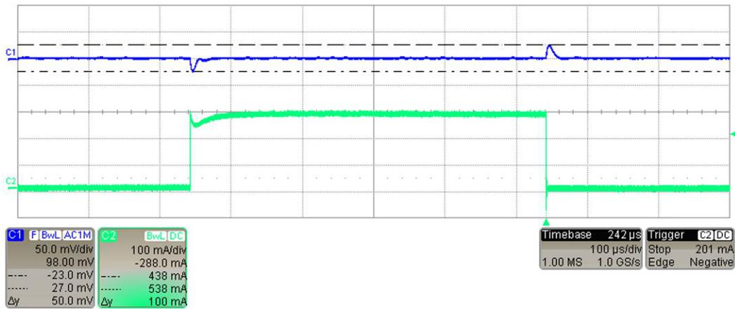
Figure 47. V\_EVE, VOUT = 1.06 V, IOU\_STEP = 300 mA
