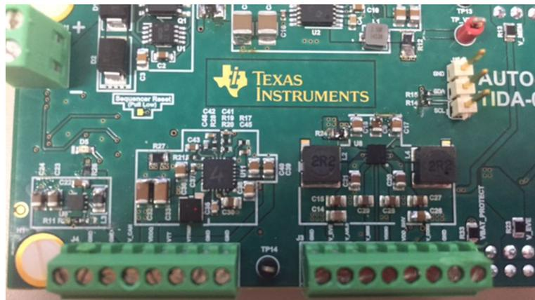
**Figure 15. Screw Terminals for Supply Outputs**
