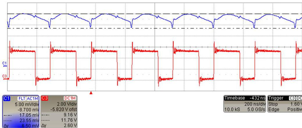
Figure 45. V\_CAN, VOUT = 5V, IOUT = 200mA
