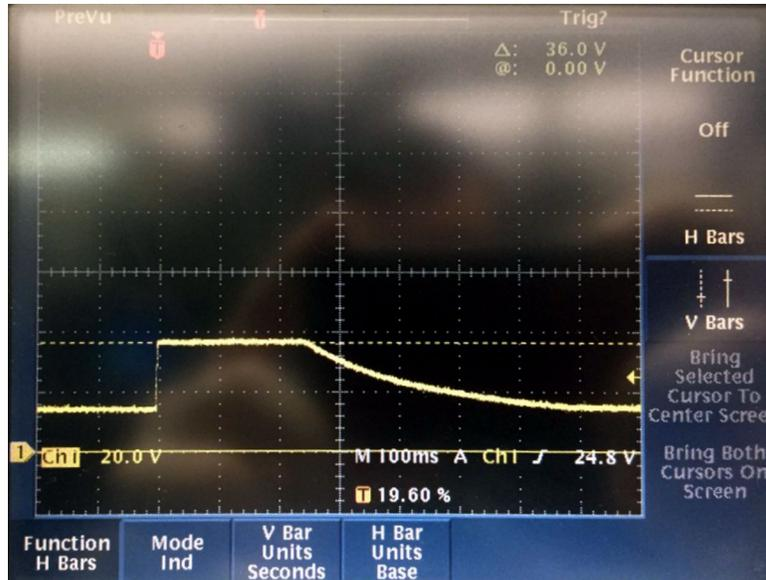
Figure 70. Pulse 5b (Clamped Load Dump) Test Pulse
