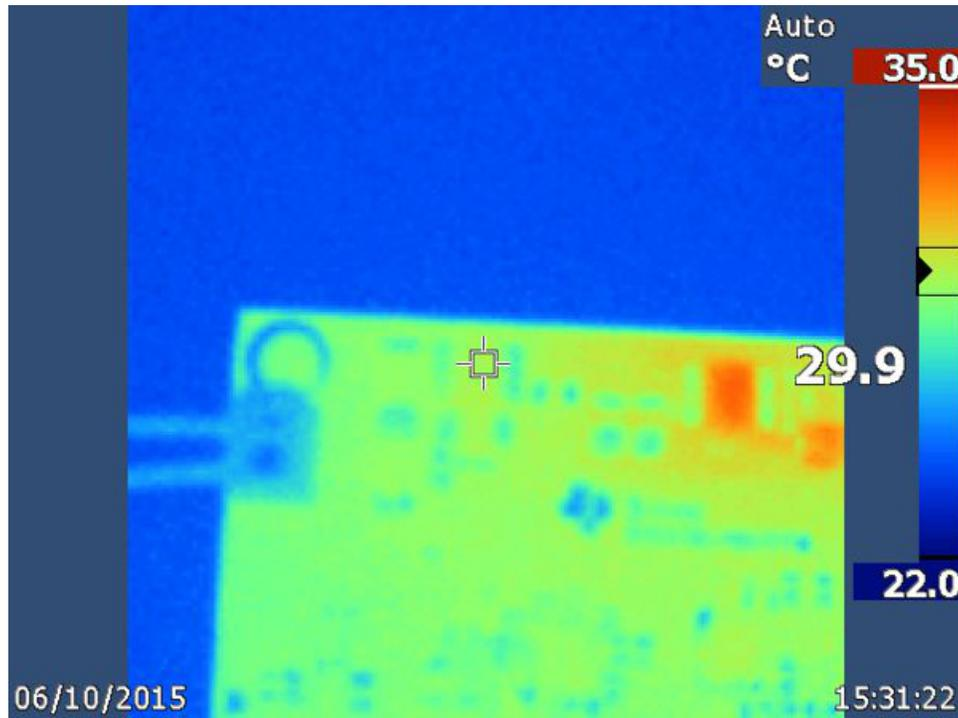
Figure 51. LM74610 (Reverse Polarity Protection) FET, No Load, Steady State
