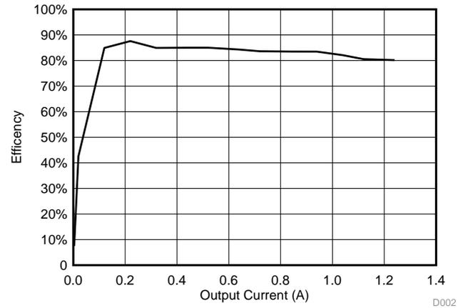
Figure 28. VEE Efficiency ( $V_{IN} = 3.3\text{ V}$ )
