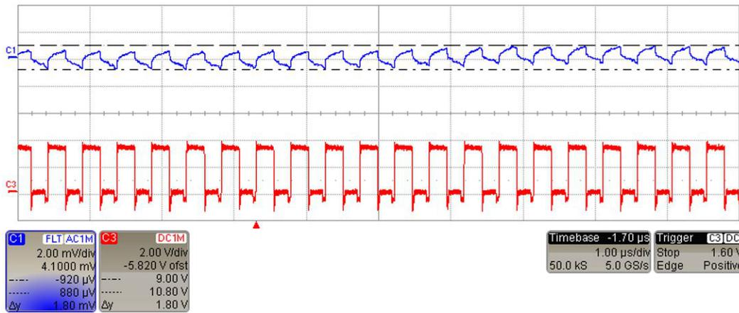
Figure 44. VDDQ, VOUT = 1.5V, IOUT = 1A
