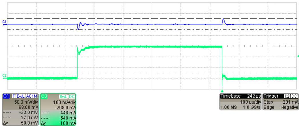
Figure 48. V\_CORE, VOUT = 1.06 V, IOU\_STEP = 300 mA
