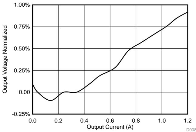
Figure 34. VCORE Load Regulation 0 to 1.2 A (V<sub>IN</sub> = 3.3 V)
