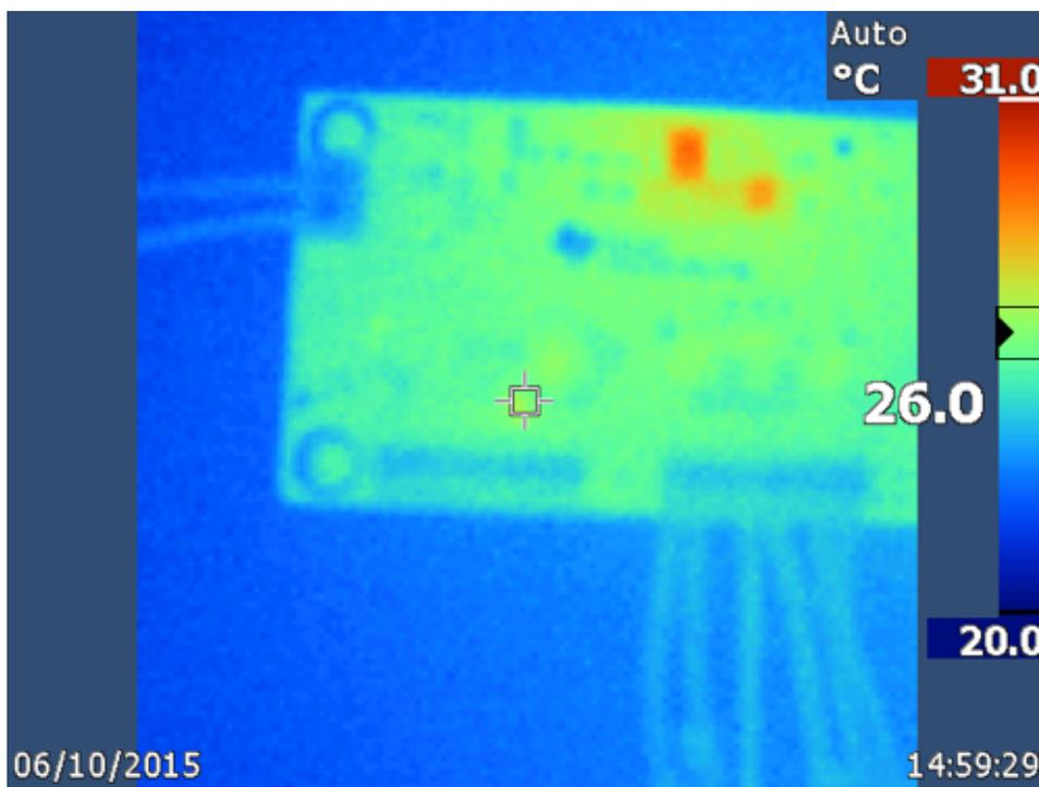
Figure 58. TPS54116-Q1 IC, No Load, Steady State
