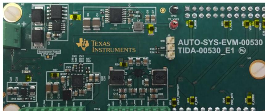
**Figure 16. 0- $\Omega$  Resistors for Isolating Supplies**
