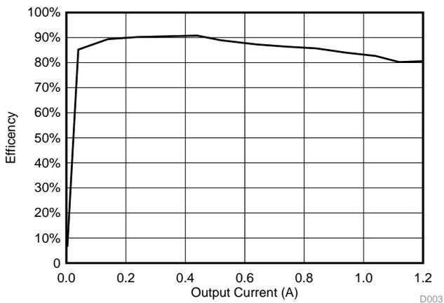
Figure 29. VCORE Efficiency ( $V_{IN} = 3.3\text{ V}$ )
