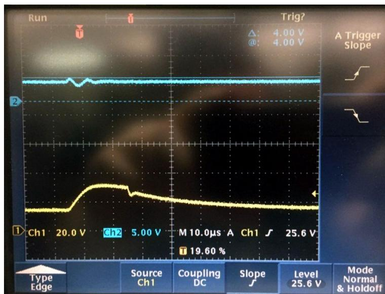
Figure 69. Max Overshoot = 4 V Protects Circuits Downstream
