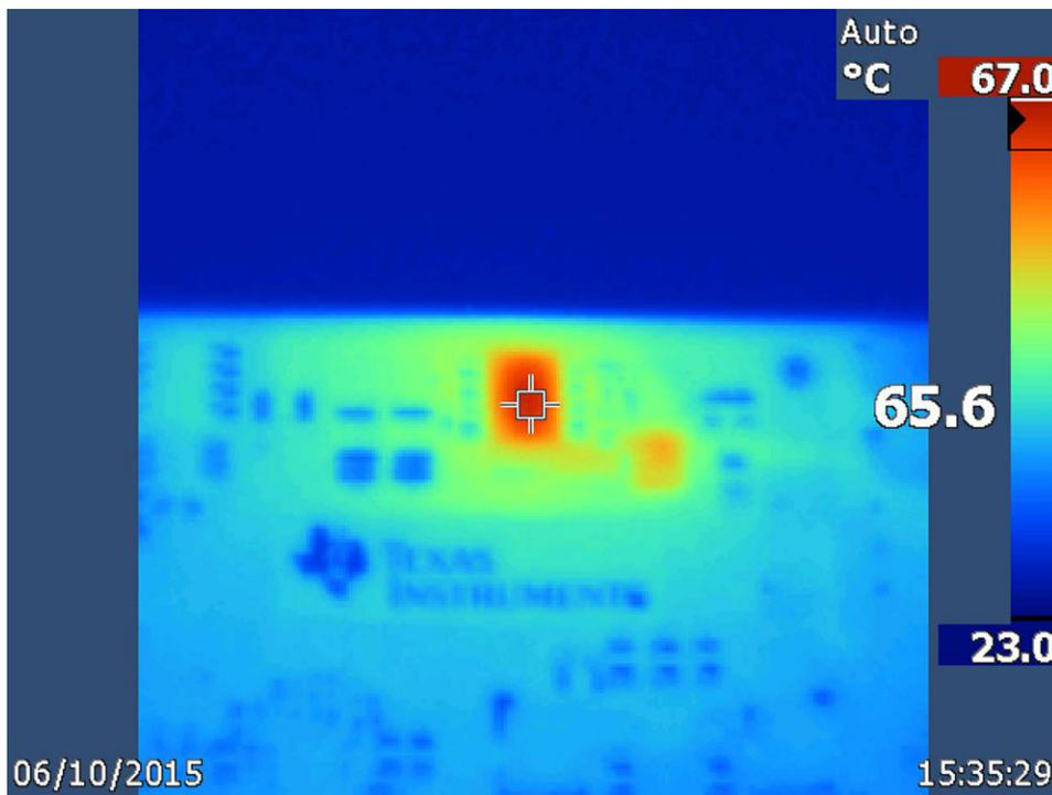
Figure 54. LM53603 (Wide-VIN Buck) IC, Full Load, Steady State
