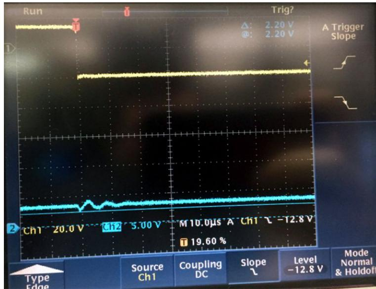
Figure 66. Max Undershoot = 2.2 V may be too low for some downstream converters to maintain regulation. Additional hold-up capacitors can be added to those converter inputs in this case.
