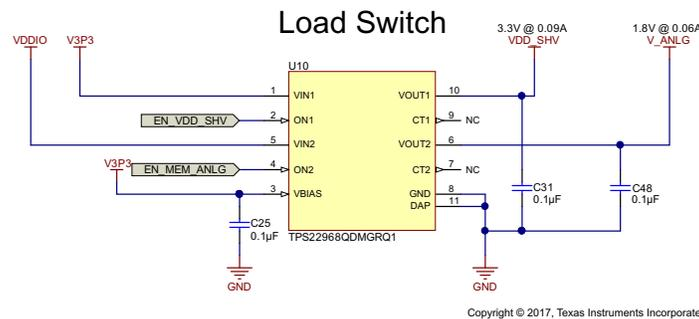
**Figure 10. Load Switch Schematic**
