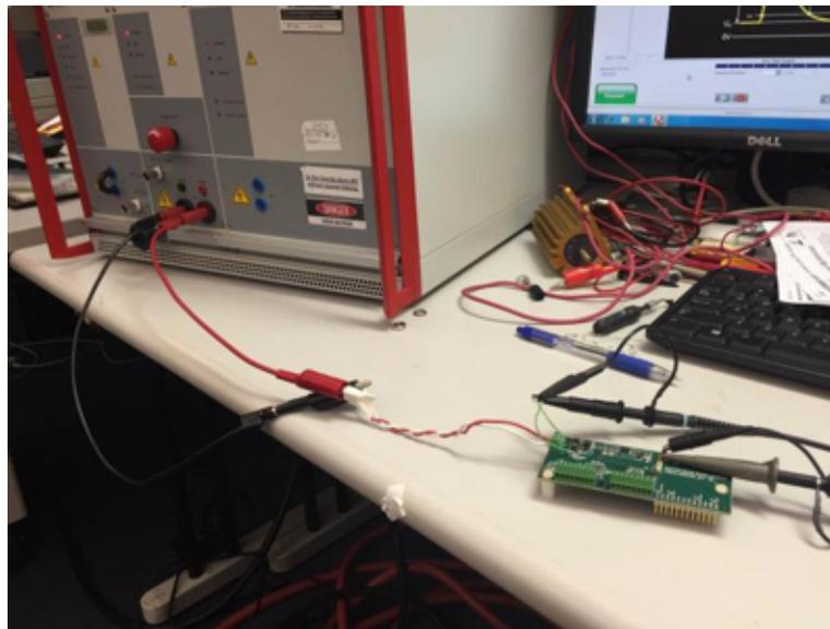
**Figure 25. Picture of Setup for Transient Tests**
