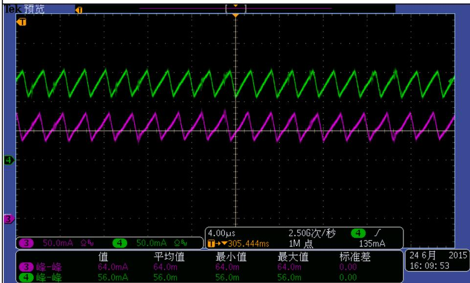
Vin:230Vac Io: LED Lamp load
