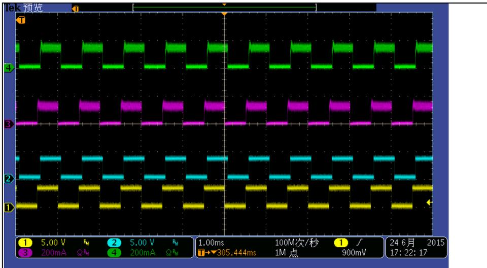
Vin:110Vac Io: LED Lamp load
