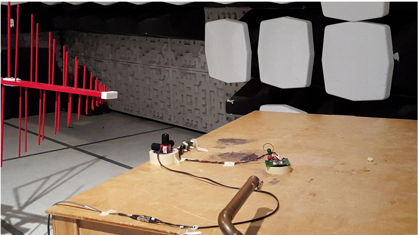
**Figure 21. RF Immunity Test Setup**
