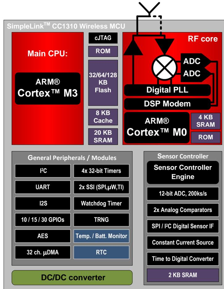
Figure 3. CC1310 Functional Block Diagram
