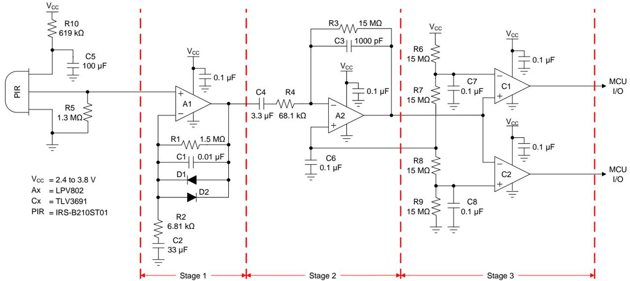
Figure 5. PIR Motion Sensor Analog Signal Path Schematic
