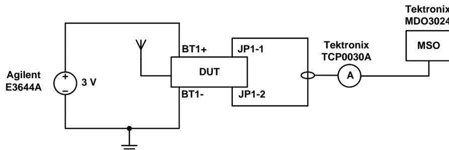
**Figure 18. Test Circuit Used for Measuring Supply Current During Radio Transmission Intervals**
