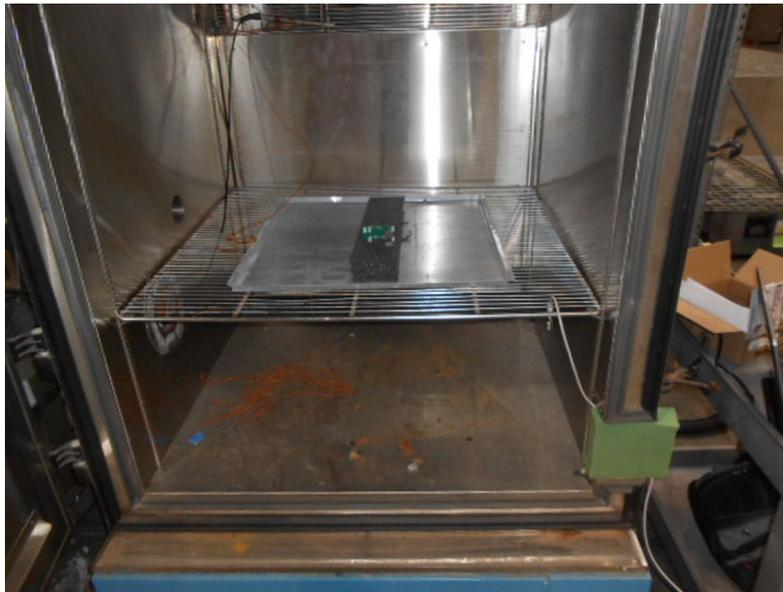
**Figure 19. Wireless PIR Motion Detector Temperature and Humidity Test Setup**
