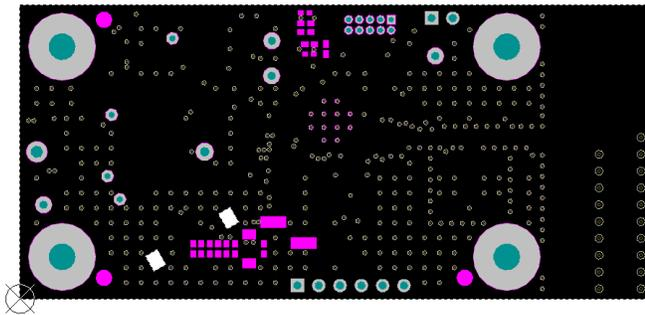
Figure 32. Bottom Solder Mask
