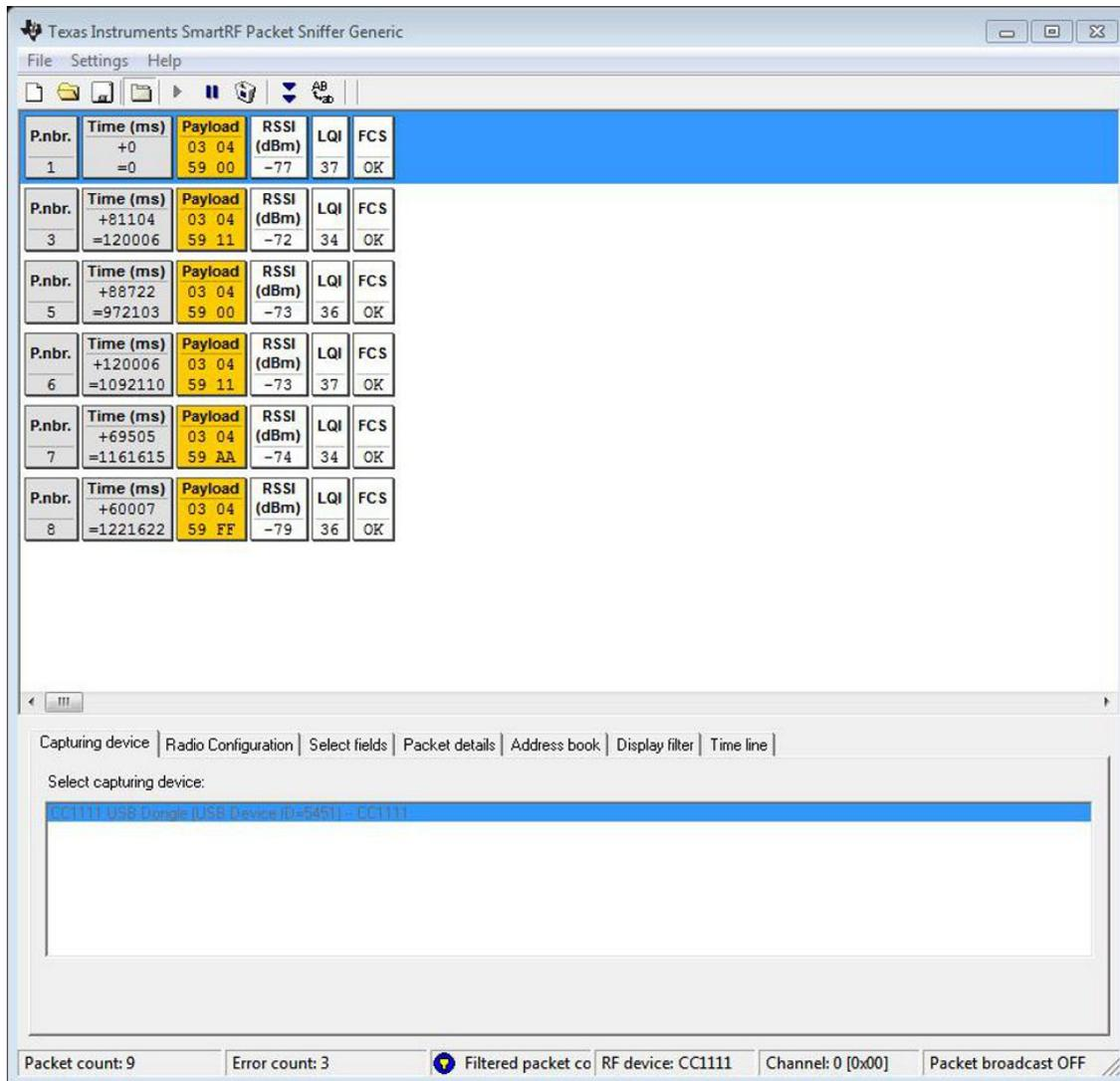
Figure 16. Packet Sniffer Software, Filtered Recording
