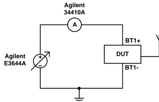
**Figure 17. Test Circuit Used for Measuring Supply Current**
