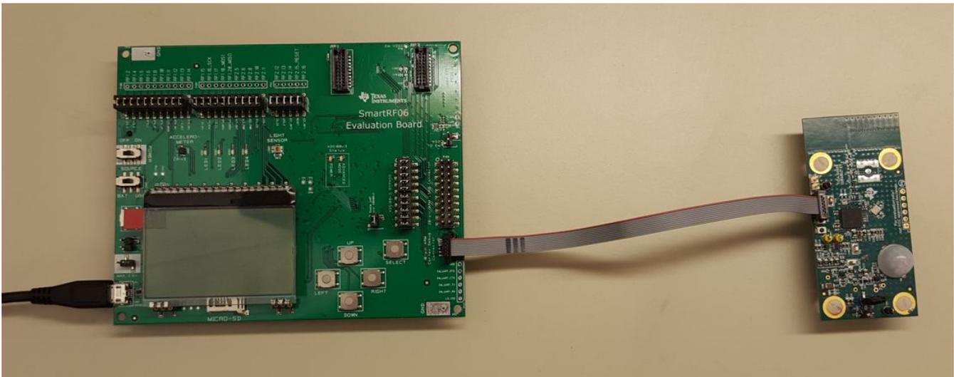
**Figure 11. Connection of SmartRF06 Evaluation Board and TI Designs Hardware for Programming and Debugging**
