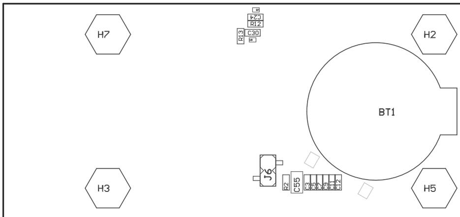
**Figure 38. Bottom Assembly Drawing**
