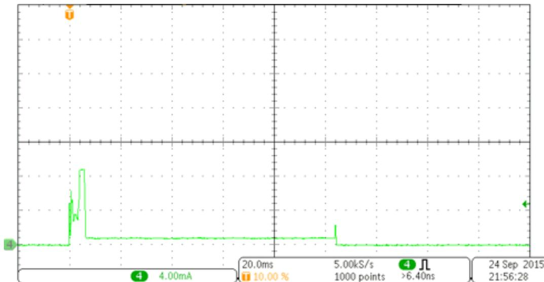
**Figure 23. Radio Transmission Event Supply Current (Full Picture)**
