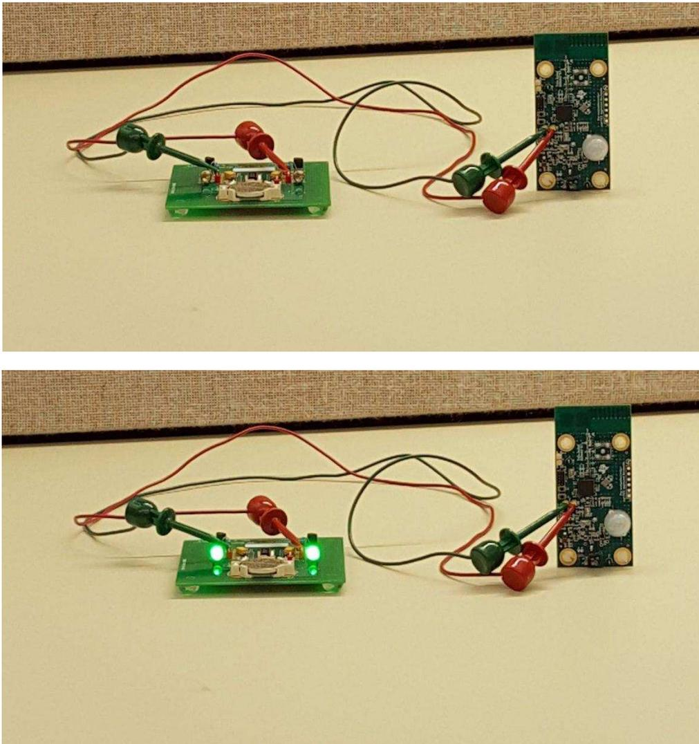
**Figure 20. Motion Sensitivity Test Setup
