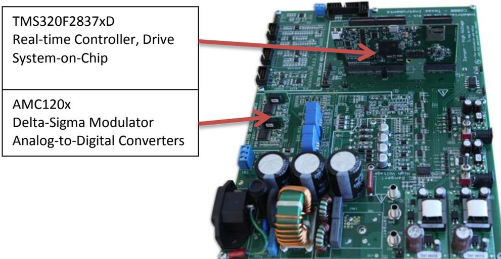
**Figure 2 DesignDRIVE IDDK Reference Design**
