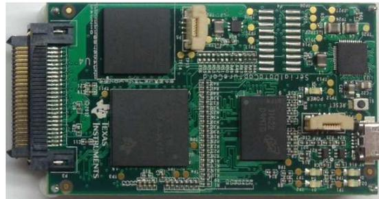
Figure 16. SDCC Card of ADSxx54 Board
