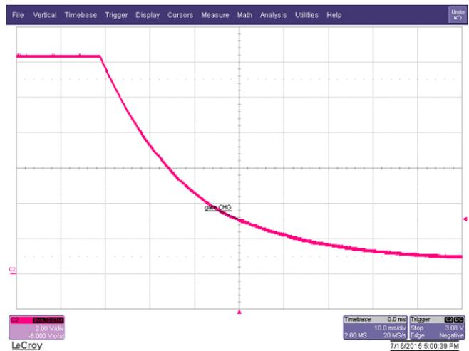
Figure 17. Gate Voltage of CHG FETs While Opening
