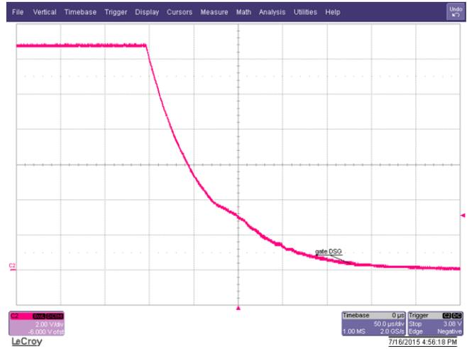
Figure 15. Gate Voltage of DSG FETs While Opening
