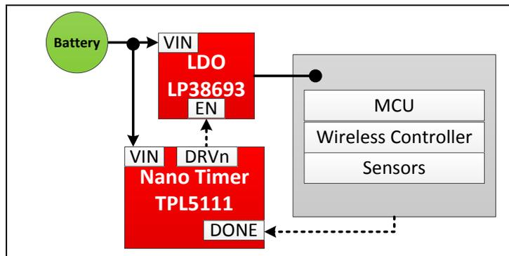
Figure 2 TIDA-00720 High Level Block Diagram
