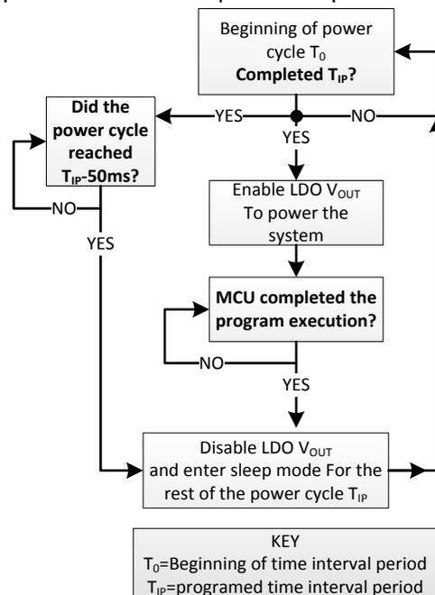
**Figure 1 Power Cycle Process**
