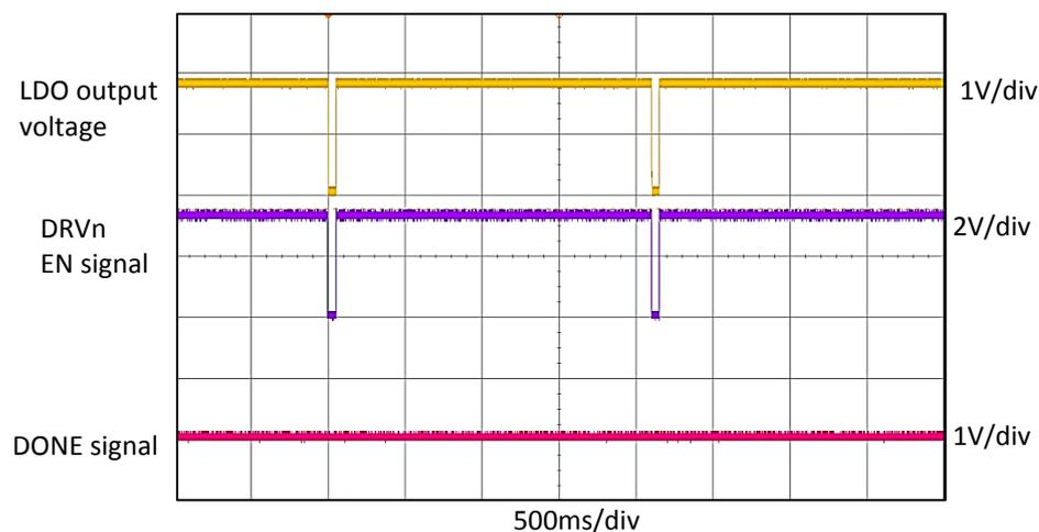
**Figure 7 DONE Signal Not Received Within Programed Time Interval**
