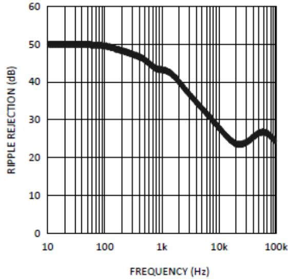
Figure 11: Comparison between PSRR and Frequency
