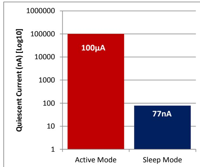
**Figure 5: Comparison between Sleep Mode and Active Mode (no load)**
