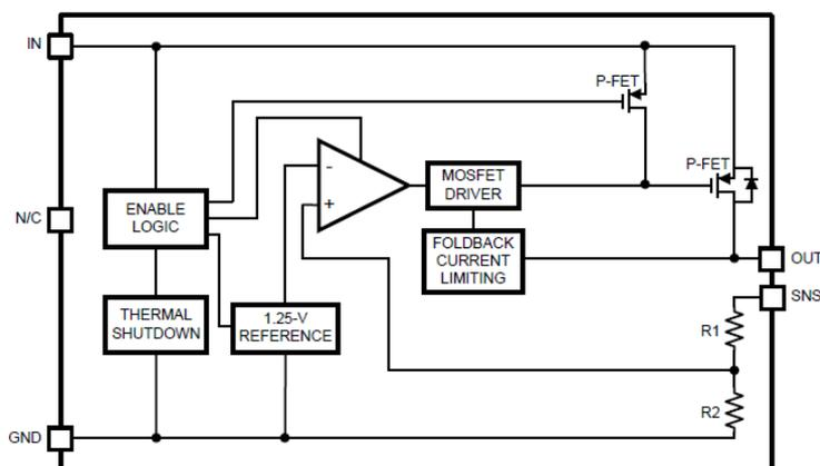
Figure 3 LP38693 Functional Block Diagram
