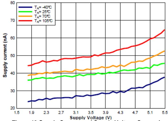
Figure 13 Supply Current and Supply Voltage Comparison
