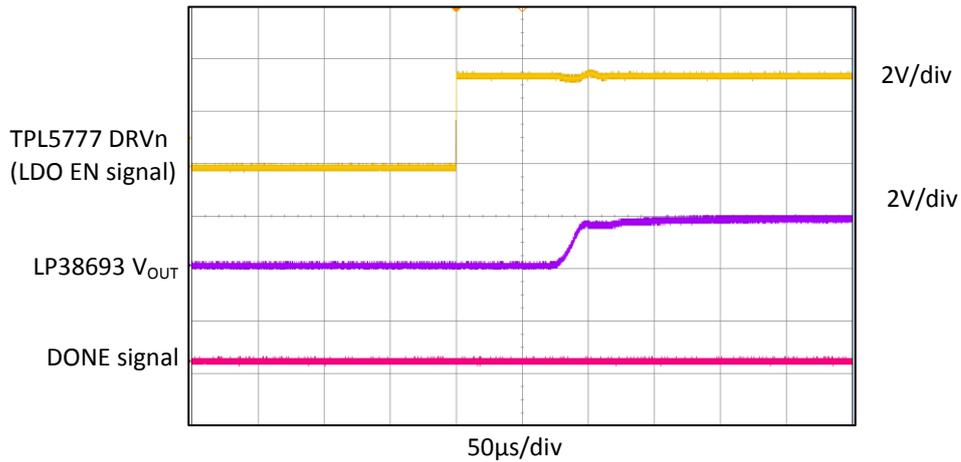
Figure 8 TPL38693 Output Voltage Power-up Time
