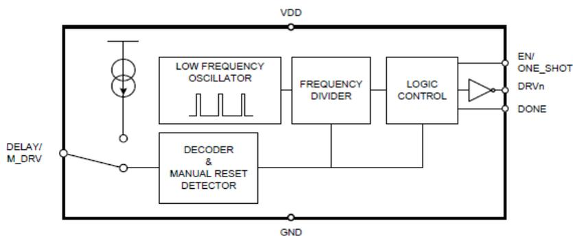
**Figure 4: TPL5111 Functional Block Diagram**
