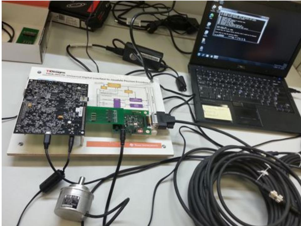
Figure 47. Setup for TIDA-00179 Test With HEIDENHAIN EnDat 2.2 Encoders
