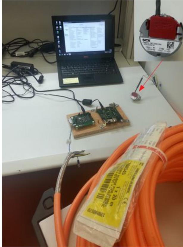
**Figure 49. Setup for TIDA-00179 Test With 2-Wire HIPERFACE DSL Encoder**
