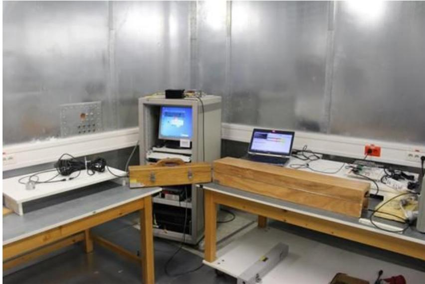
**Figure 60. EFT Test Setup for TIDA-00179**
