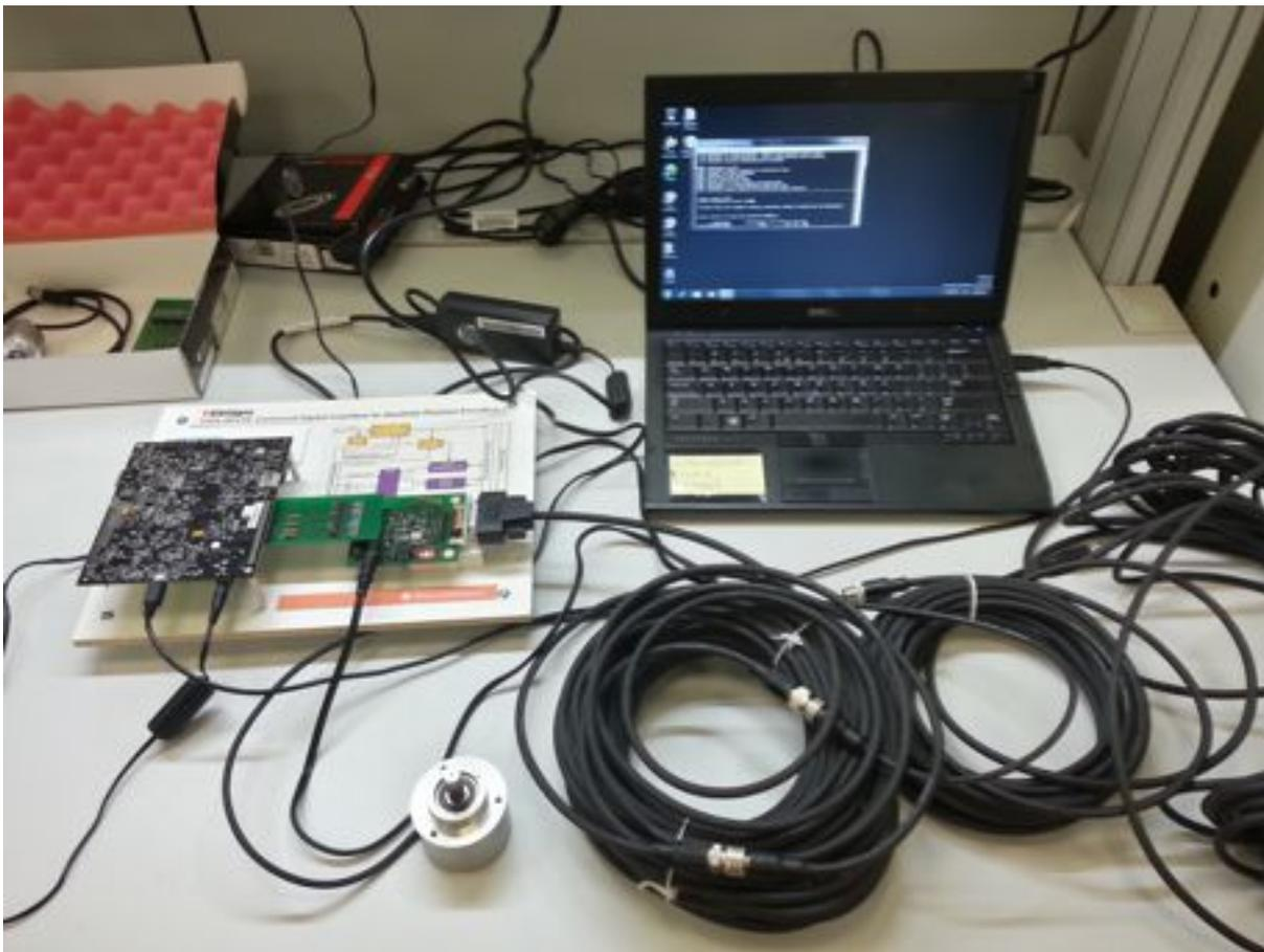
**Figure 21. Picture of Test Setup for TIDA-00179 RS-485 Performance Tests**
