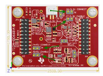
J5 is the enable pin for the 3.3V Regulator. Remove this jumper and the 3.3V Regulator will not start up.
