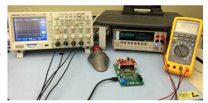
The use of a precision multi-meter along with a 1 Ohm shunt will make a great current measuring solution. Set the meter to the DC milli-volt scale and read the current as milli and micro Amps. Example: 1mV = 1mA
