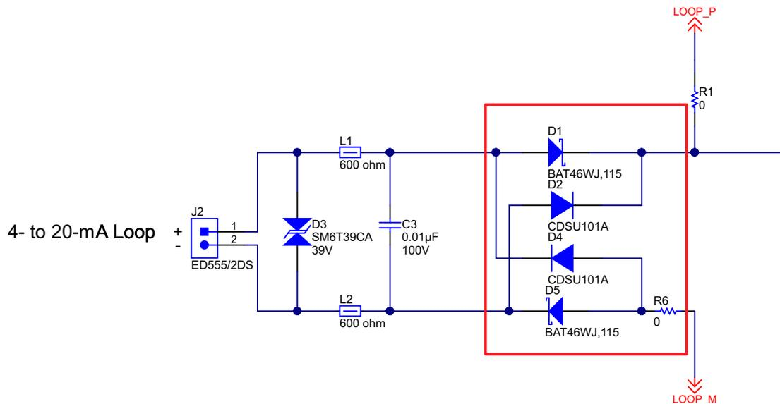
**Figure 11. Input Reverse Protection**
