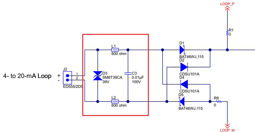
Figure 10. Input Overvoltage Protection
