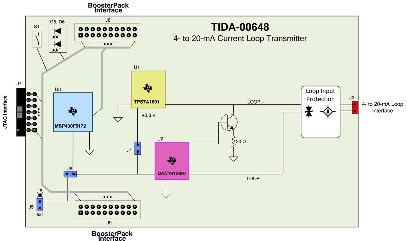
Figure 1. TIDA-00648 System Block Diagram
