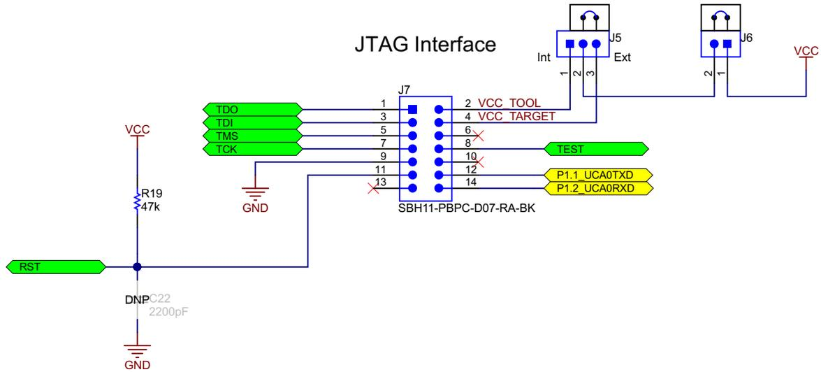
Figure 16. JTAG Interface and UART Backchannel
