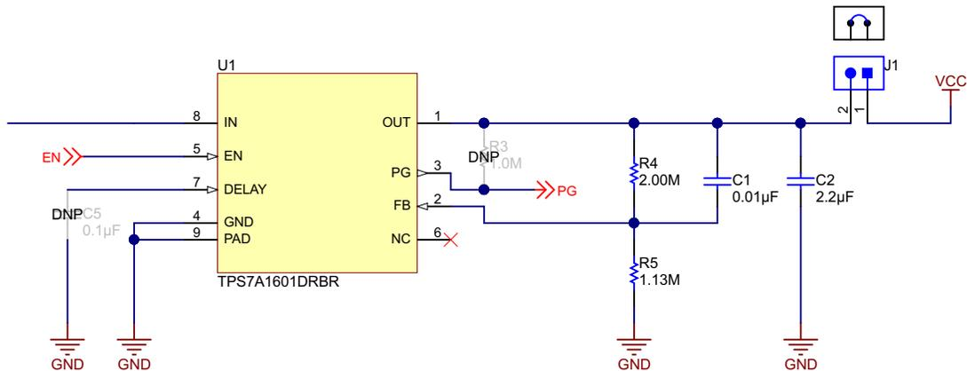
**Figure 9. LDO Circuit With Feedback for Adjustable Output**
