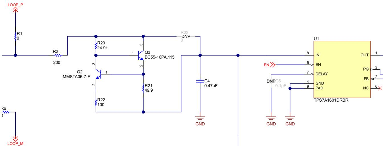
Figure 12. Current Limiter and Sense Resistor Protection
