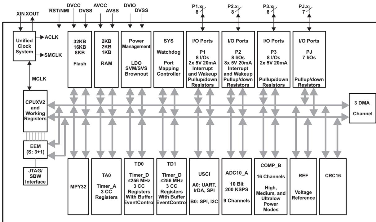
**Figure 5. MSP430F51x2 Block Diagram**
