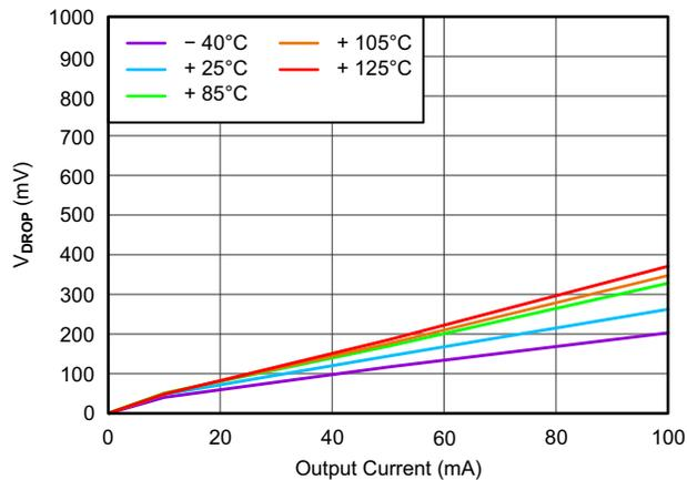
**Figure 4. Dropout Voltage Versus Output Current**
