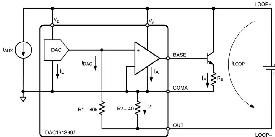
Figure 7. Loop-Powered Transmitter
