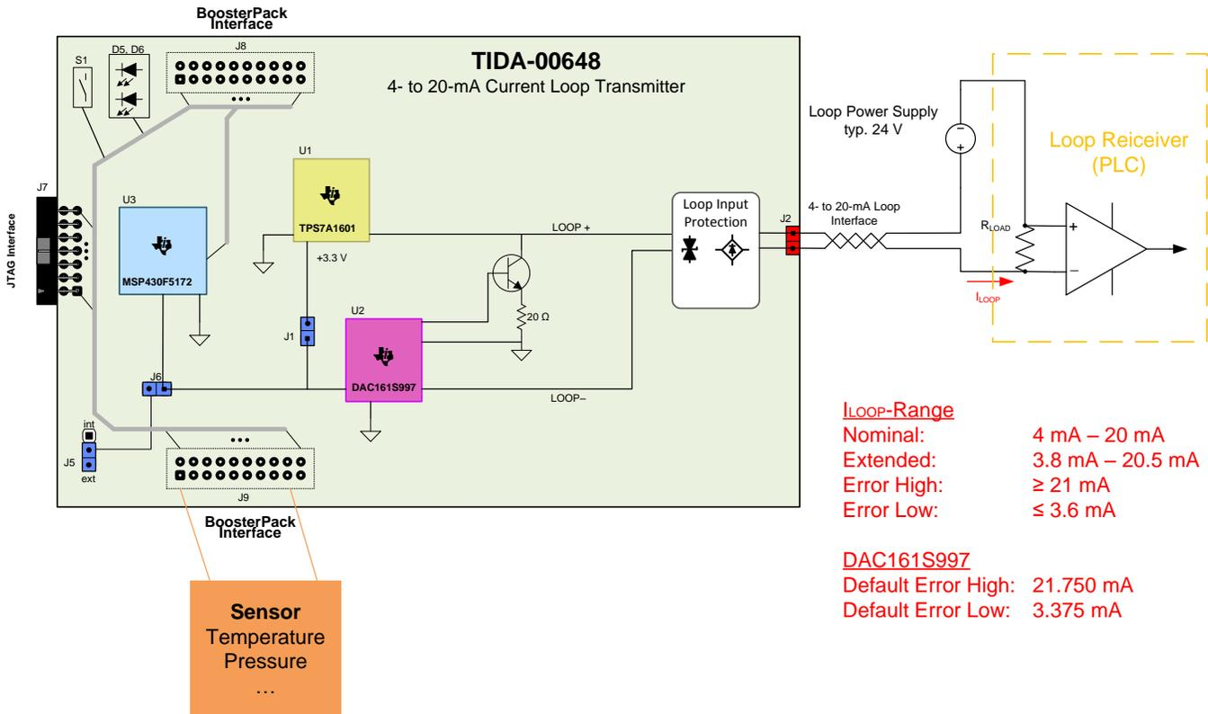
Figure 6. Typical Current-Loop System
