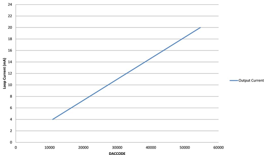
**Figure 18. 4- to 20-mA Current Loop**
