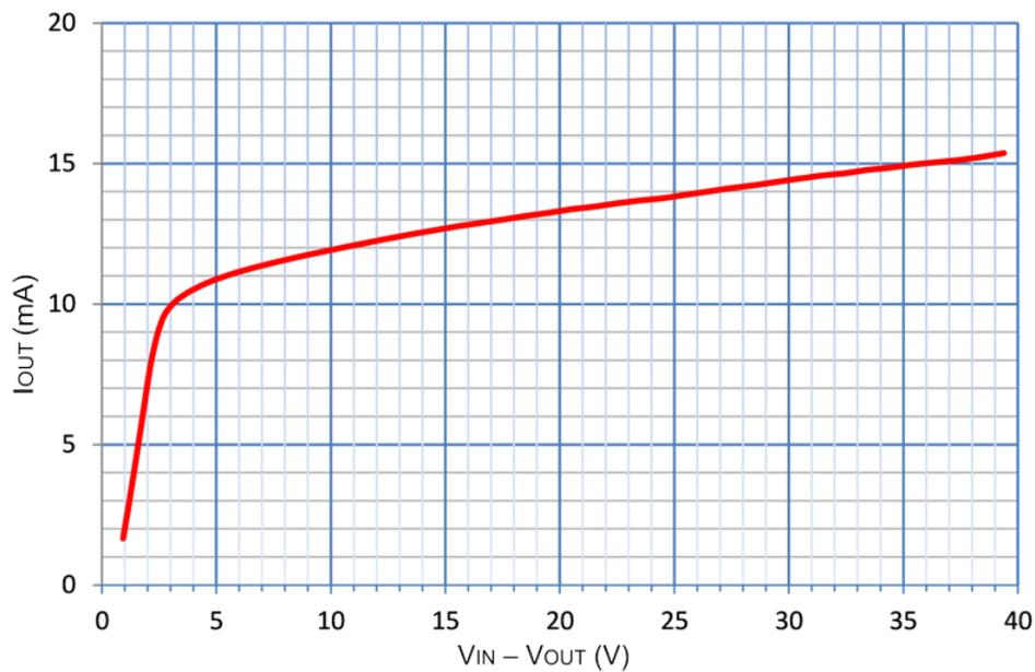
Figure 14. Active Current Limiter Characteristic— $I_{OUT}$  Versus  $V_{IN} - V_{OUT}$
