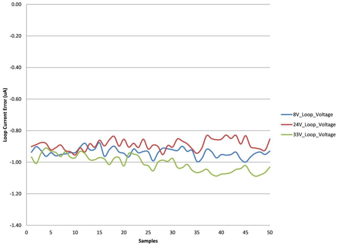
**Figure 19. Loop Voltage Influence and DAC Noise Error**
