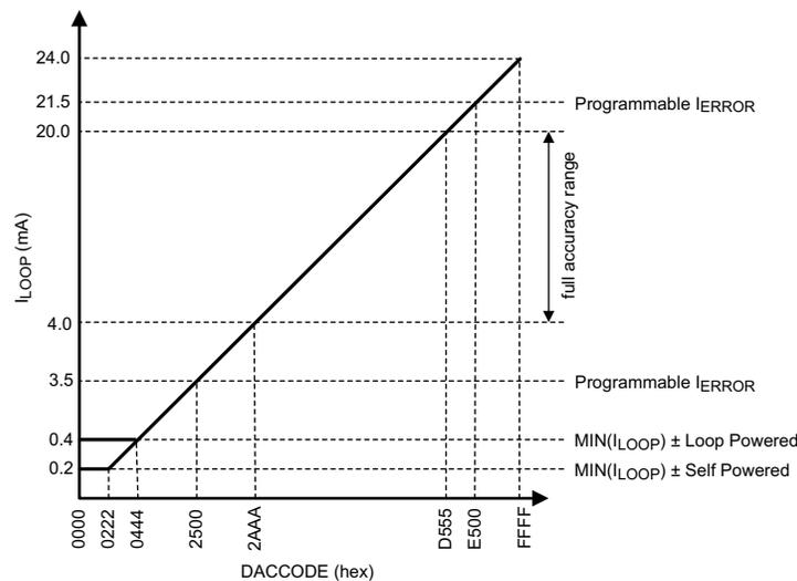
Figure 8. DAC-DC Transfer Function
