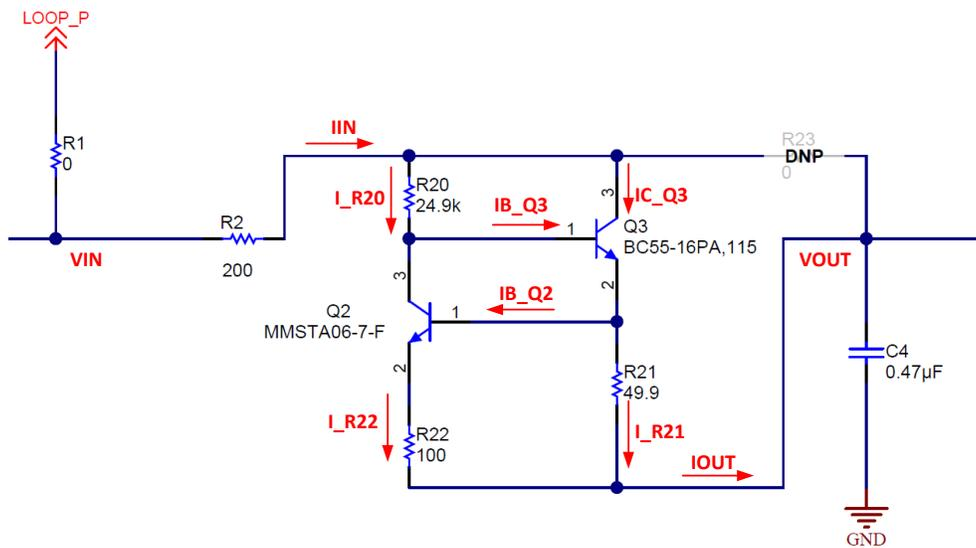
Figure 13. Active Current Limiter—Schematics and Operation
