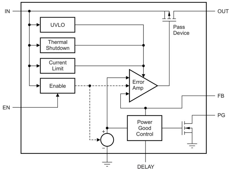
**Figure 3. TPS7A1601 Block Diagram**
