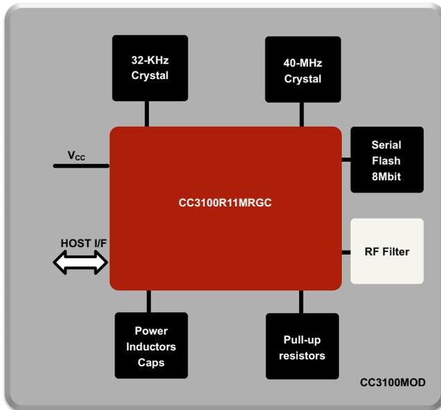
Figure 3. CC3100MOD Functional Block Diagram
