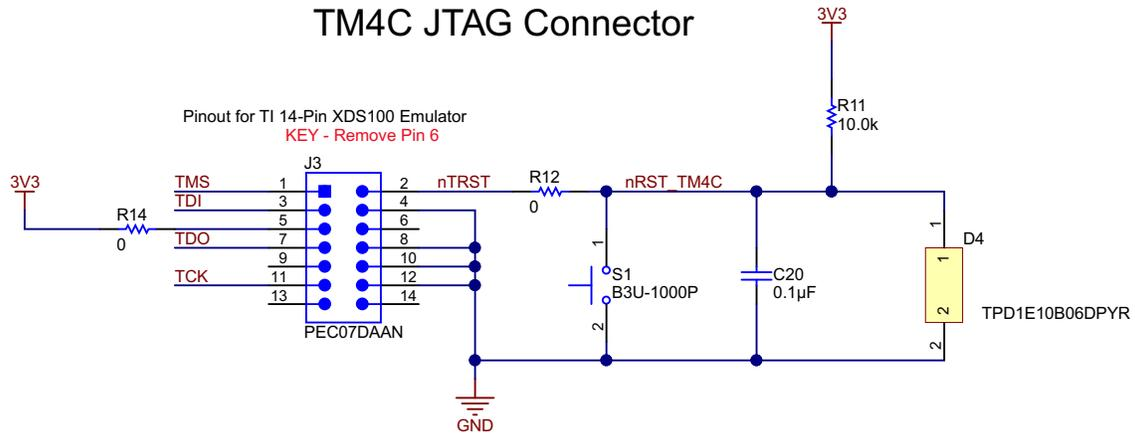
Figure 13. TM4C123GH6PM JTAG Connector Schematic
