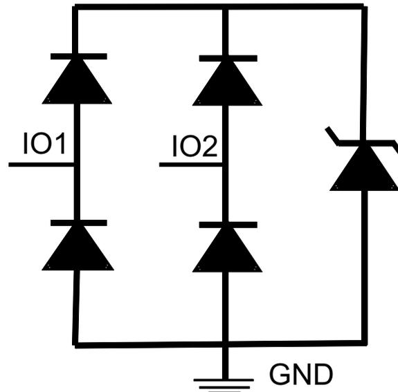
Figure 9. TPD2E2U06 Functional Block Diagram
