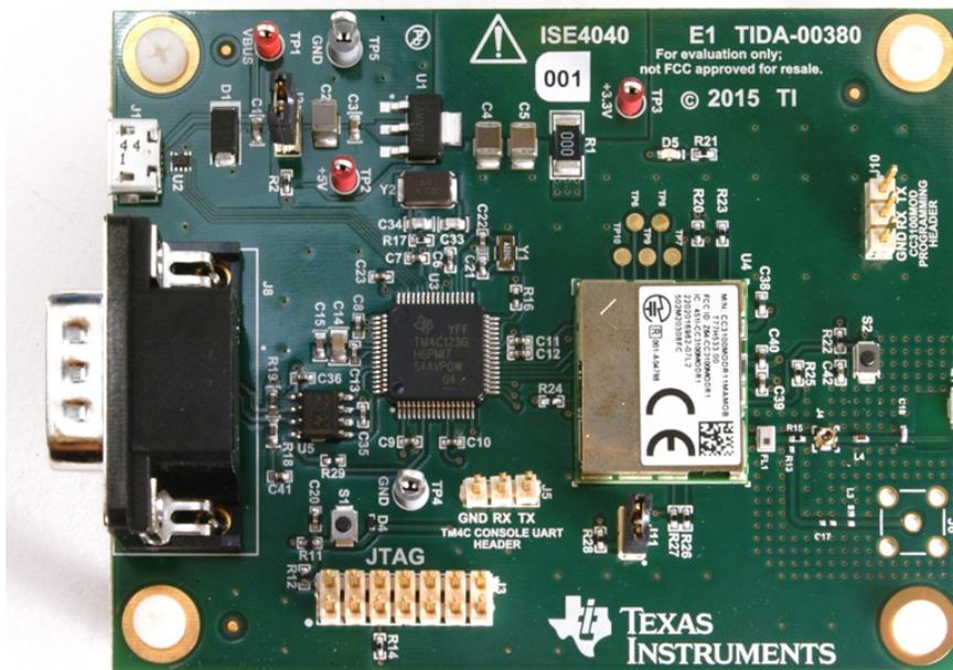
**Figure 1. CAN to Wi-Fi® Gateway**
