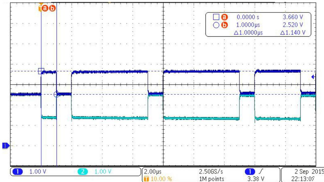
Figure 35. CAN SOF Timing Measurement Plus CANH Level During Transmit
