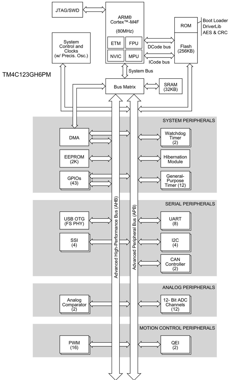
Figure 5. TM4C123GH6PM High-Level Block Diagram
