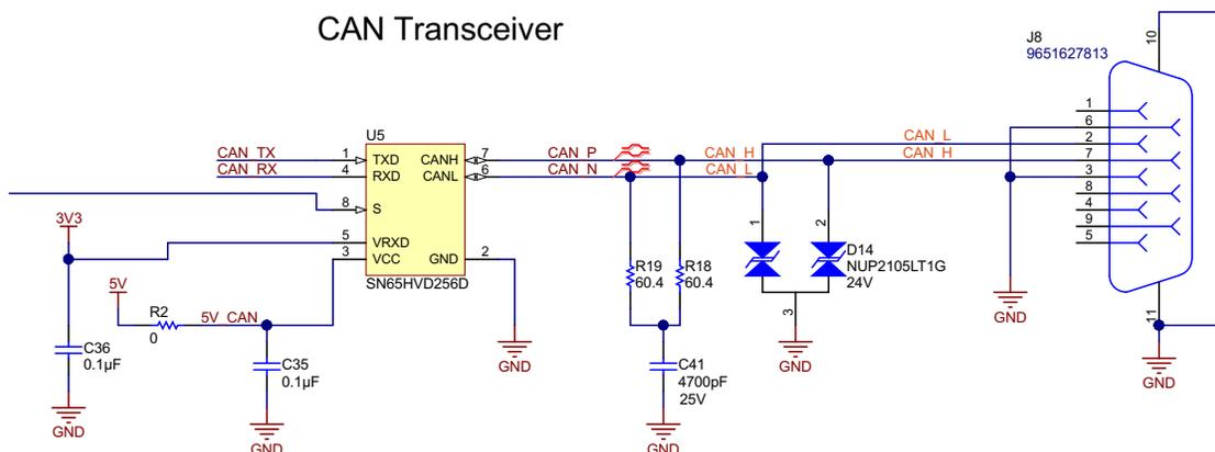
Figure 11. CAN Transceiver Schematic
