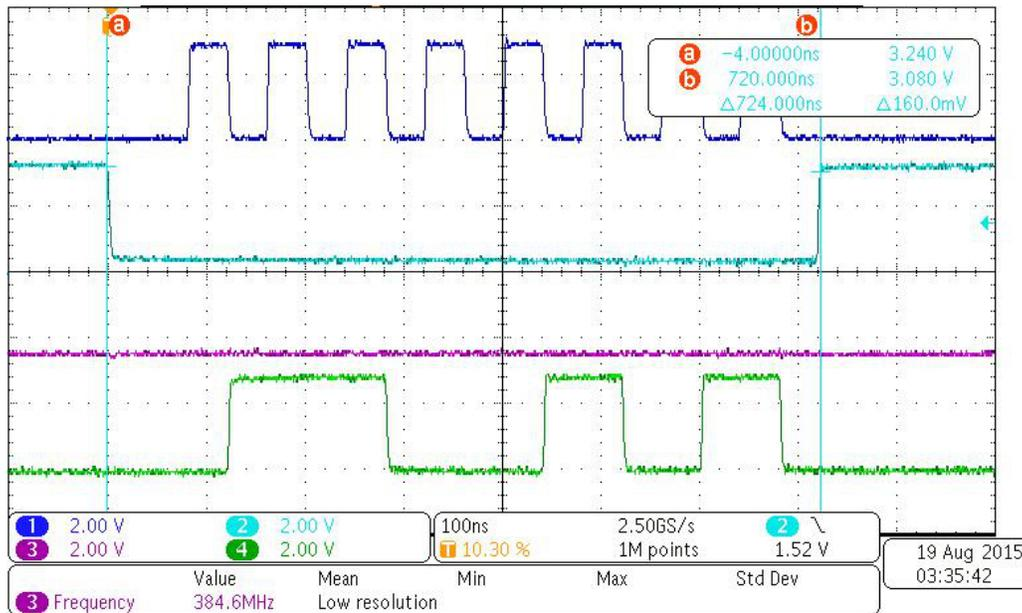
Figure 33. SPI Chip Select (CS) Period
