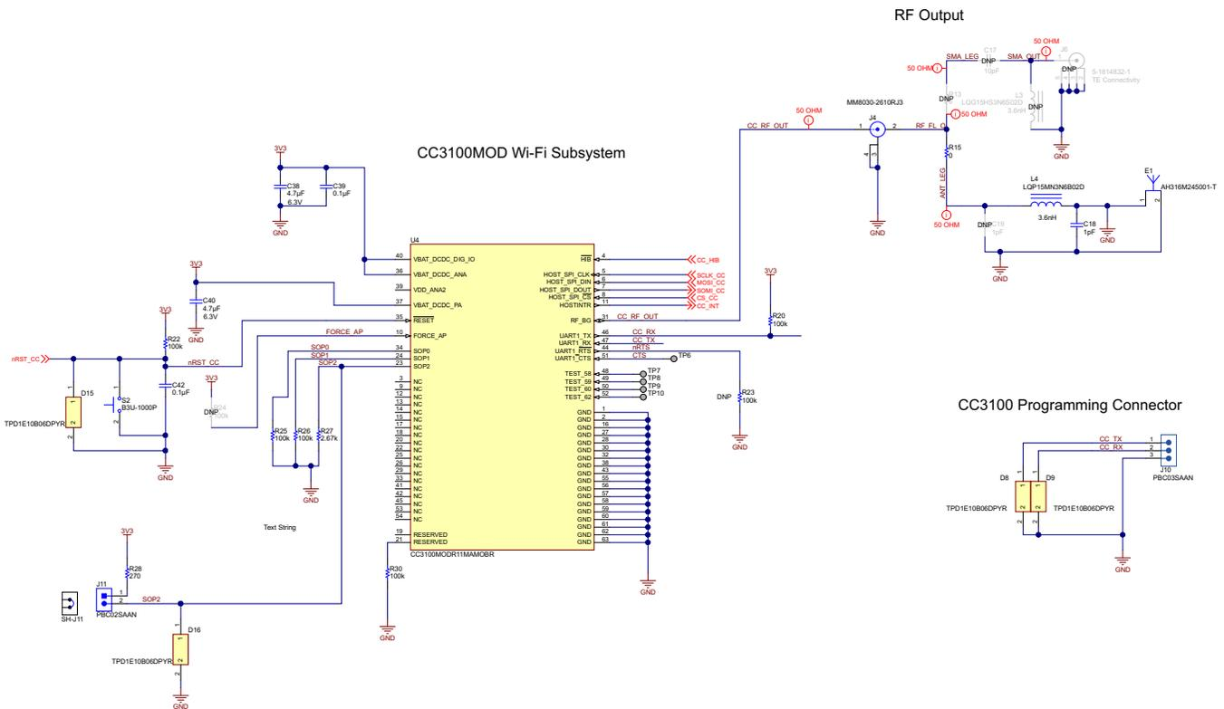
Figure 15. CC3100MOD Schematic
