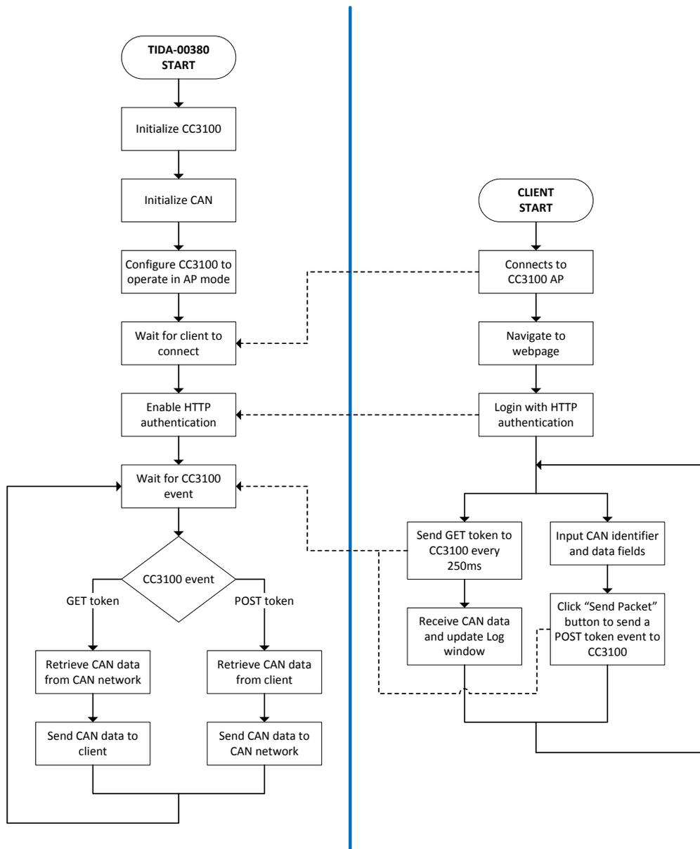
Figure 17. Application Software Flow Diagram
