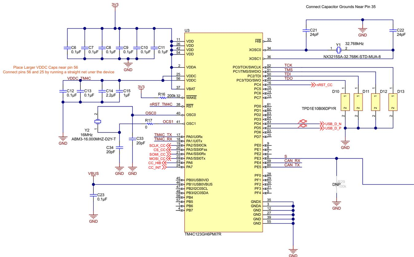
Figure 12. TM4C123GH6PM Microcontroller Schematic
