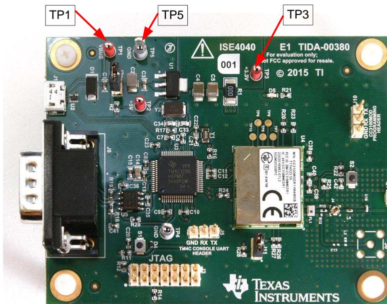
Figure 29. Locations of Test Points Used During Power Tests
