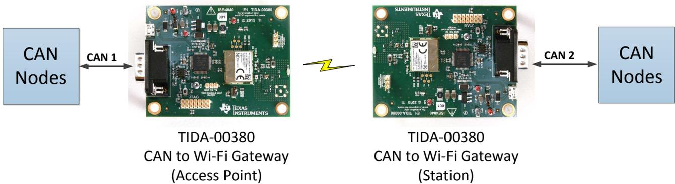
**Figure 37. CAN-to-Wi-Fi® Gateway Configured as Cable Replacement**
