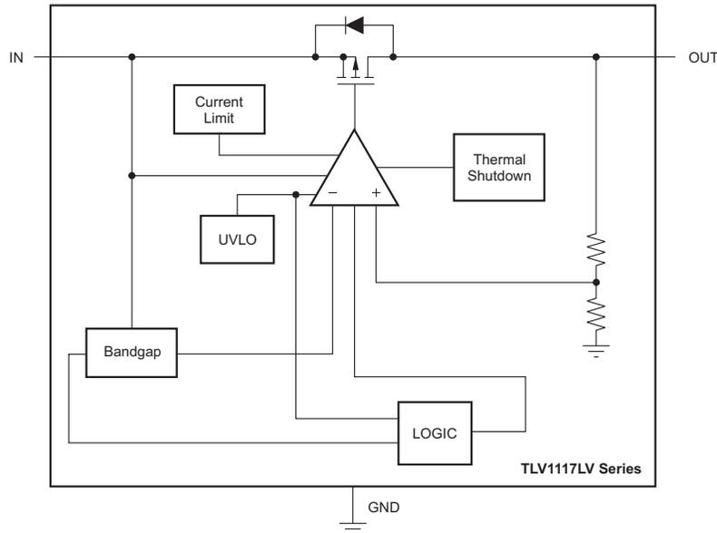
Figure 7. TLV1117LV33 Functional Block Diagram
