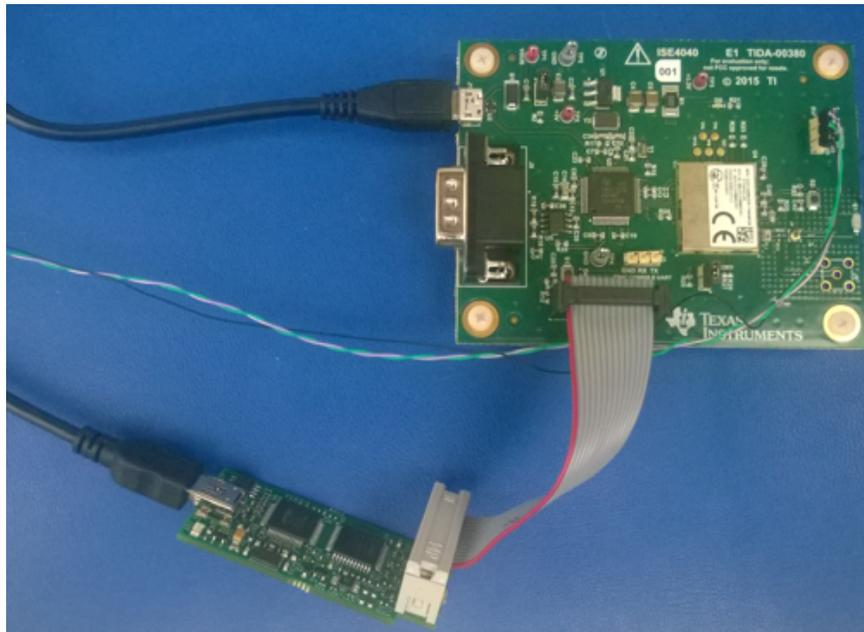
Figure 20. USB Cable for Power, XDS100v2, and UART-to-USB Connections for Programming
