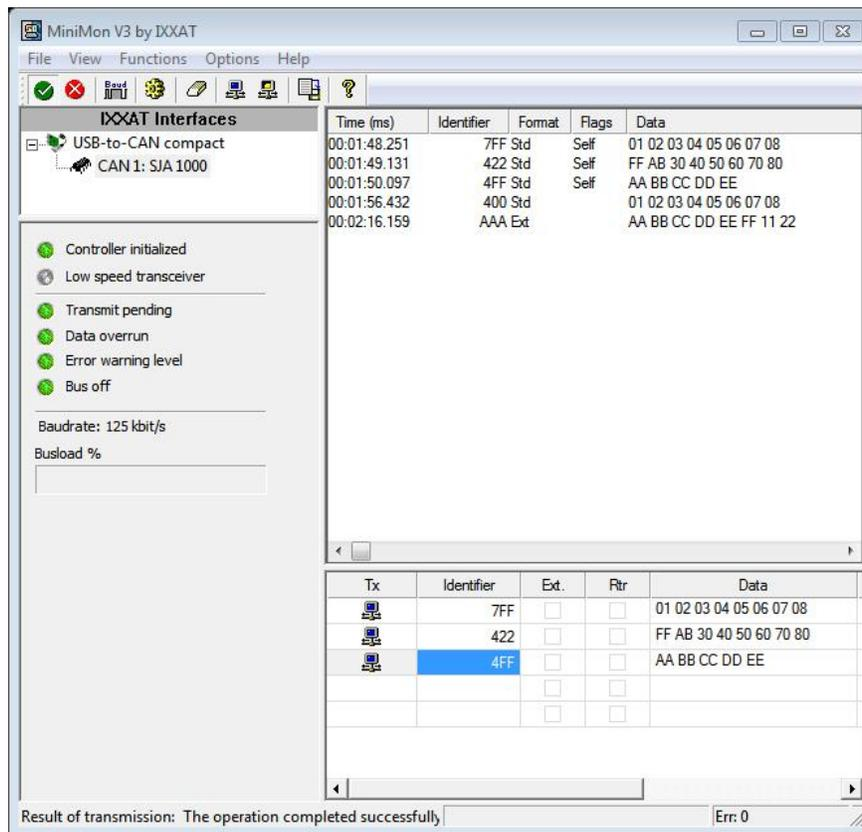
Figure 27. Example of CAN Sniffer Monitoring Software
