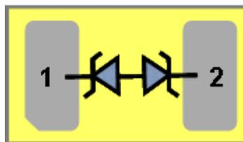
Figure 8. TPD1E10B06 Device Configuration
