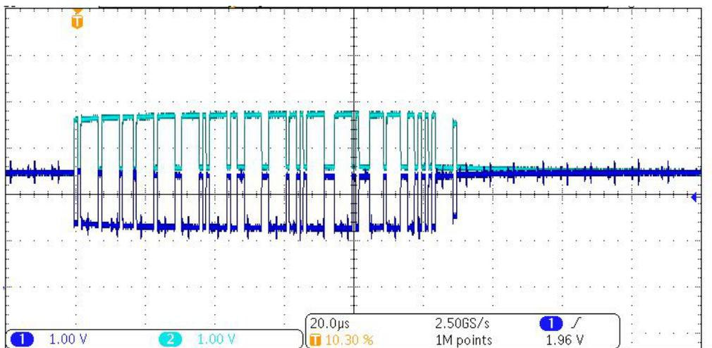
Figure 34. CAN Transmit from SN65HVD256
