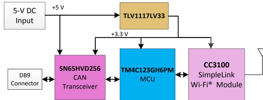
Figure 2. TIDA-00380 System Block Diagram
