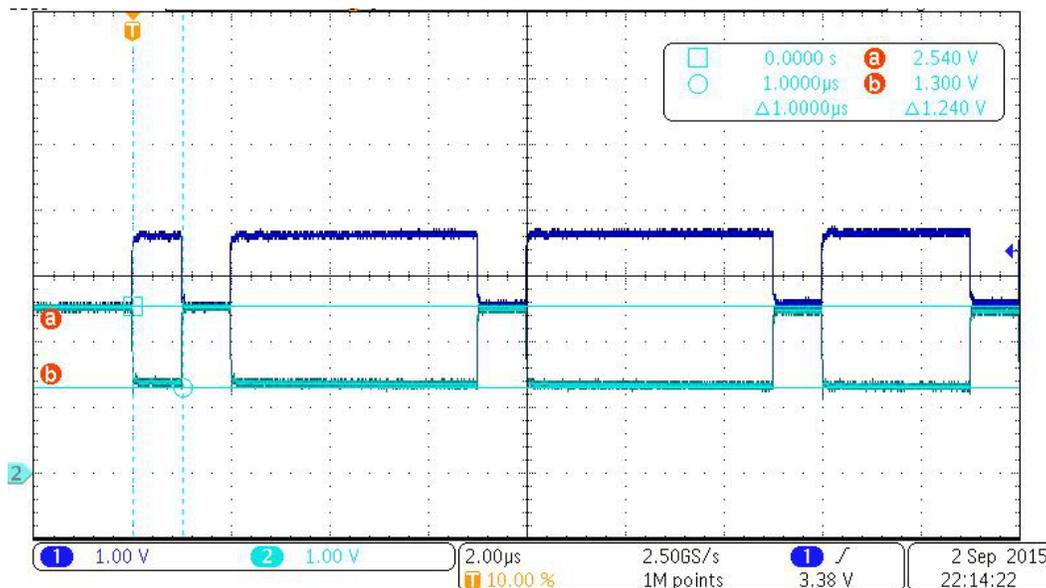
Figure 36. CANL Level During Transmit
