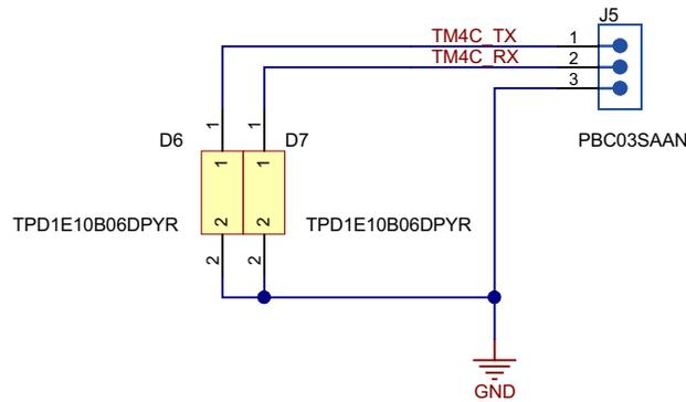
Figure 14. TM4C123GH6PM UART Terminal Connector Schematic
