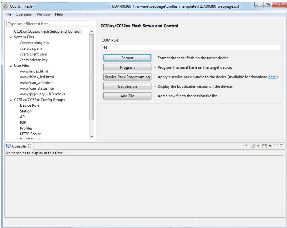
**Figure 21. CCS™ UniFlash Setup**
