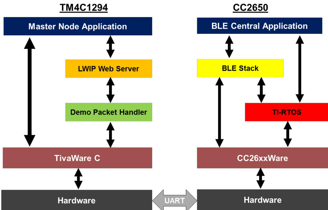
**Figure 6. TM4C BLE Central Architecture Block Diagram**
