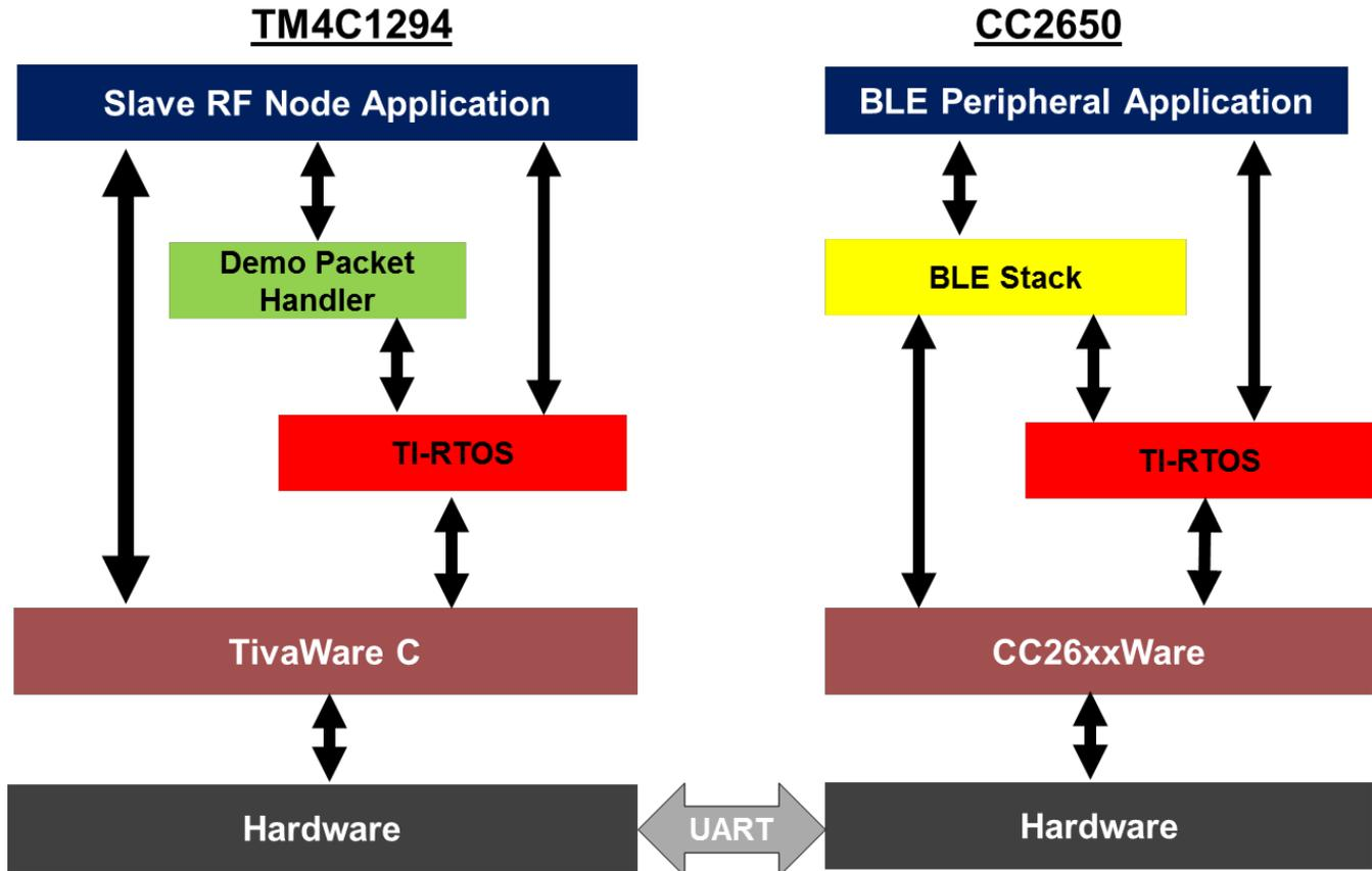
Figure 7. TM4C BLE Peripheral Architecture Block Diagram
