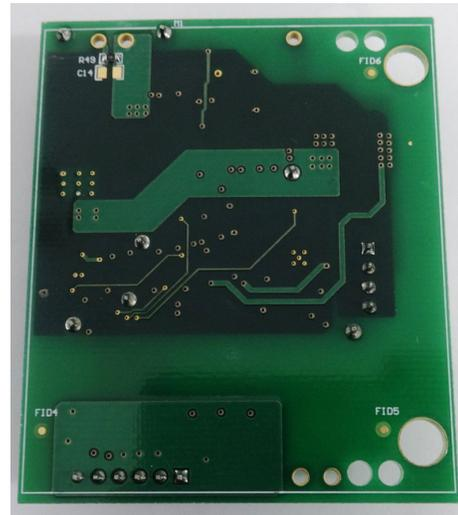
Figure 20. Isolated IGBT Gate Driver Bottom Side
