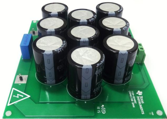
**Figure 23. DC Link Capacitor Bank**
