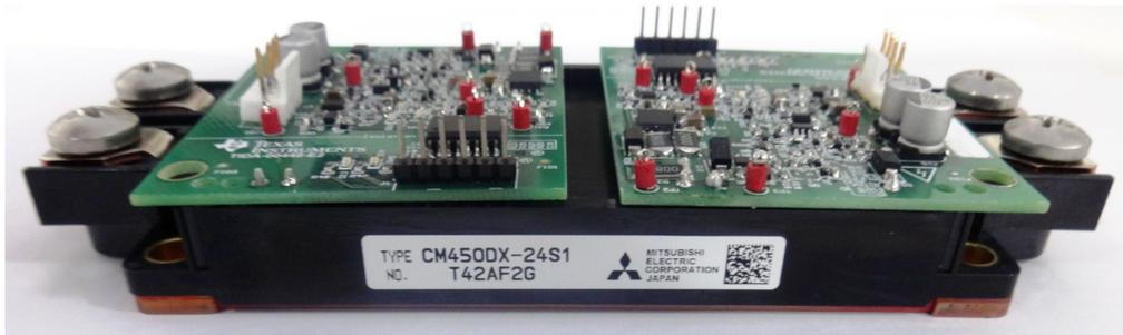
**Figure 22. Isolated IGBT Gate Driver Mounted on IGBT Module**
