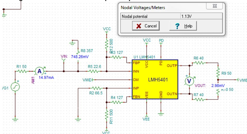
Figure 9 Bias Resistors Pull Up ( $V_s = 5V$  Single Supply)
