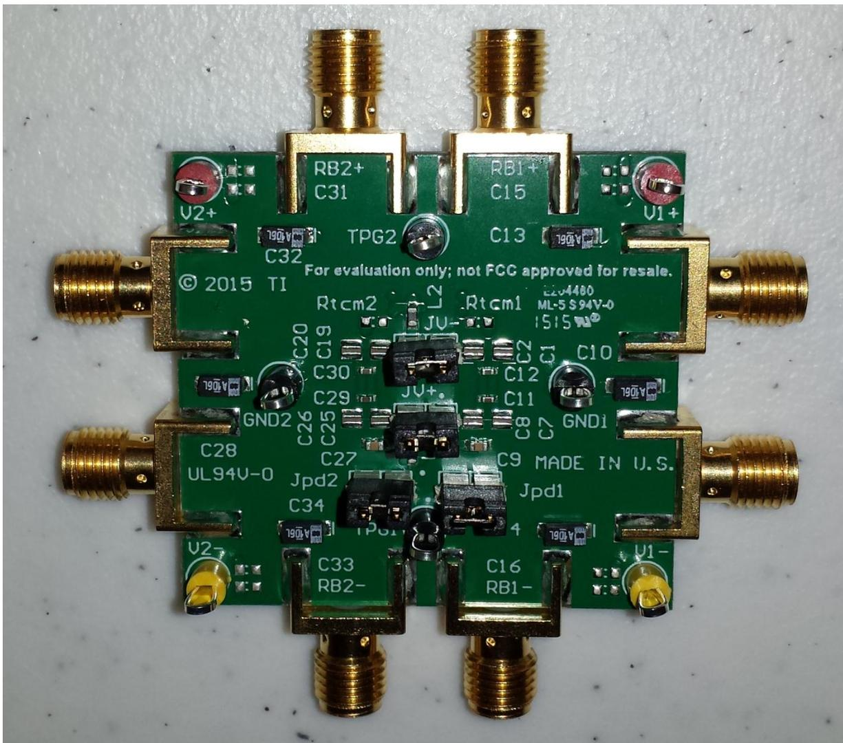
Figure 1: Rear of Board showing power connectors and jumpers
