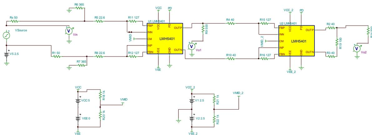
Figure 7 Schematic for Common Mode Shift
