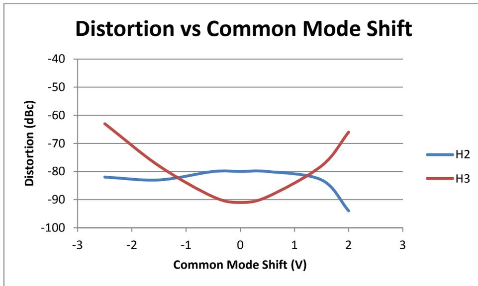
Figure 14 Cascaded Harmonic Distortion,  $V_{out} = 2v_{pp}$ ,  $V_{supply} = 5 V$
