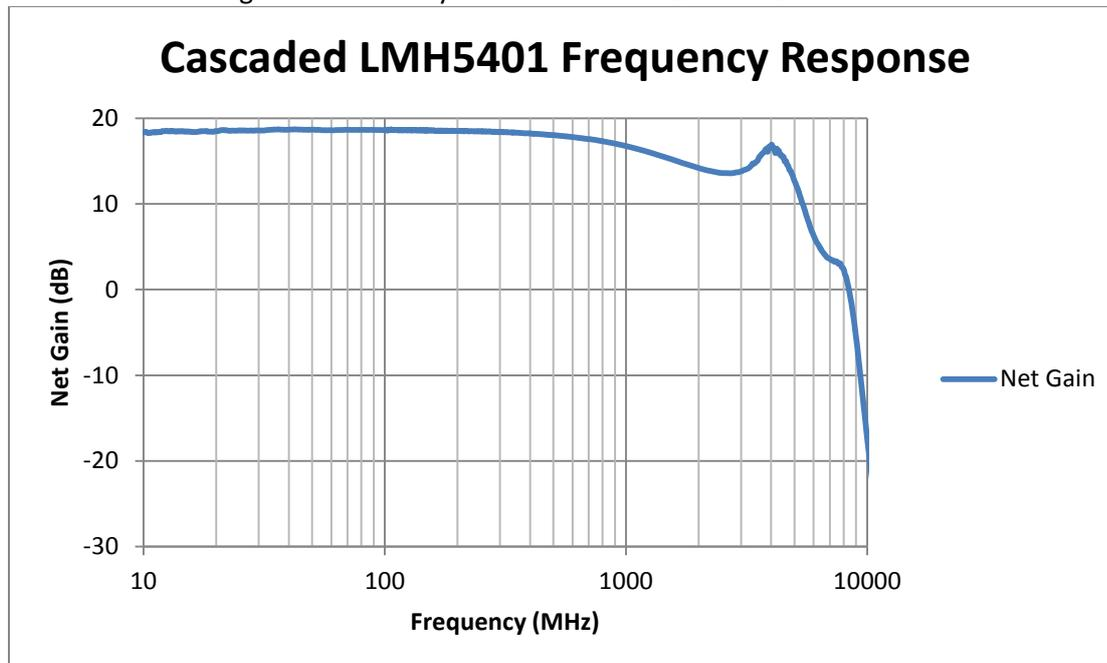
Figure 13 Cascaded Frequency Response (no common mode shift)
