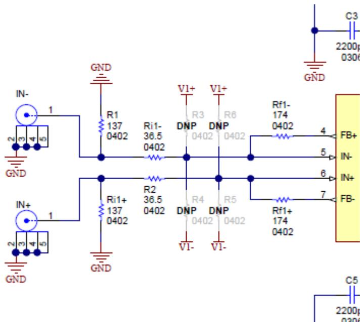
Figure 3 Schematic for Single Ended Input Resistor Value Table
