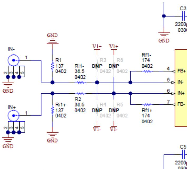
Figure 8 Details of TIDA-00659 Input Components
