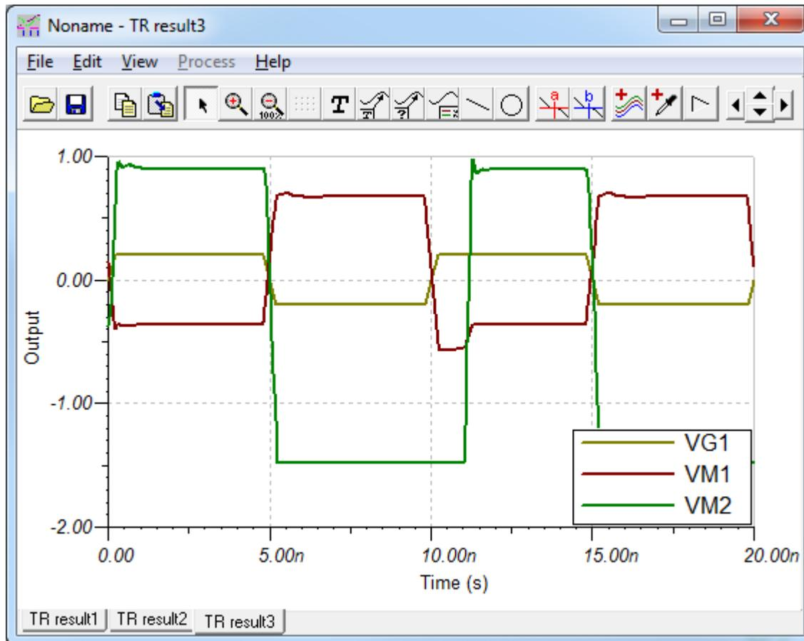
**Figure 19 Transient Response for Cascaded LMH3401, LMH5401**
