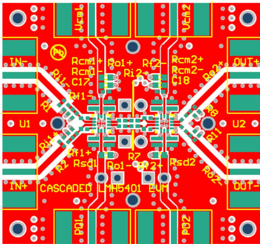
Figure 25: Top Layer, Signal Path
