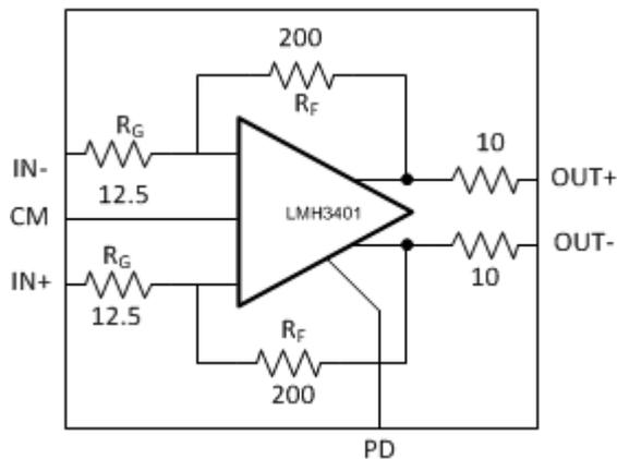
Figure 21 LMH3401 On-Chip Resistors
