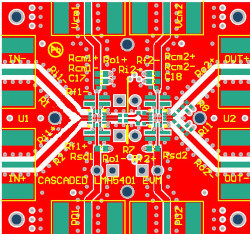
Figure 17 Layout Suggestion for LMH3401 as First Stage
