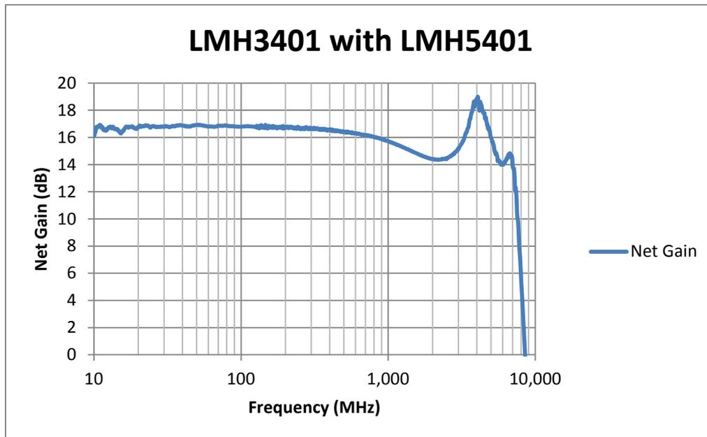
Figure 16 LMH3401 First Stage, LMH5401 Second Stage, Single Ended Input
