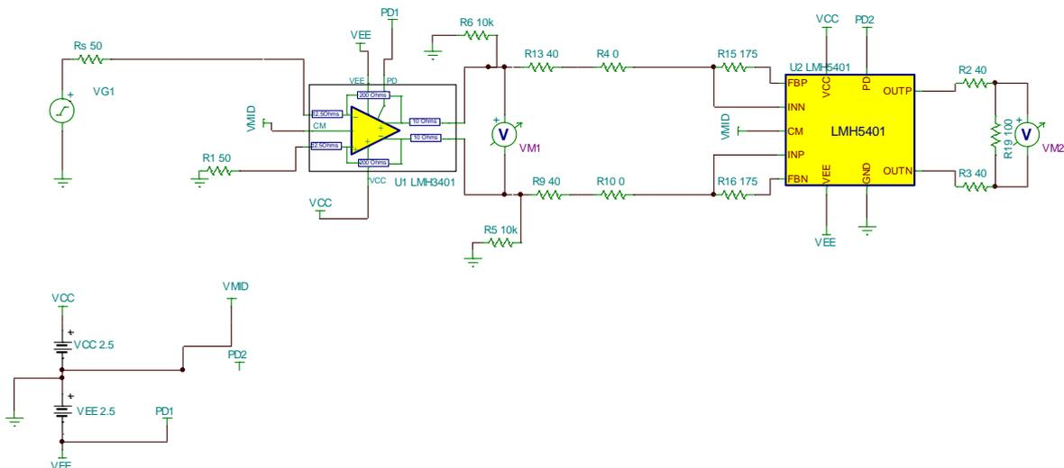
Figure 18 Schematic using LMH3401 and LMH5401.
