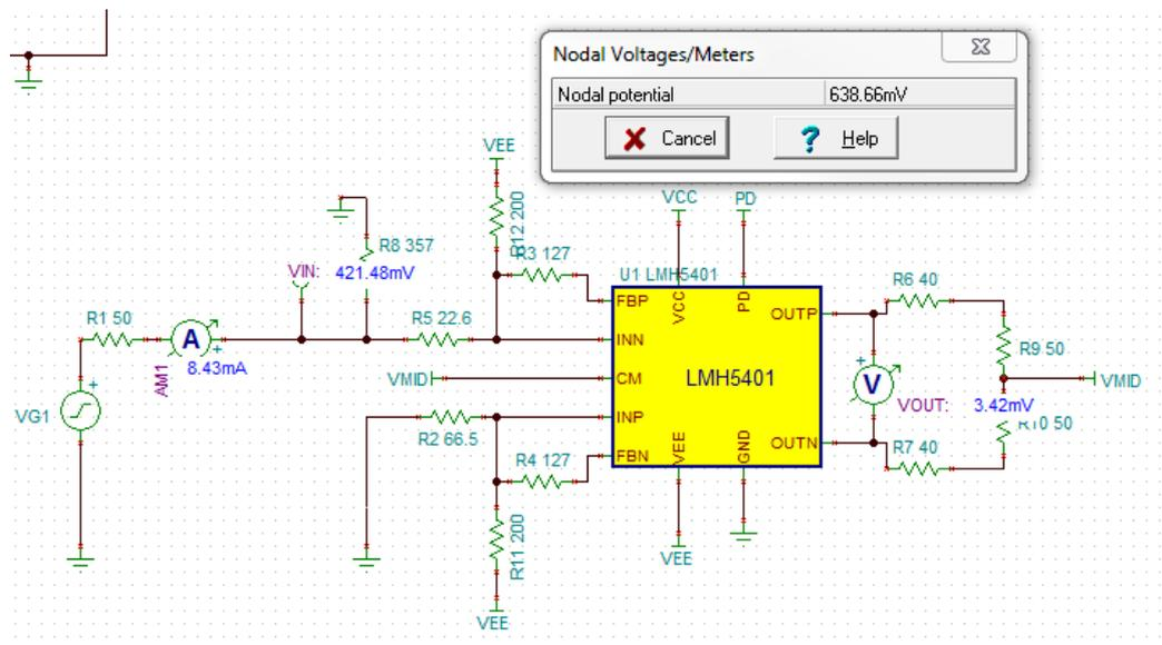
**Figure 10 Bias Resistors Pulling Down**
