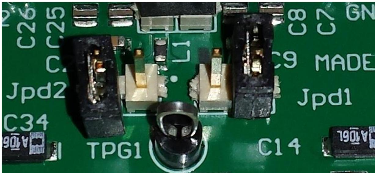
Figure 5 PD Jumpers, Device enabled
