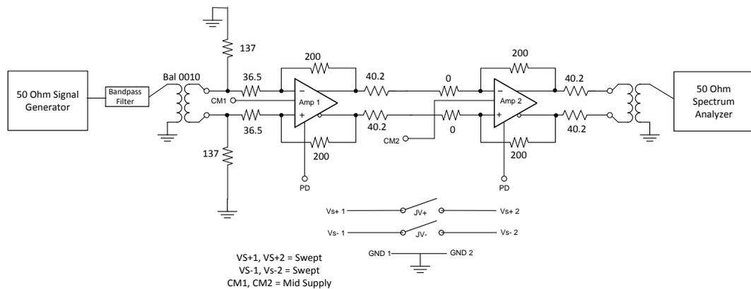
Figure 12 Test Setup Harmonic Distortion
