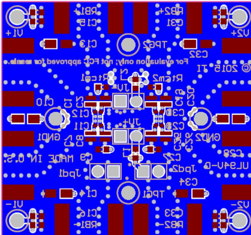
Figure 30: Layer 6, Bypassing capacitors and Power Connectors
