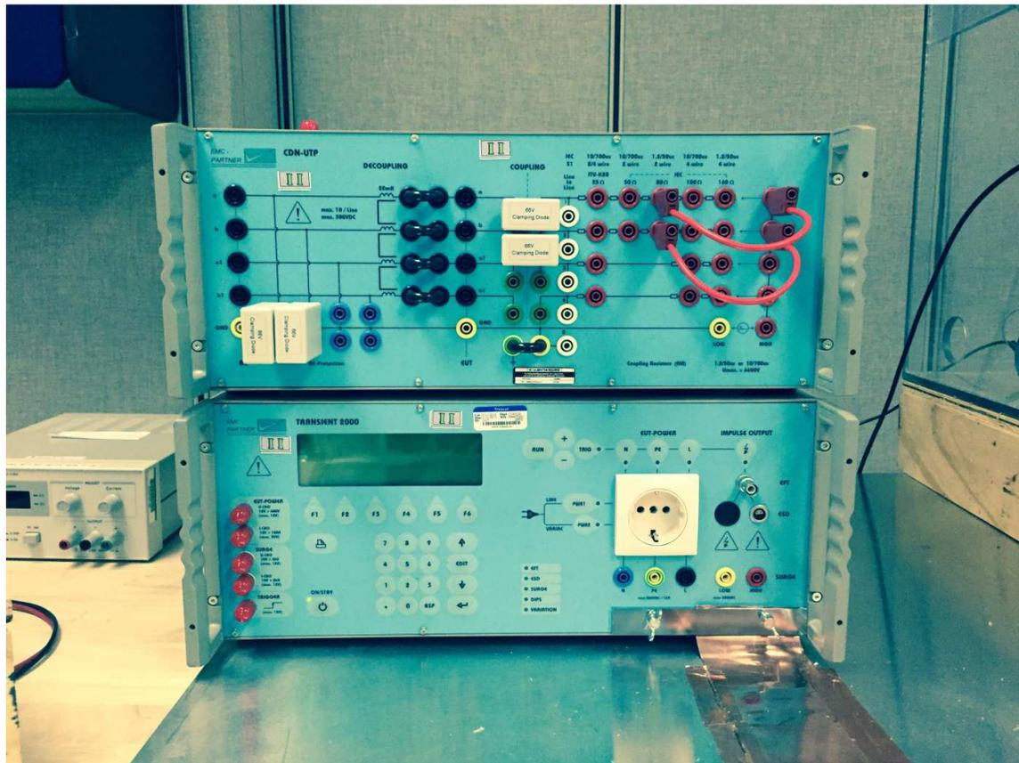
**Figure 7: Electrical Fast Transient (EFT) and Surge Generator**
