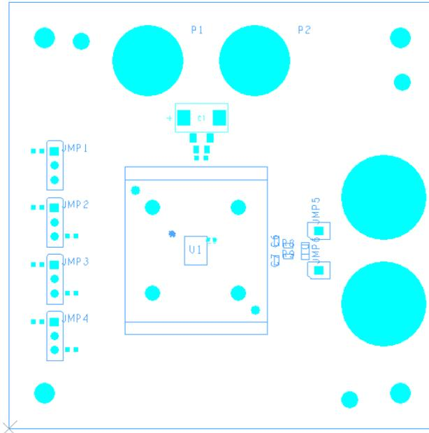
**Figure 16: Bottom Solder Mask**
