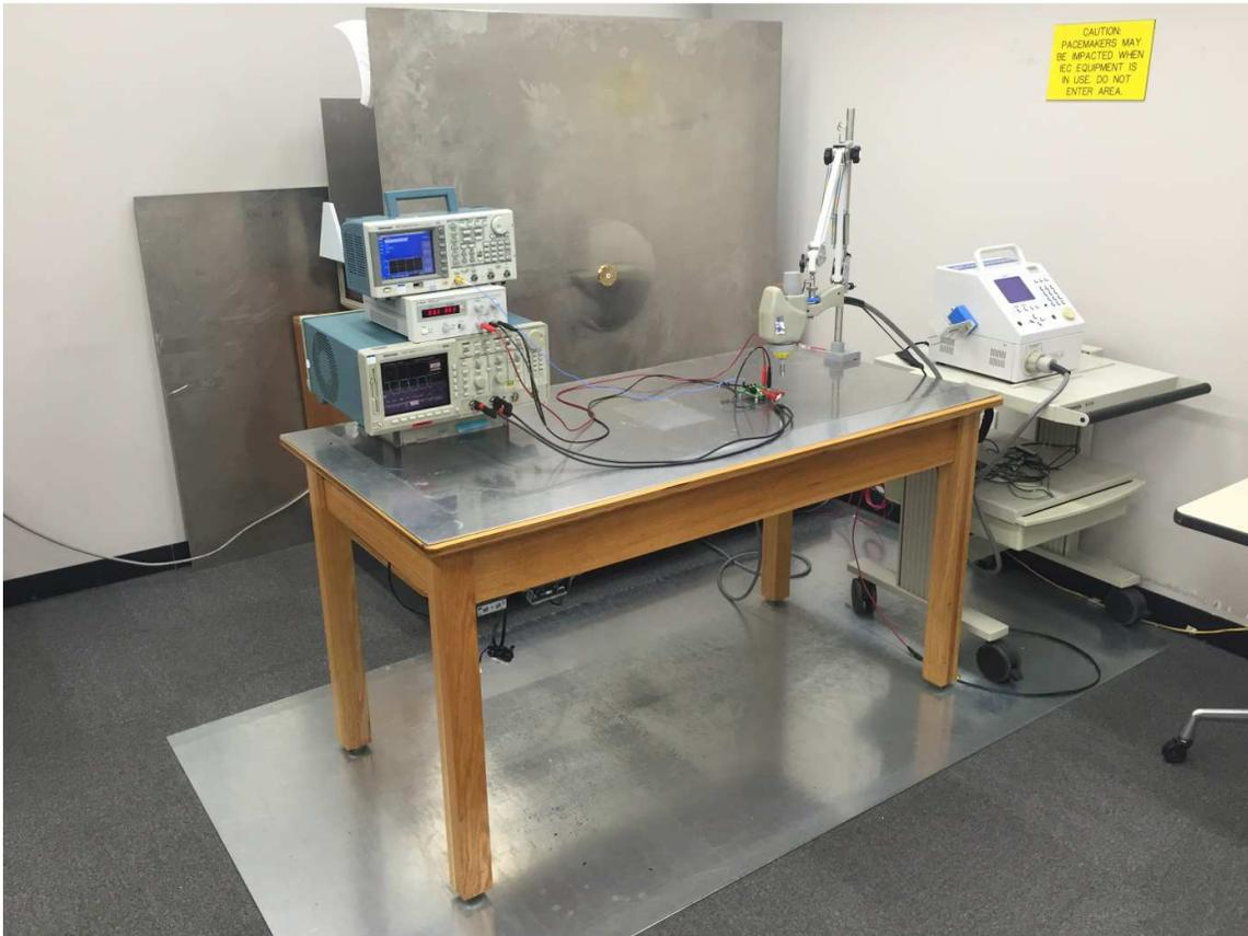
**Figure 6: IEC ESD Compliant Test Setup**
