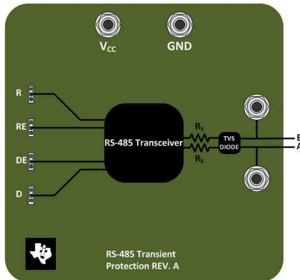
Figure 4: RS-485 Transceiver with TVS Diode and Series Pulse Proof Resistors
