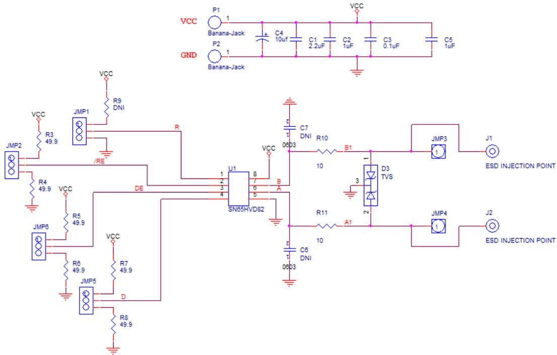
**Figure 10: IEC ESD RS-485 Bus Protection Schematic**
