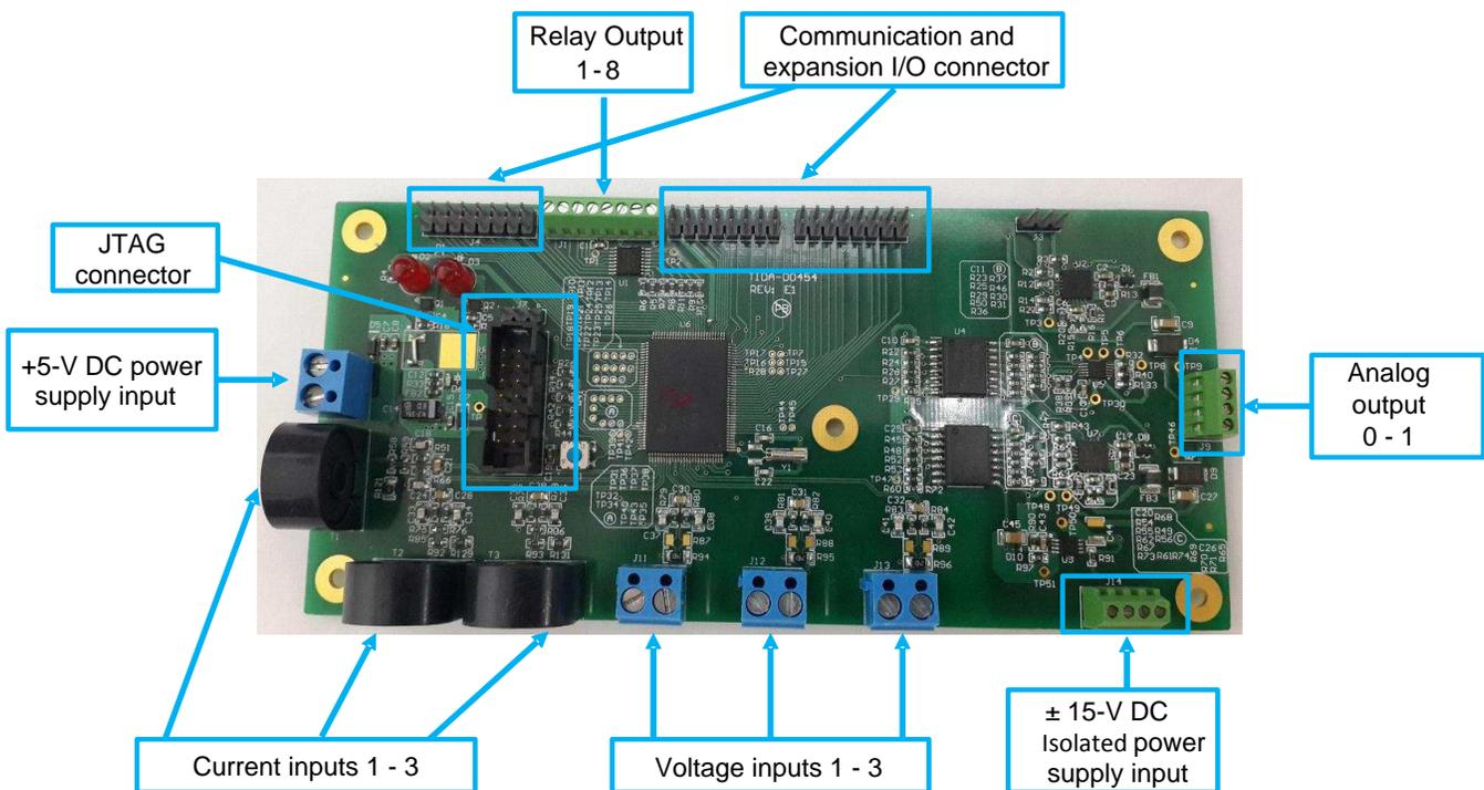
Figure 23. TIDA-00454 Interface Connectors
