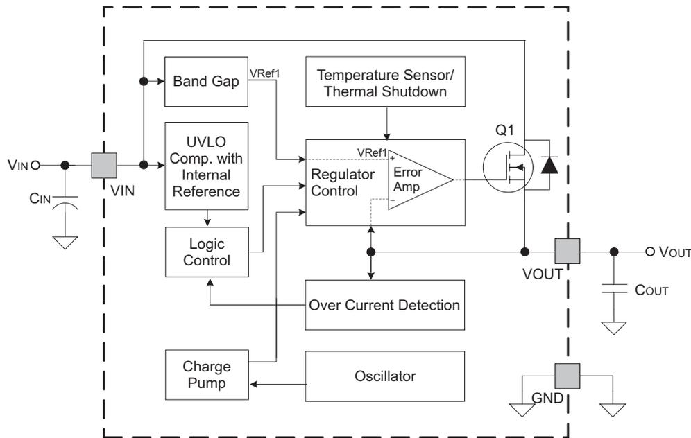
**Figure 8. TPS7A65-Q1 Functional Block Diagram**
