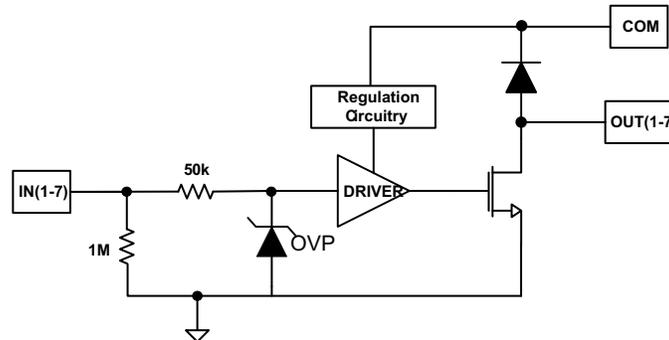
Figure 6. TPL7407L Functional Block Diagram
