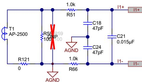
Figure 9. Circuit Diagram of Current Input
