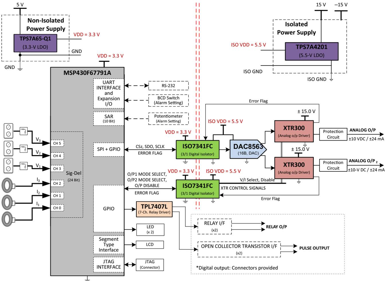
Figure 1. TIDA-00454 Functional Block Diagram
