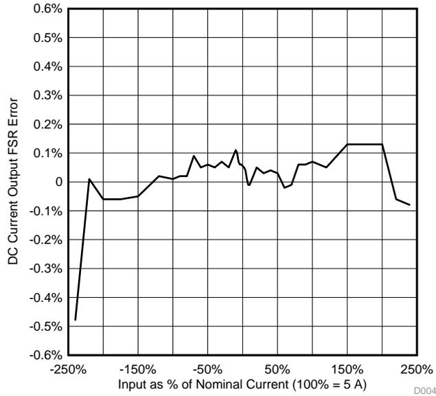
**Figure 35. DC Current Output Accuracy Test for AOUT1**
