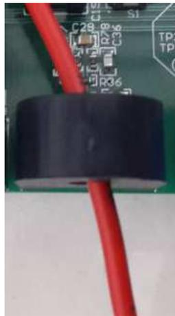
Figure 22. Current Input Wire Through CT
