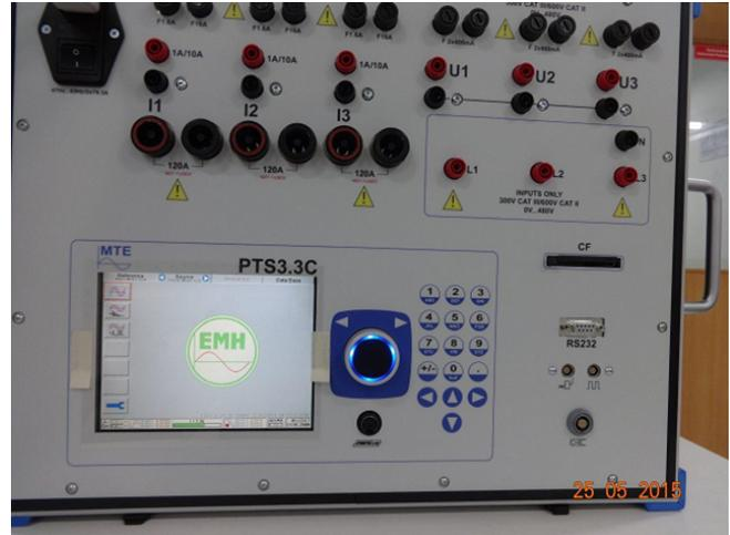
Figure 30. Programmable Power Source
