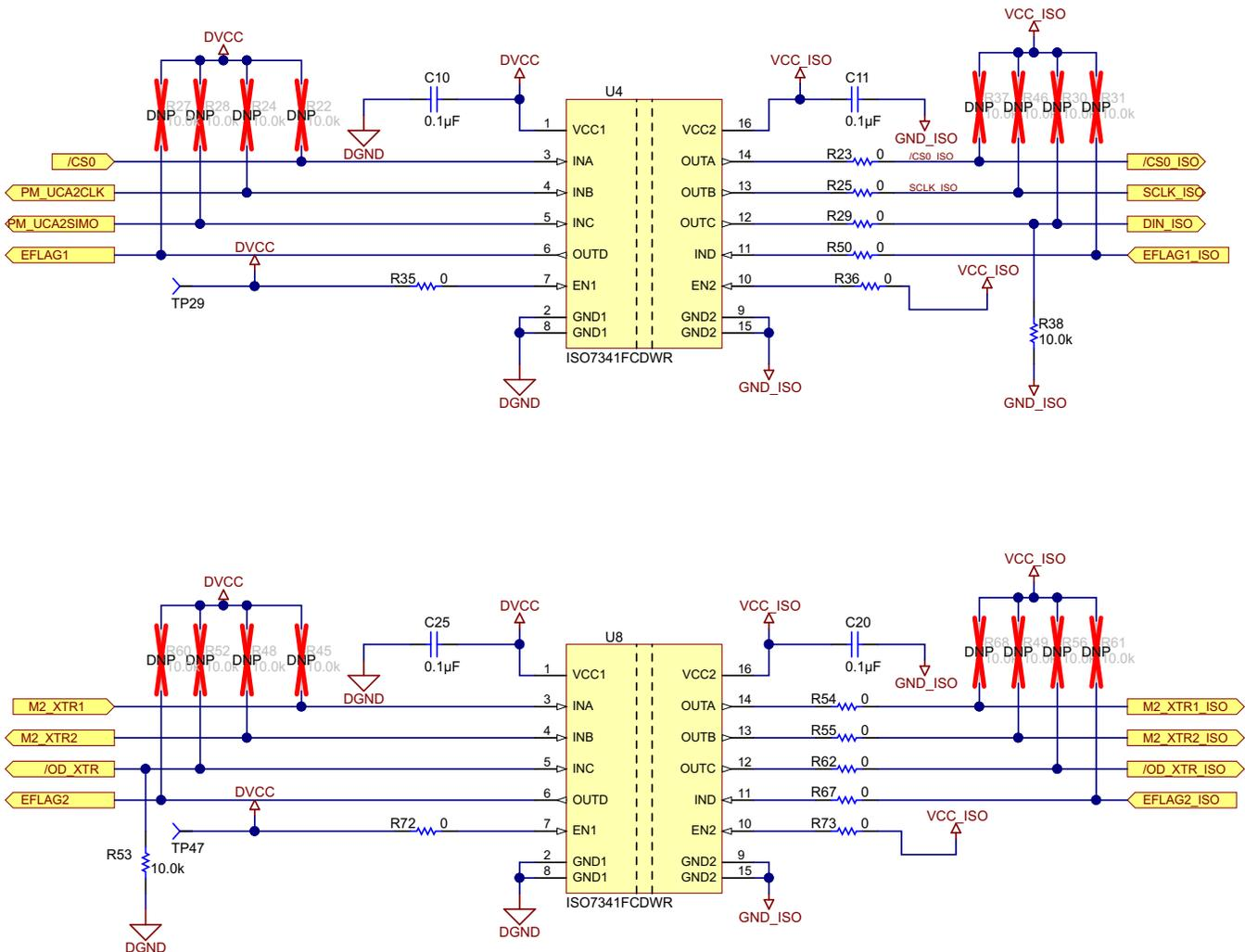
**Figure 13. Circuit Diagram of Digital Isolators Interface**
