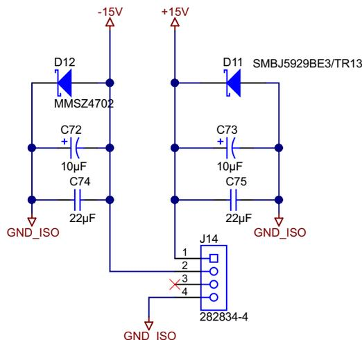
Figure 19. Input Connection for 15 V and –15 V
