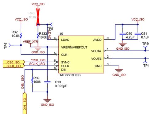
Figure 11. DAC8563 Circuit Diagram
