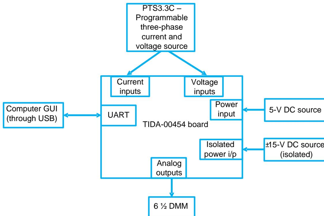
Figure 31. Test Setup for Connecting TIDA-00454 Board
