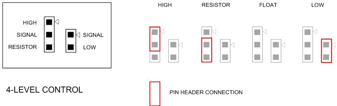
**Table 1: Jumpers to set the 4-Level input control pins**
