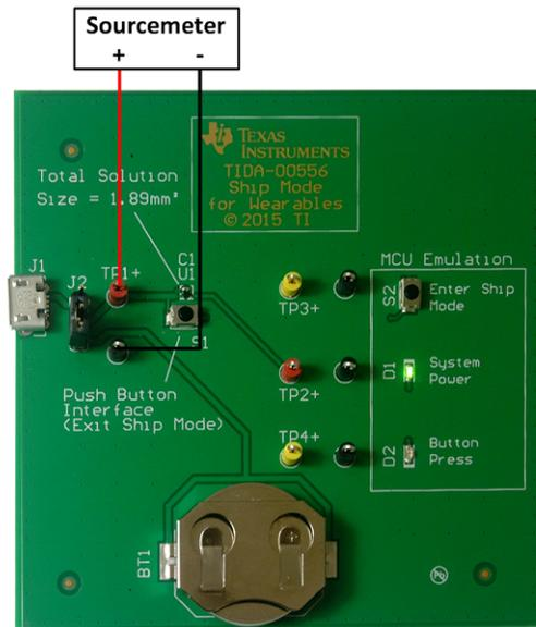
**Figure 13. Configuration for Quiescent Current Measurements**
