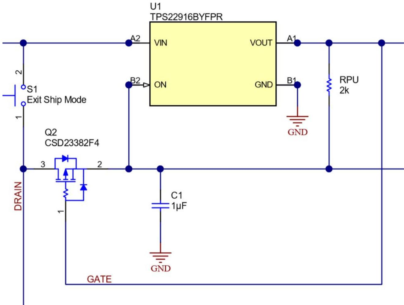
Figure 4. Exit Ship Mode Schematic
