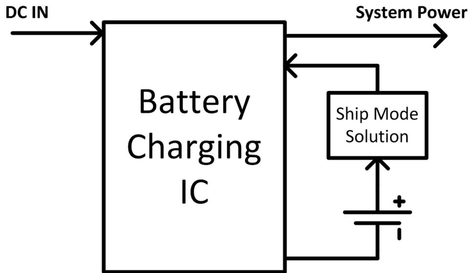
Figure 7. Ship Mode Implementation With a Rechargeable Battery IC
