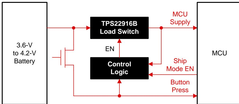
**Figure 2. Block Diagram of the TPS22916B**
