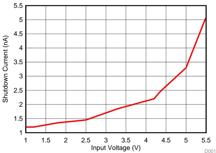
**Figure 14. Shutdown Current Across Input Voltage**
