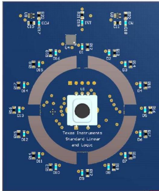
Figure 7. Prototype Hardware With Rotary Quadrature Decoder and Output Circuitry
