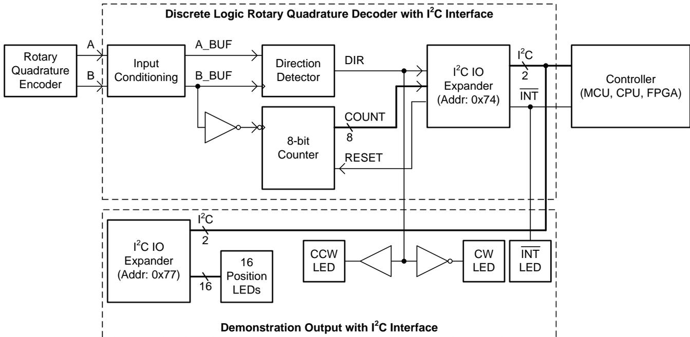
Figure 1. Rotary Quadrature Decoder TIDA-00580 Block Diagram
