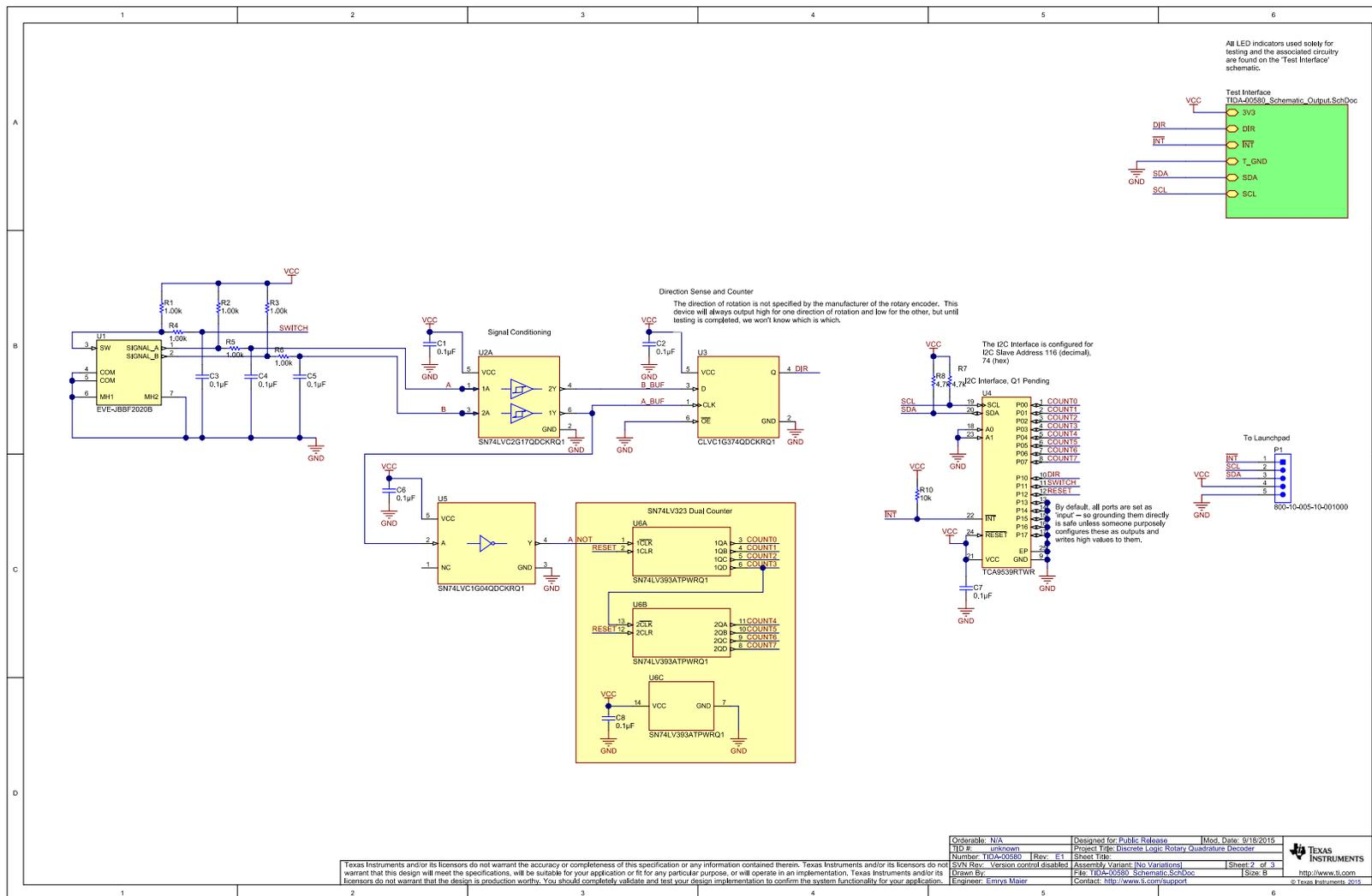
Figure 13. Schematics Page 1—Rotary Quadrature Decoder Circuitry
