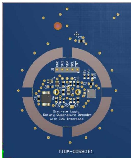
Figure 8. Rotary Quadrature Decoder Bottom View
