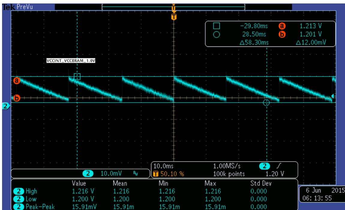
Figure 12 – DCDC2 Voltage Ripple, Light Load @ 25C
