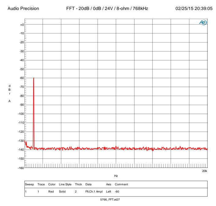
Figure 1. Optical Input to Class-D Output Noise Floor FFT
