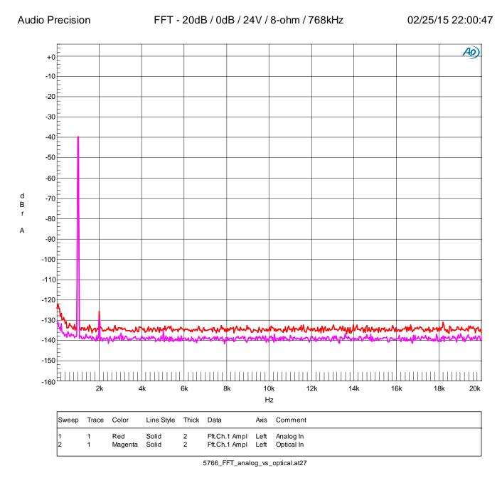
Figure 2. Optical Input / Analog Input Comparison
