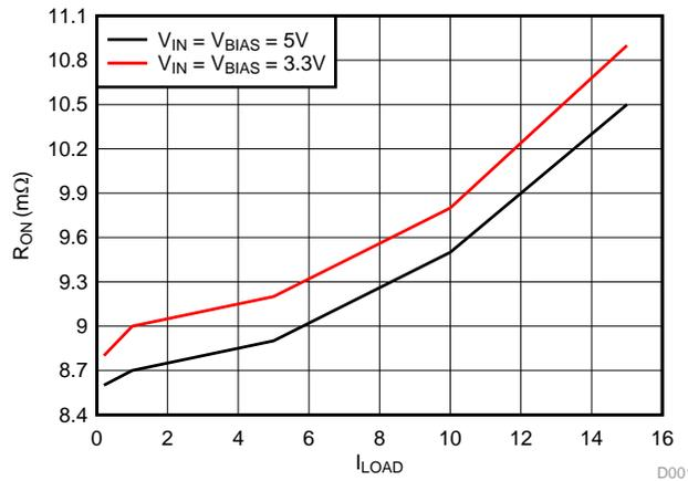
Figure 15. Back-to-Back Circuit ON Resistance versus Load Current
