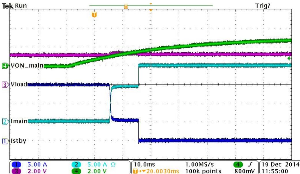
Figure 13. Switching from Standby to Main (3.3 V)
