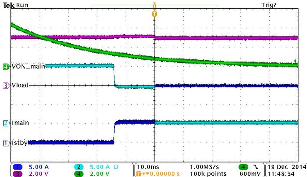
Figure 10. Switching from Main to Standby (5 V)
