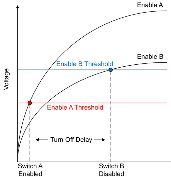
**Figure 5. RC Timing Circuit Charging**
