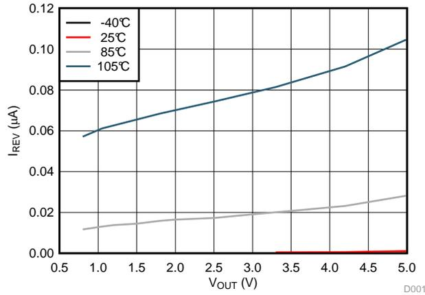
Figure 14. Back-to-Back Circuit Reverse Leakage Current
