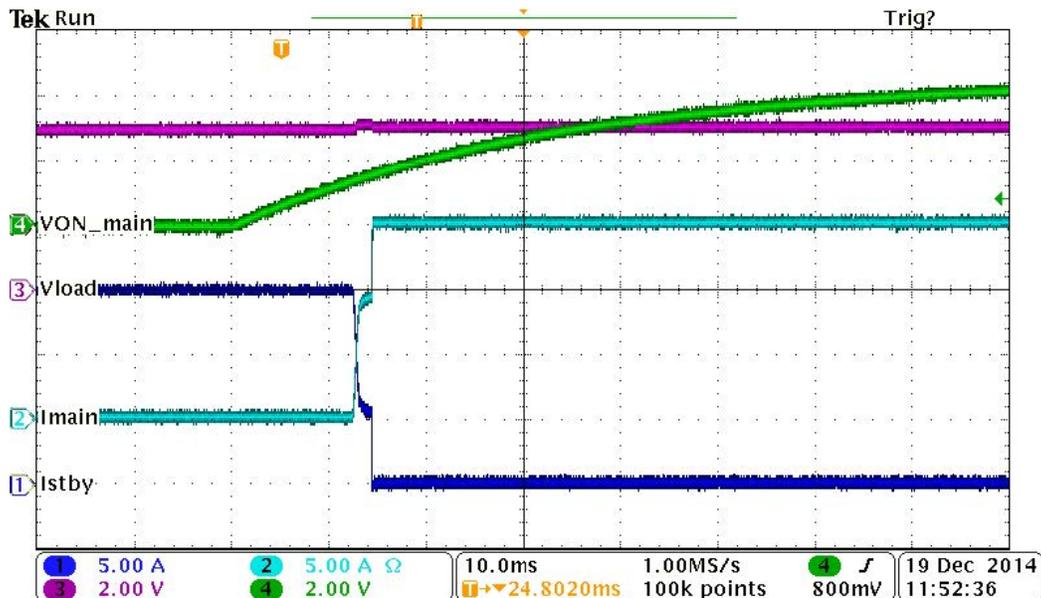
Figure 11. Switching from Standby to Main (5 V)
