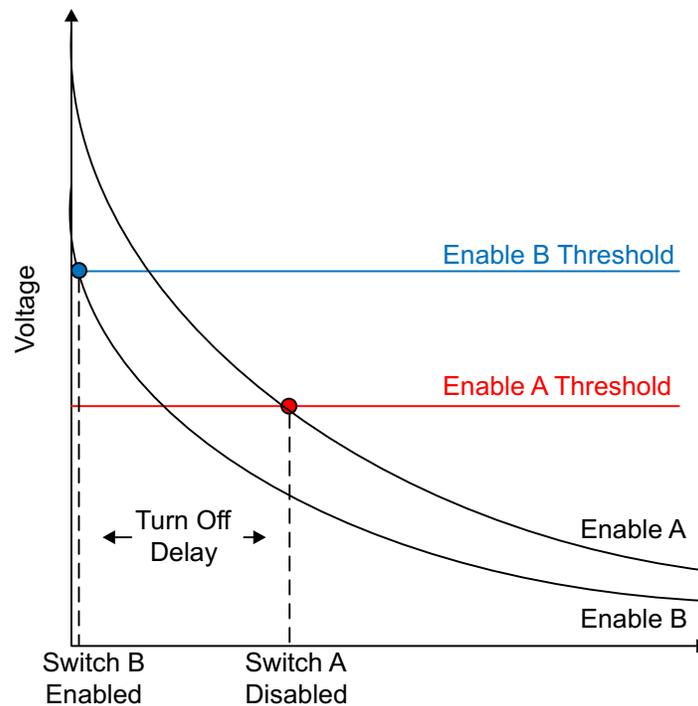
**Figure 6. RC Timing Circuit Discharging**
