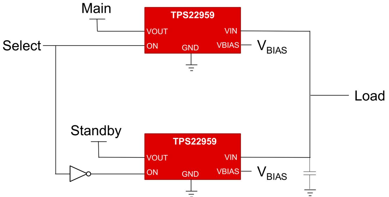
Figure 1. Make-Before-Break 2:1 Power MUX Block Diagram
