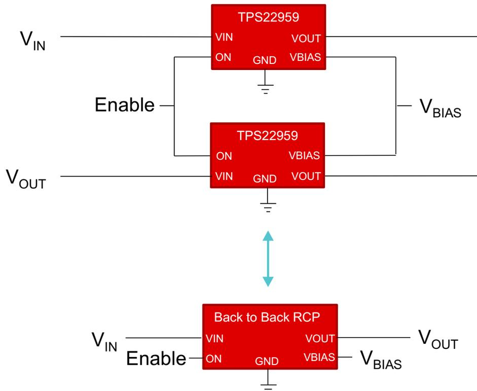
**Figure 2. Back-to-Back Configuration for Bi-Directional Current Blocking**
