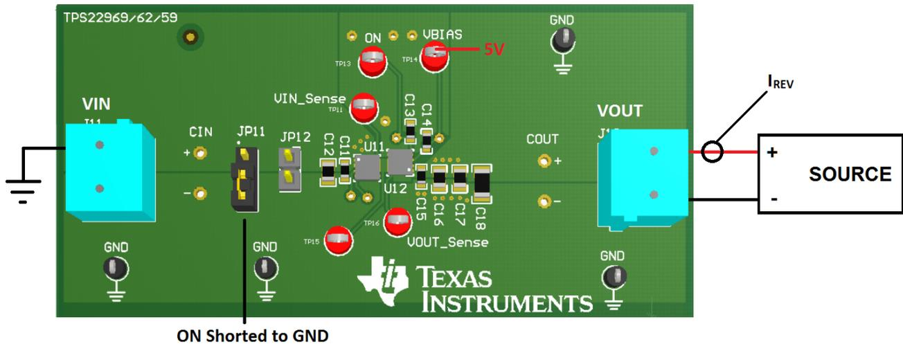
Figure 8. Back-to-Back Reverse Current Blocking Test Setup
