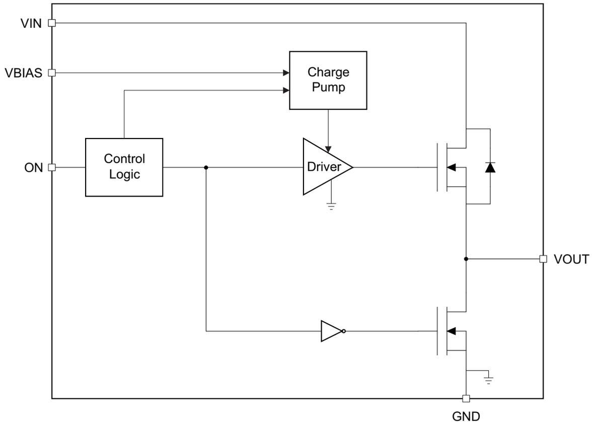
Figure 3. TPS22959 Functional Block Diagram
