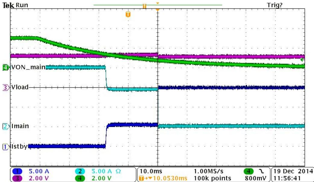
Figure 12. Switching from Main to Standby (3.3 V)
