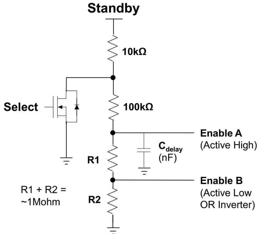
Figure 4. Make-Before-Break RC Timing Circuit
