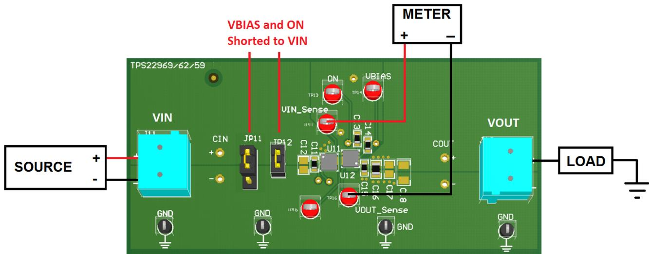
Figure 9. Back-to-Back Circuit ON Resistance Test Setup
