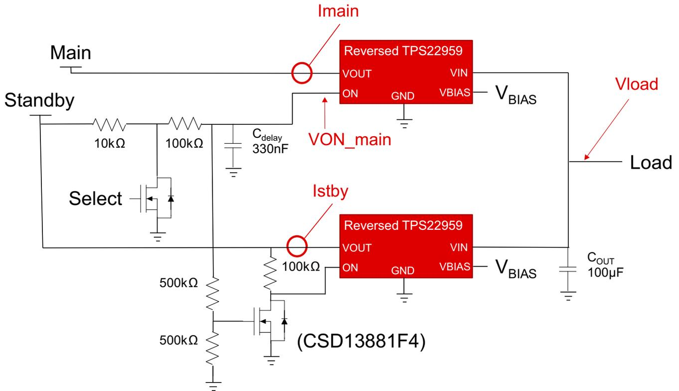
Figure 7. Power MUX Waveform Setup
