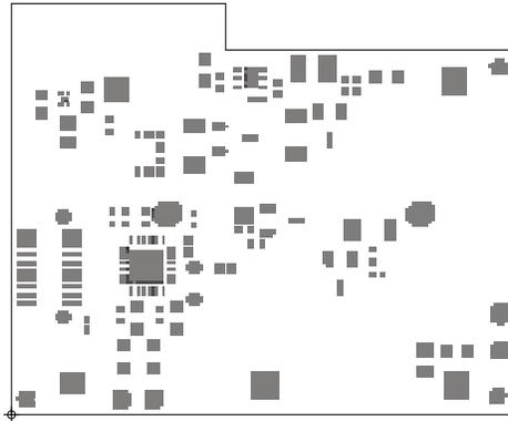
**Figure 13. Bottom Solder Mask**
