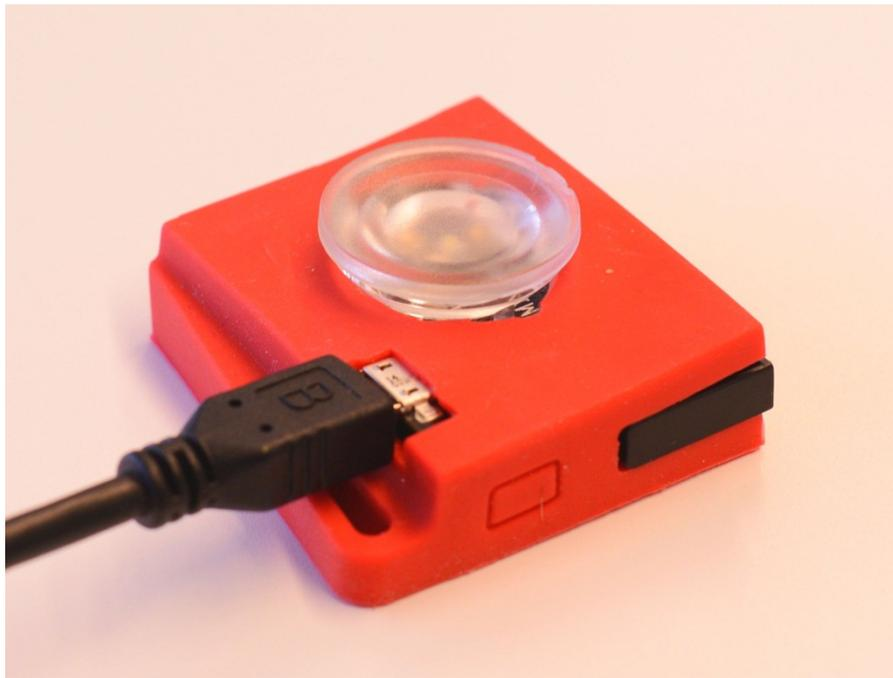
**Figure 7. LED Audio DevPack with Lens and USB Power**
