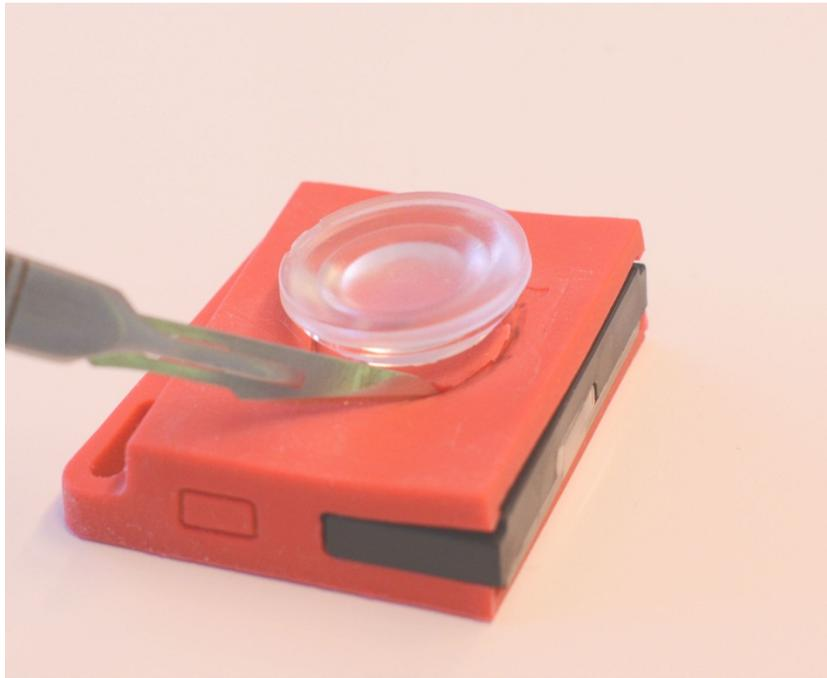
**Figure 6. Cutting the Sleeve to Fit a Lens**
