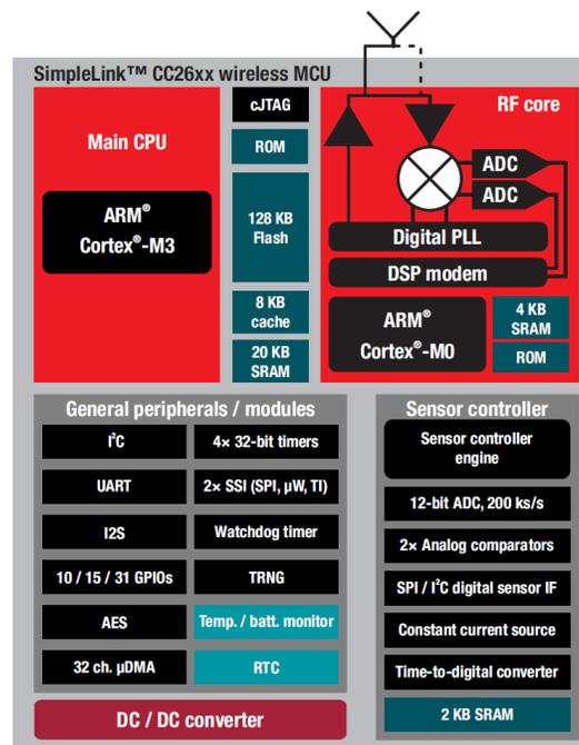
Figure 1. CC2650 Functional Block Diagram
