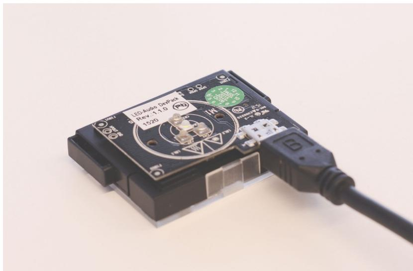
Figure 4. LED Audio DevPack with USB Power
