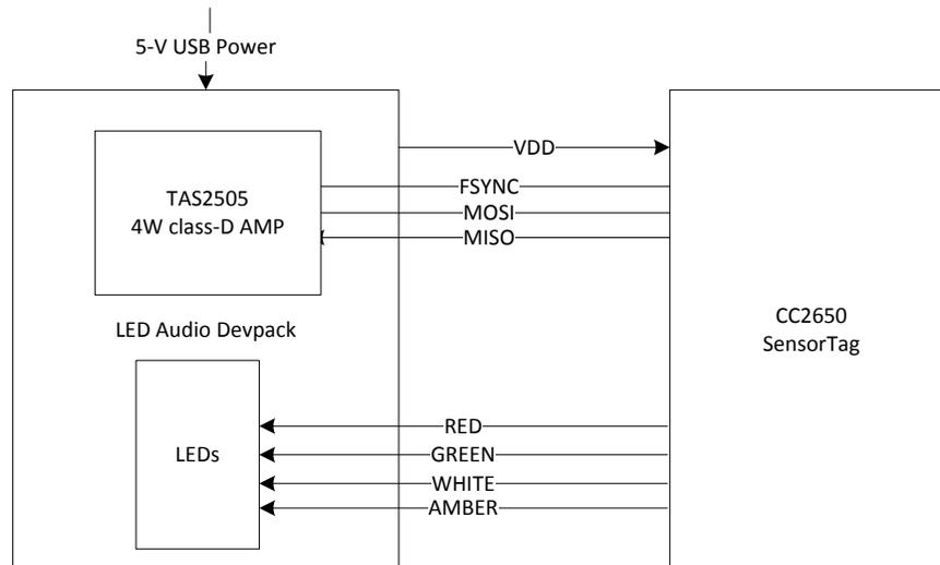
Figure 2. Block Diagram
