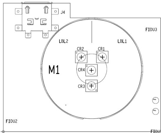
Figure 16. LED Audio DevPack Assembly Top
