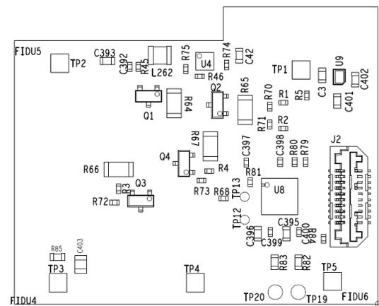
Figure 17. LED Audio DevPack Assembly Top
