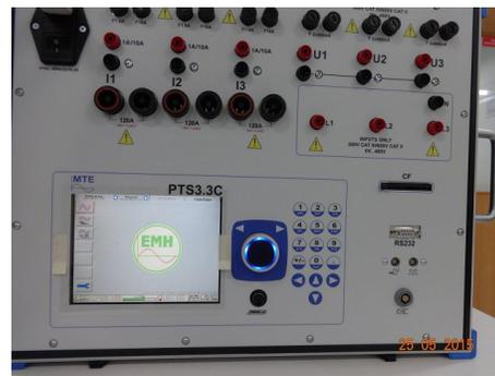
Figure 20. Programmable Power Source
