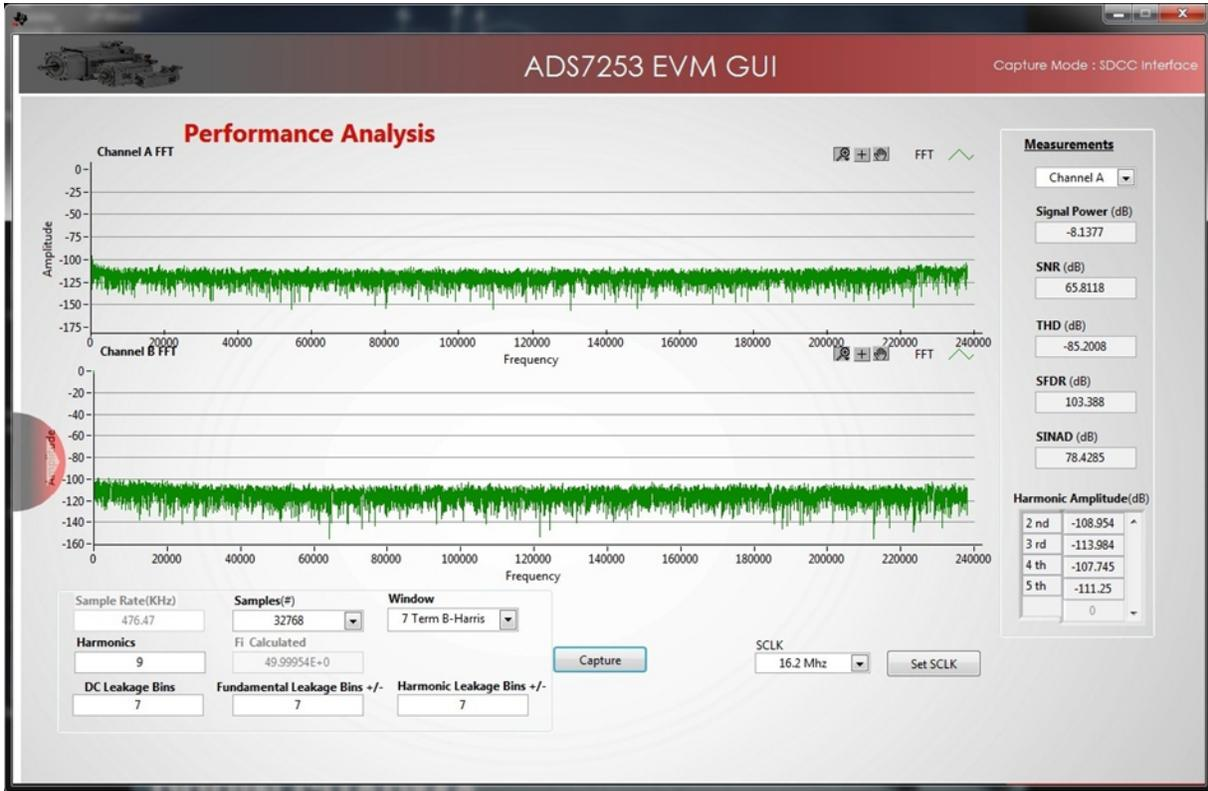
Figure 67. FFT Captured With ADS7253EVM GUI
