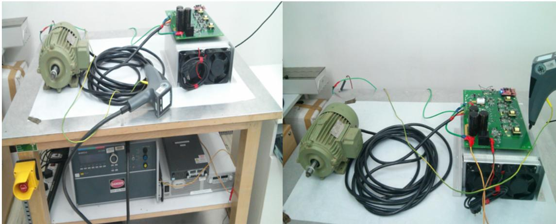
**Figure 113. EUT/AUX Equipment on Insulated Sheet**
