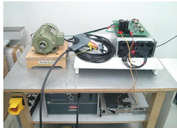
**Figure 115. EUT/AUX Equipment Isolated From Reference Plane by 10 cm**
