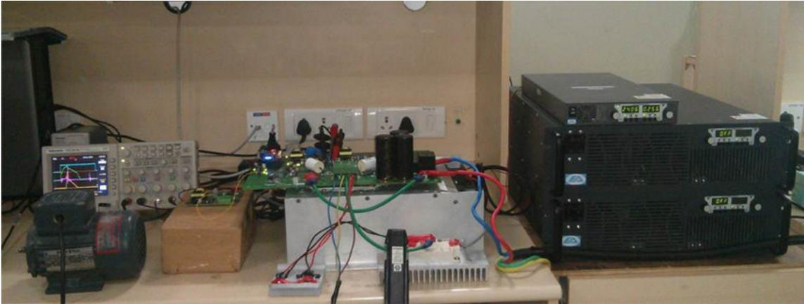
**Figure 101. Setup for Short Circuit Test — Fault Under Load**
