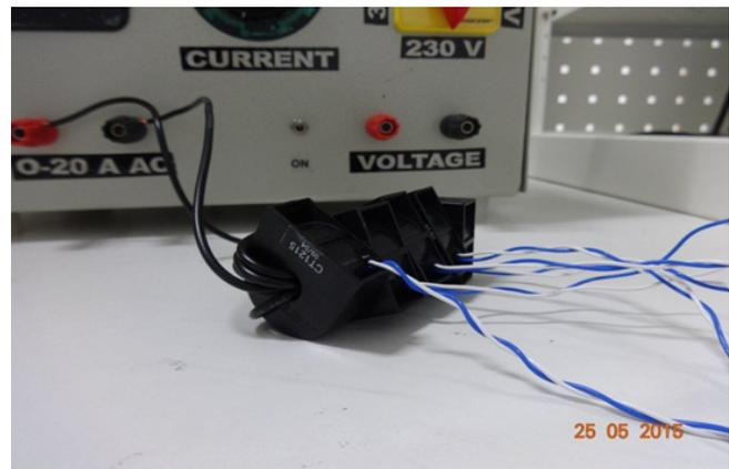
Figure 25. Current Transformer
