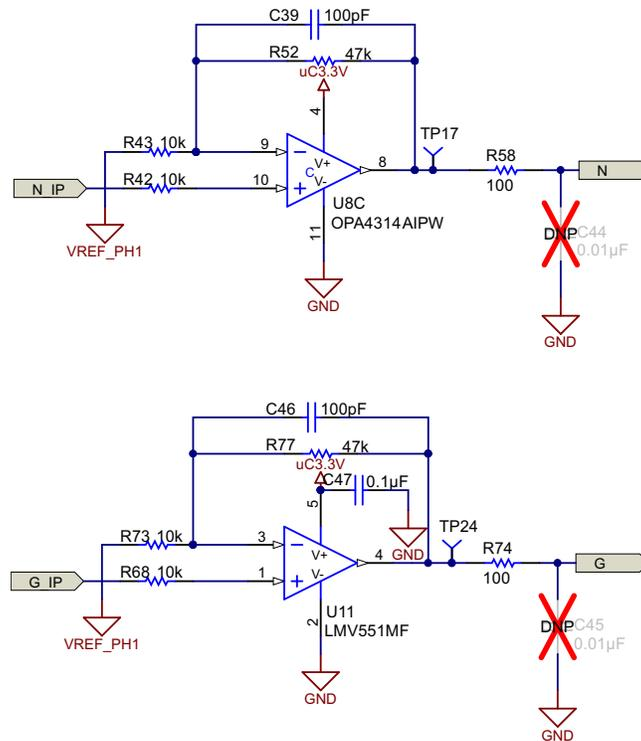
Figure 17. Amplifier With Single Gain Schematic
