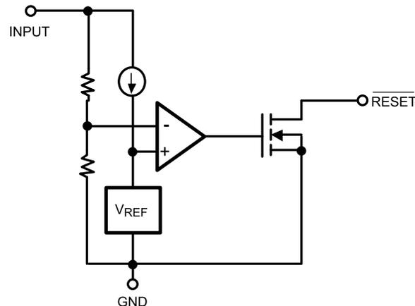
Figure 7. LM8364 Functional Block Diagram
