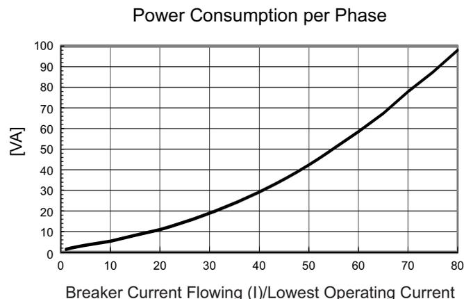
**Figure 1. Typical Power Consumption for Current and Lowest Operating Current**
