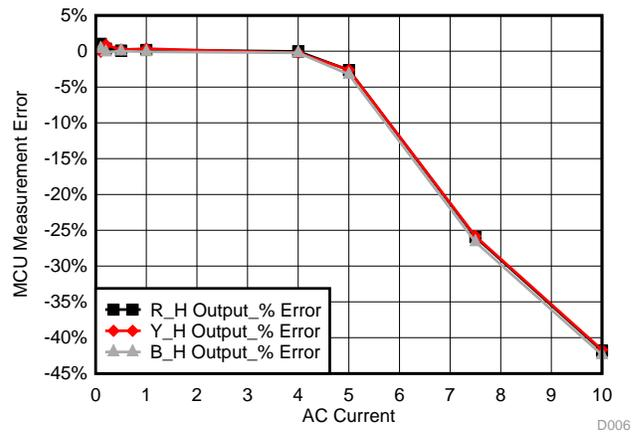
**Figure 35. High Gain Measurement Error With Internal 12-Bit ADC**
