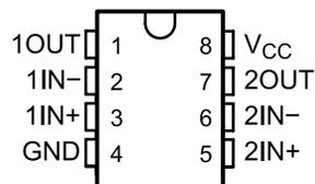
**Figure 9. LM2903 Pinout Diagram**
