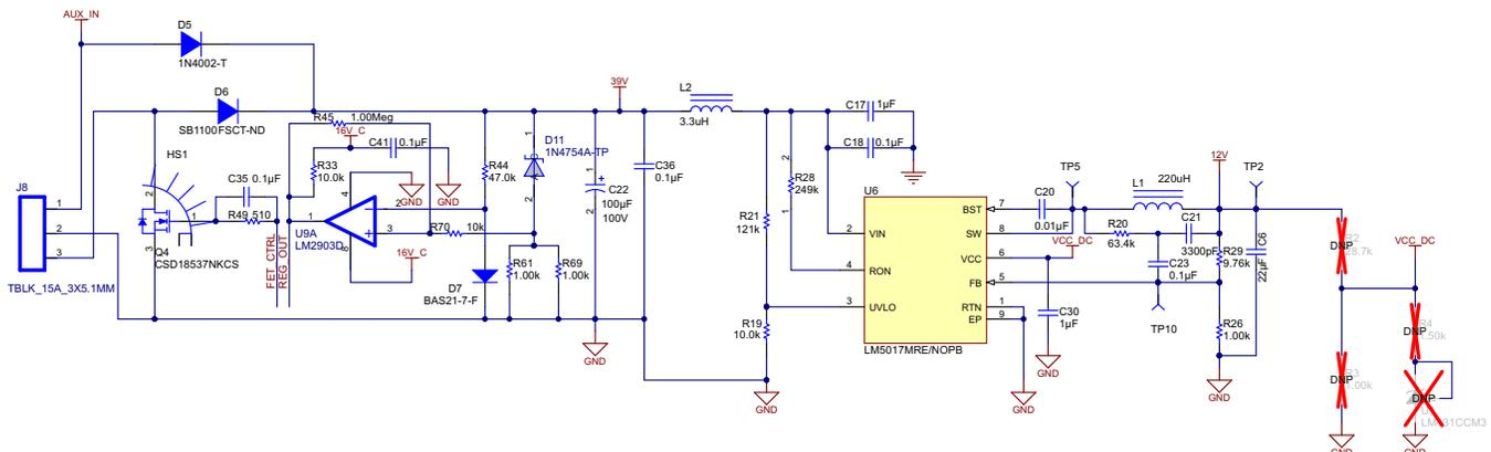
Figure 10. Self-Power Supply Including DC-DC Converter Schematic
