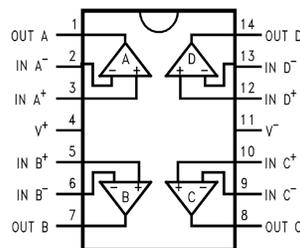
**Figure 5. LMV614 Pinout Diagram**
