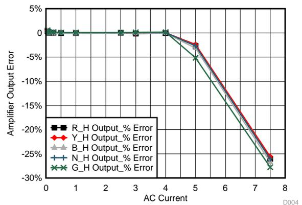
**Figure 33. Current Versus Output Error for High Gain Amplifier Using OPA4314**
