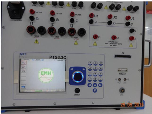
Figure 24. Programmable Current Source
