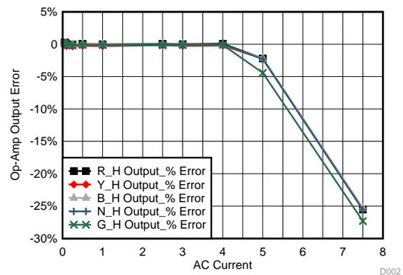
**Figure 31. Current Versus Output Error for High Gain Amplifier Using LMV614**
