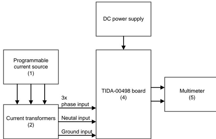
Figure 23. Test Setup Block Diagram
