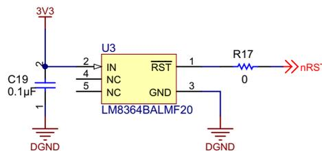
Figure 22. Undervoltage Sense Input to MCU Schematic
