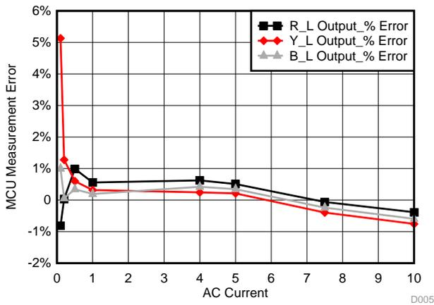
**Figure 34. Low Gain Measurement Error With Internal 12-Bit ADC**
