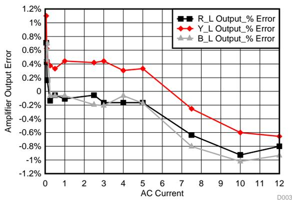
**Figure 32. Current Versus Output Error for Low Gain Amplifier Using OPA4314**
