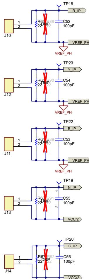
Figure 15. Current Input Connector With Burden Resistor
