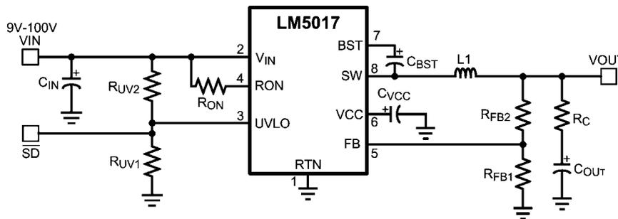
**Figure 8. LM5017 Typical Application Diagram**
