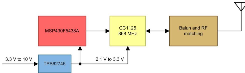
**Figure 4. TIDC-DSSS868WMBUS-DC Block Diagram**
