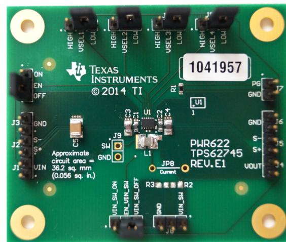
Figure 6. TPS62745 EVM With Jumpers to Set  $V_{OUT}$  Voltage
