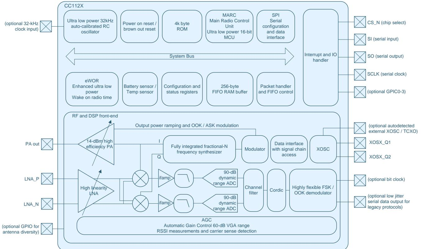
Figure 2. CC1125 Functional Block Diagram
