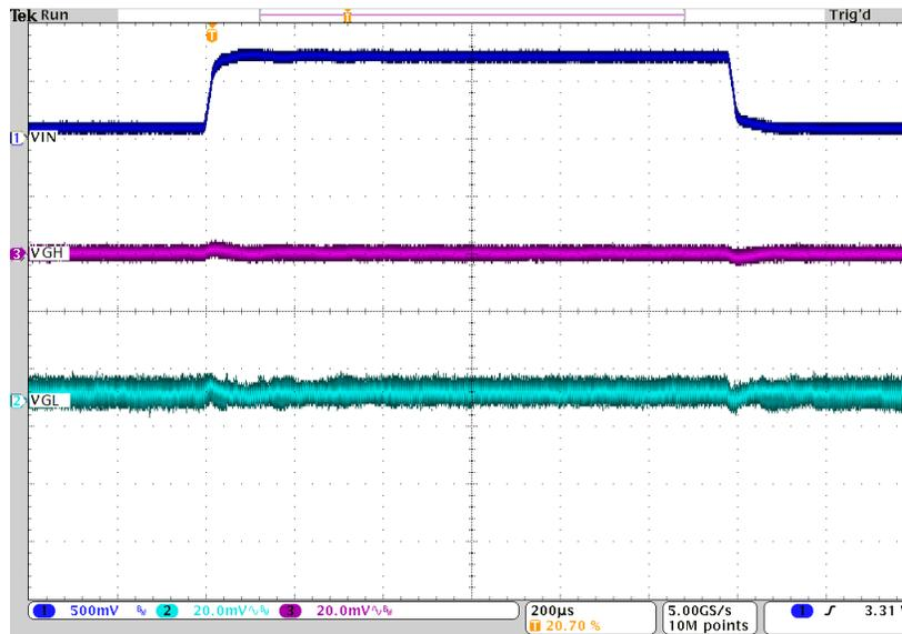
Figure 11.  $V_{GH}$  and  $V_{GL}$  Line Transient Response
