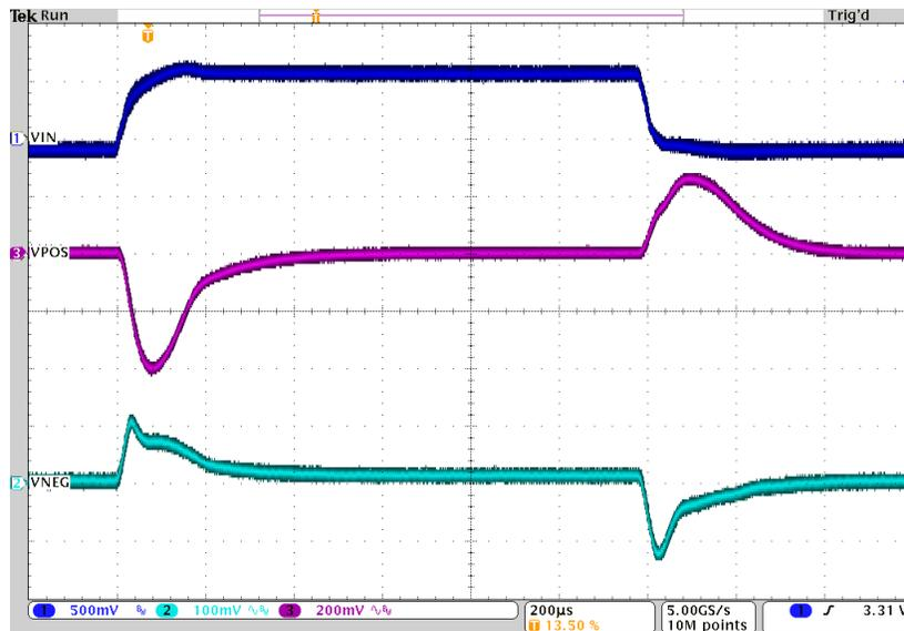
Figure 10.  $V_{POS}$  and  $V_{NEG}$  Line Transient Response
