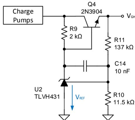
Figure 3.  $V_{GH}$  Regulator
