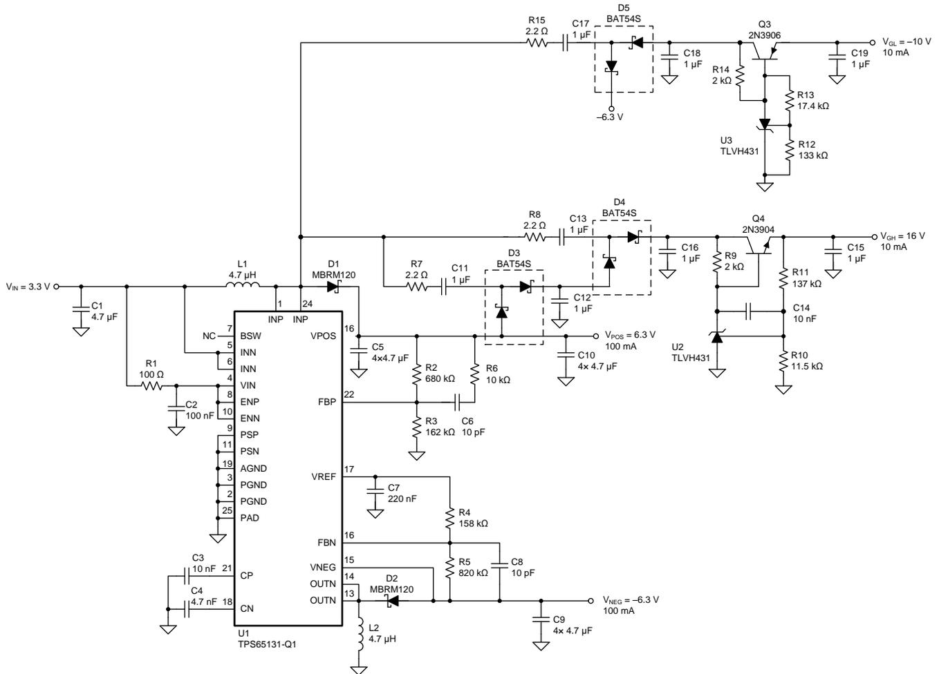
**Figure 1. TPS65131-Q1 Circuit Schematic and Charge Pump**
