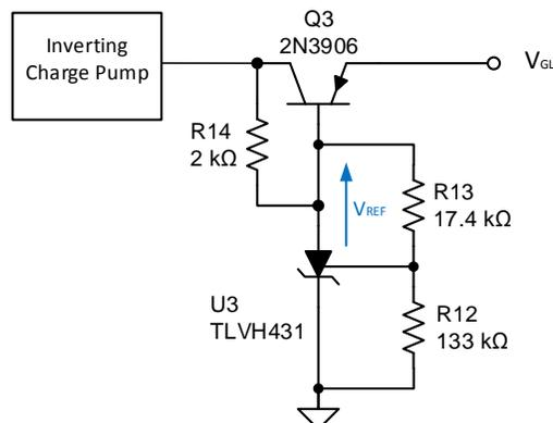
Figure 4.  $V_{GL}$  Regulator
